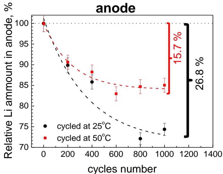
By the fatigue introduced the system loses free (transport) lithium;
