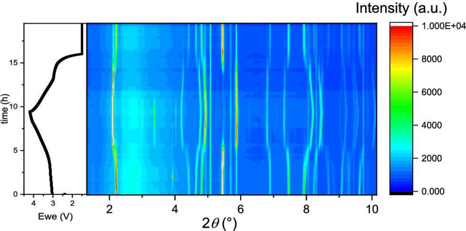
Courtesy: D. Mikhailova; Evolution of  $\text{NaNi}_{0.5}\text{Ti}_{0.5}\text{O}_2$  structure, NNTO+NiO+Na+Al present to pattern
