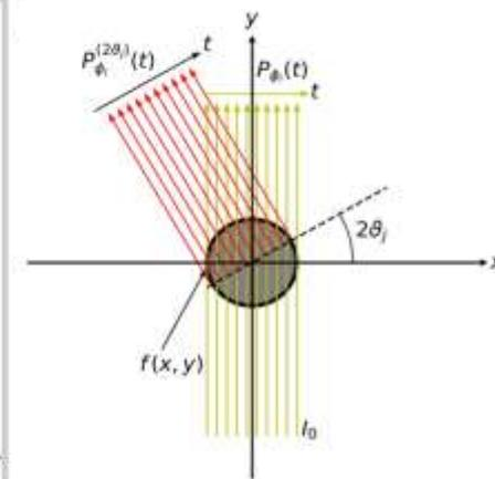
The XRD tomography experiment was performed on P07 beamline at PETRA III using  $0.5 \times 0.5 \text{ mm}^2$  sized beam of ca. 60 keV energy, 0.2 mm rastering step (111 translation points) and 61 projections collected upon  $6^\circ$  rotation. Altogether 6771 diffraction patterns were collected.
