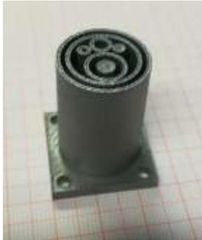
“Phantom” sample – object with the contrast sufficient for the method validation. The 3D printed aluminum cylinder (20 mm in diameter) with the following layout was filled with different powders:
