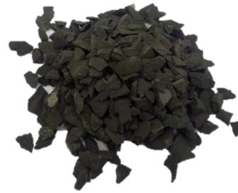
**Figure 83. A disintegrated core sample of Bazhenov oil shale (Bondarenko et al., 2016).**
