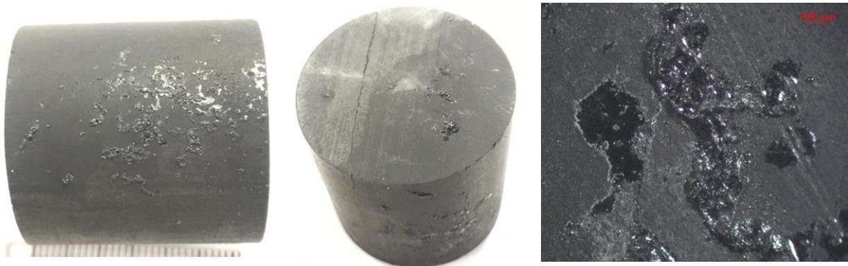
**Figure 87. Photo of the core sample after exposure (Oil Field 4).**
