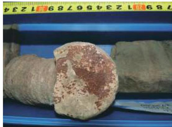
**Figure 13.** Photo of the core from the Well #219bis drilled 70m away from the injection well, giving evidence of oxidation reactions occurrence (*Darischev et al., 2017*).
