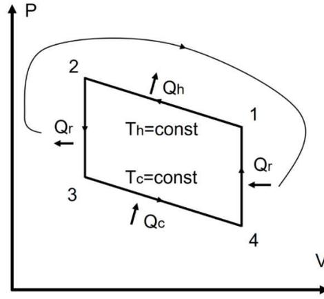
Fig. 2. Ideal Stirling refrigerator cycle.
