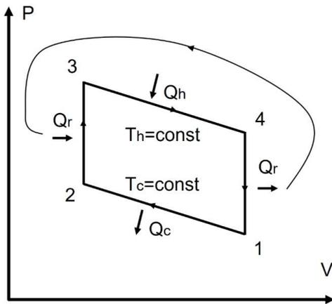
Fig. 1. Ideal Stirling engine cycle.
