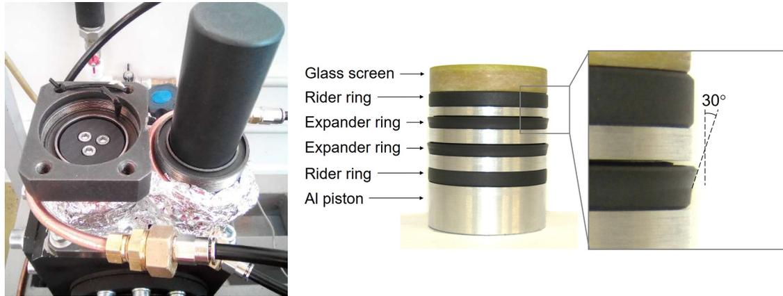
Fig. 6. Piston-cylinder pairs. On the left: Installed piston pairs for compressor and expander with dismounted cold head. On the right: the external view of the aluminum compressor piston with PTFE piston rings.
