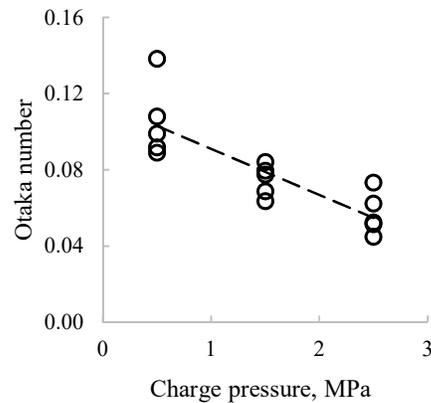
Fig. 3. Otaka number from the charge pressure.
