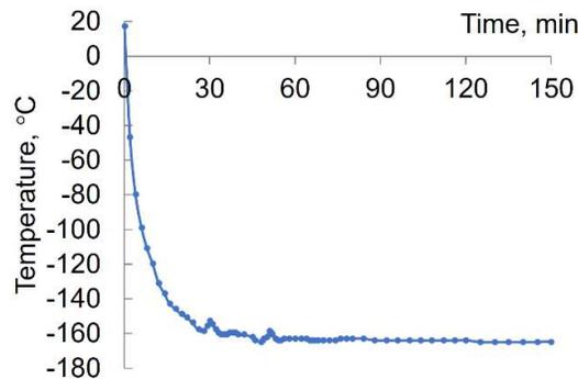
Fig. 11. Refrigerator temperature during operation with the dry-friction seal after the cumulative operation of 19 refrigerator hours.
