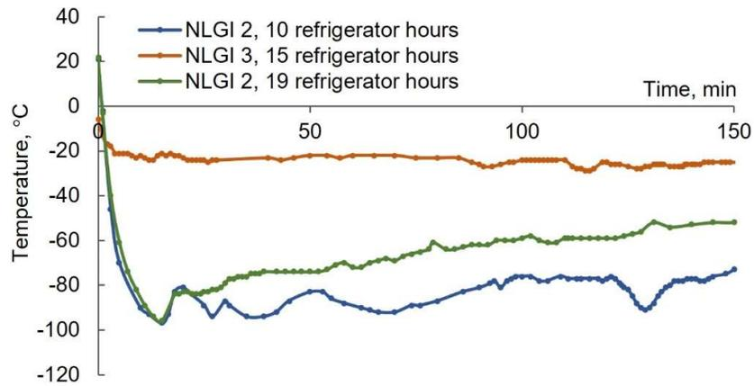
Fig. 7. Refrigerator temperature during operation for different lubricant and after different cumulative operation time of the refrigerator: “10 refrigerator hours” means that before this test the total cumulative operation of the PCP was 10 h.
