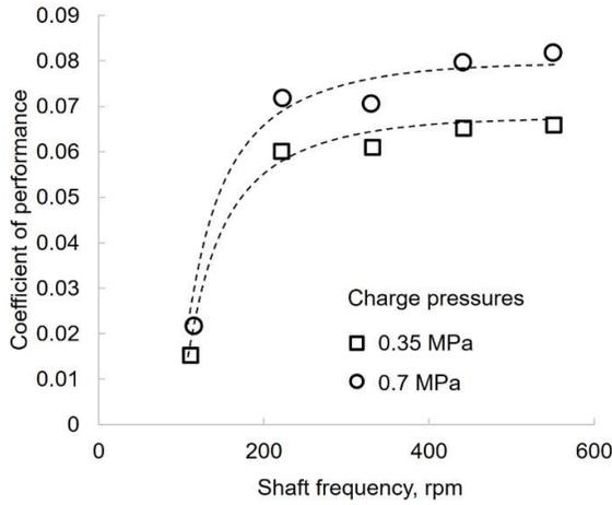
Fig. 7. Coefficient of performance as a function from shaft frequency and charge pressures.
