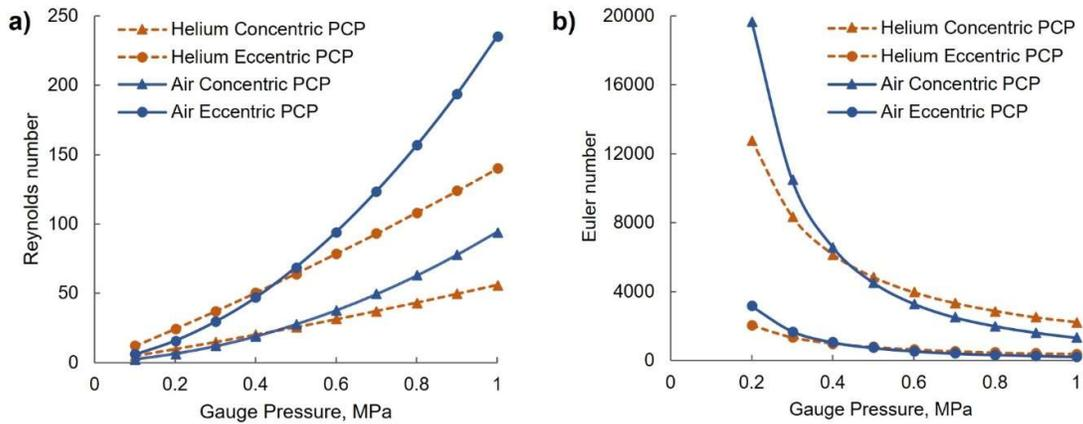
Fig. 6. Calculated Reynolds (a) and Euler (b) Numbers for concentric and eccentric PCP with air and helium as working medium. Absolute pressure after the gap for air PCP is 101.3 kPa and for helium PCP is 2.5 MPa.
