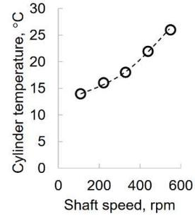
Fig. 8. Measured cylinder temperature with dismantled cold head and heat exchangers.
