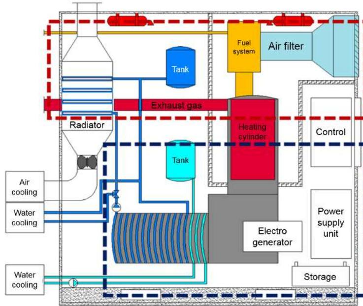
Fig. 4. Stirling m-CHP. Red dashed line is the boundaries of the thermal system, blue dashed line is the boundaries of the mechanical system [9].
