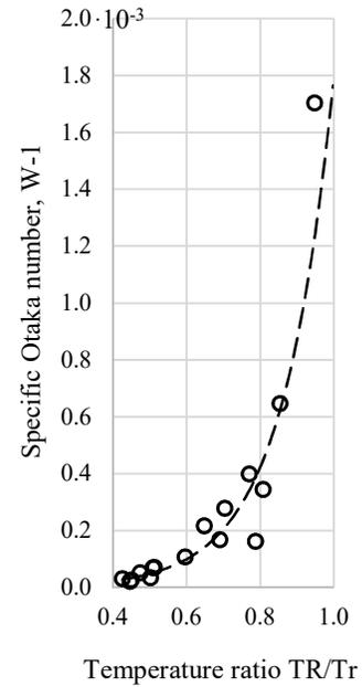
Fig. 4. Specific Otaka number from temperature ratio.
