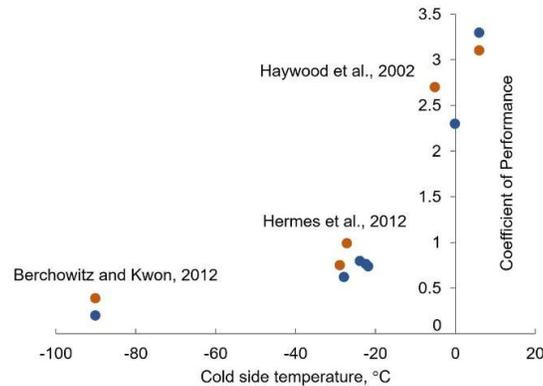
Fig. 1. Empirical comparison of COP values for vapor-compression refrigerators (blue) and Stirling refrigerators (orange).
