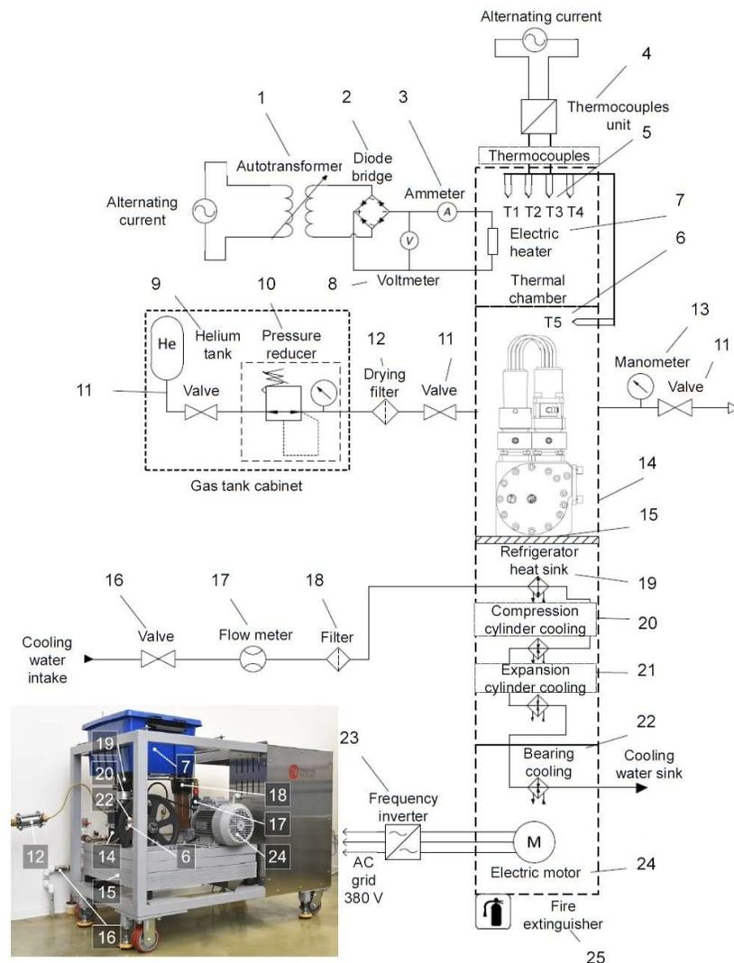
Fig. 8. Principal diagram and external view of the in-house Stirling refrigerator test rig.
