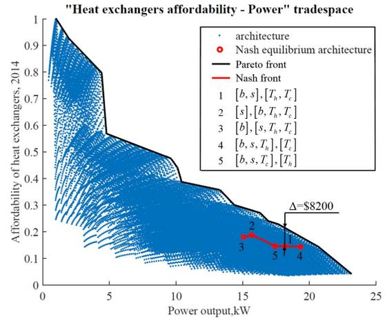
Fig. 7. Tradespace of 49,200 m-CHP architectures, Case 2.
