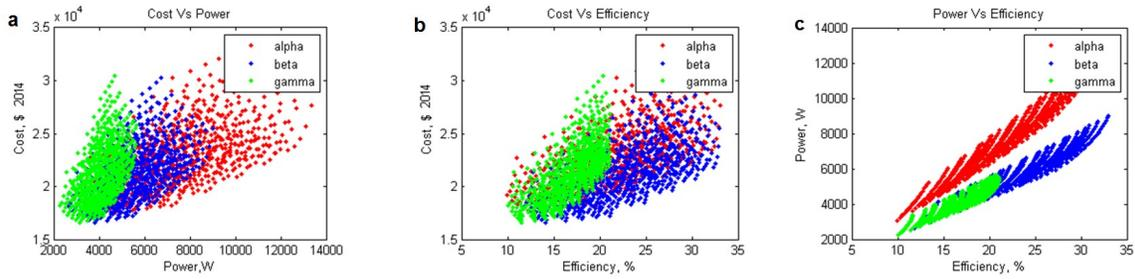
Fig. 21. Engine architecture tradespace, (a) Cost-Power trade-off; (b) Cost-Efficiency trade-off; (c) Power-Efficiency trade-off. Reprinted from [49].
