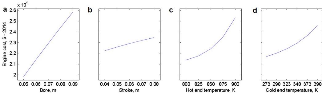
Fig. 23. Main effects of (a) bore; (b) stroke; (c) hot temperature, (d) cold temperature (from left to right) on the alpha-type engine cost. Reprinted from [49].
