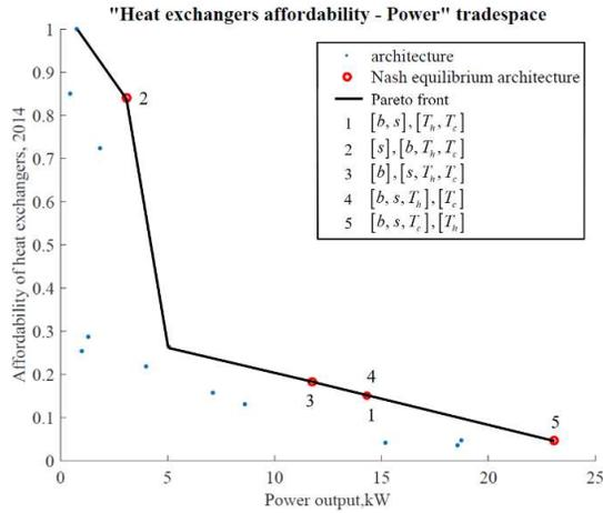
Fig. 6. Tradespace of 16 m-CHP architectures, Case 1.
