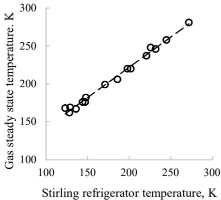
Fig. 2 Relation between gas and refrigerator temperatures measured in the experiment.
