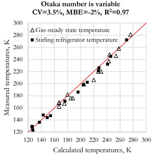
Fig. 6. Measured and calculated temperatures in the thermal chamber, with a variable Otaka number.
