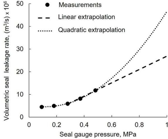
Fig. 5. Measured leakage rate for dry (no lubricant) PCP from varying pressure gradient. Dotted and dashed lines are the quadratic and linear extrapolations correspondingly for experimental points.
