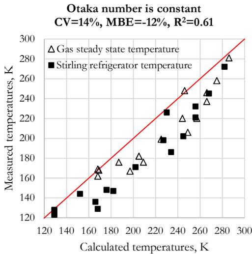
Fig. 5. Measured and calculated temperatures in the thermal chamber with a constant Otaka number.
