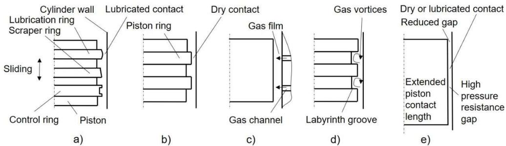
Fig. 2. Illustrative representation of piston-cylinder seal types in Stirling machines: a) Lubricated piston rings, b) dry-friction piston rings c) gas bearing, d) labyrinth seals, and e) analyzed in this work high-tolerance seal.
