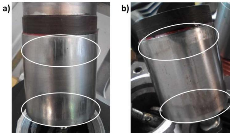
Fig. 8. Expansion (a) and compression (b) piston with worn-out areas on the surface (white).
