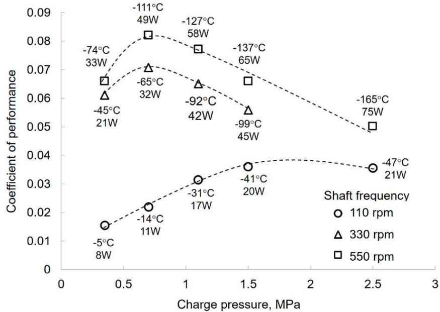
Fig. 9. The coefficient of performance from the refrigerator charge pressure and the shaft frequency. Each point indicates the steady-state cold head temperature and the cooling capacity.
