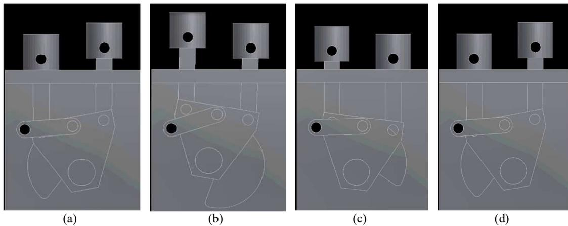
Fig. 7. Schematic depiction of the Ross-yoke drive with instantaneous cycle pictures. The compressor piston is on the left, the expander piston is on the right: a) the beginning of compression, b) the end of compression and beginning of expansion, c) the end of expansion d) the beginning of compression. Credit for the dynamic model of the mechanical drive: Vladimir Dvorzov.
