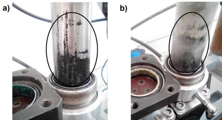
Fig. 9. Displacer surface covered with NLGI 2 (a) and NLGI 3 (b) lubricant (black), which was squeezed out from the gap during operation.
