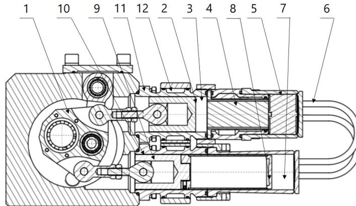
Fig. 3. Internal structure of the in-house Stirling refrigerator [29]: 1 kinematic drive of Ross-yoke type; 2 compression piston; 3 compression space; 4 water-cooled radiator; 5 regenerator; 6 heat exchanger; 7 expansion space; 8 displacer; 9 expansion piston; 10 piston-cylinder sealing gap; 11 compression cylinder; 12 cooling jacket.
