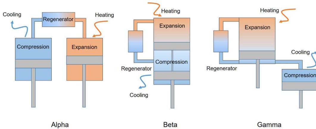
Fig. 19. Schematic views of different kinematic configurations of Stirling engines: alpha, beta and gamma types.
