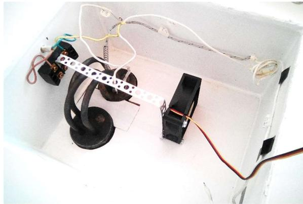
Fig. 4. Internal view of the thermal chamber with the cold head, air fan and thermocouples. External view is in Fig. 8.
