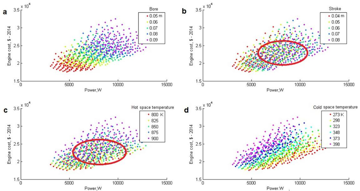
Fig.22. Architectures of the alpha-type engine colored by different design parameters: (a) bore, (b) stroke, (c) hot space temperature, (d) cold space temperature. Reprinted from [49].
