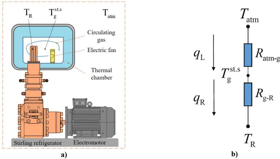
Fig. 1. Thermal system “Stirling refrigerator – Thermal chamber”: a) principal diagram with key elements b) Thermo-electrical analogy.
