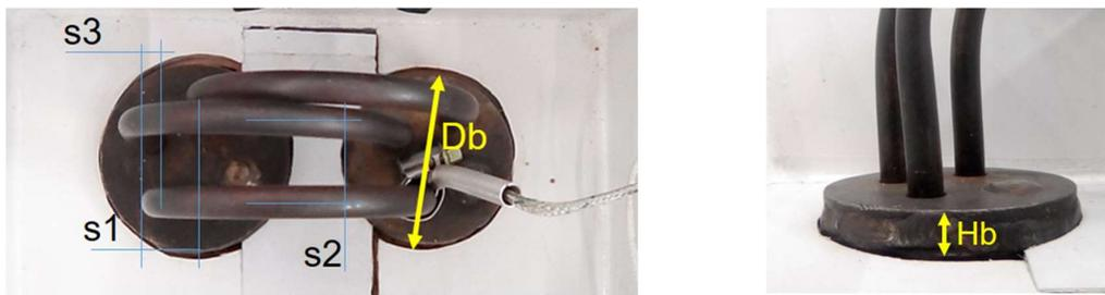
Fig. 5. External views of the cold head inside the thermal chamber with key geometrical parameters: the top view (left) and the approach flow view (right).
