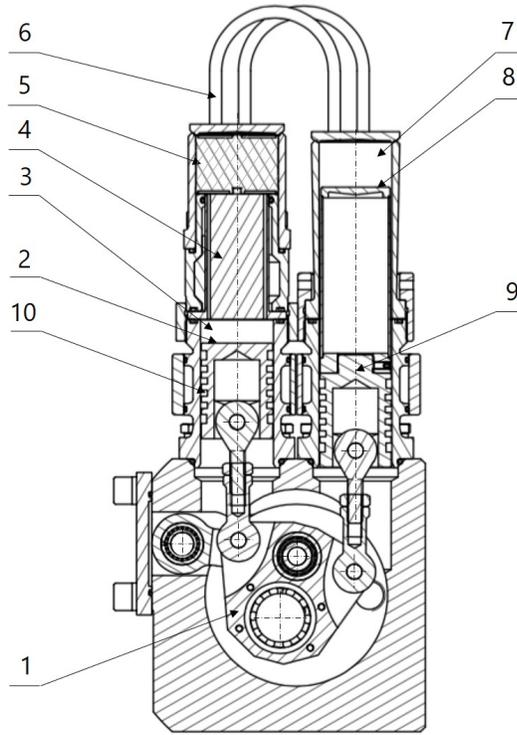
Fig. 3. Internal structure of the Stirling refrigerator TM1.
