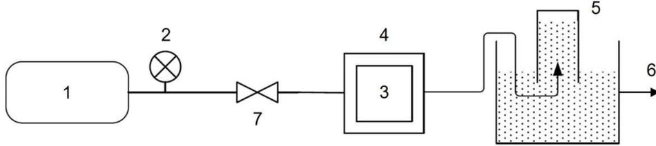
Fig. 4. Schematic diagram for measurements of gas leakage: 1 compressor receiver; 2 manometer; 3 piston; 4 cylinder with plugs; 5 control volume; 6 hydraulic locking; 7 valve.
