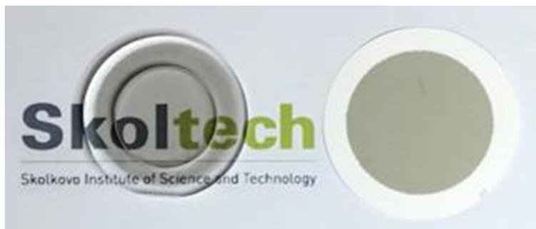
**Figure 4.3:** Photo of a free-standing thin film (left) and thin film on a filter of SWCNTs (thickness of the film is about 60 nm in both cases) produced by the spark discharge aerosol CVD method.
