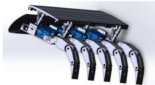
Figure 3-41: The design of the adaptive wing segment in SolidWorks software
