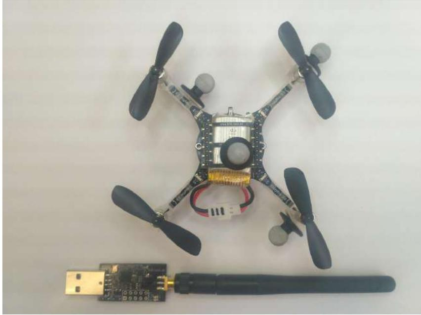
Figure A-7: Crazyflie 2.0 quadrotor with four IR reflective markers and 2.4 GHz Crazyradio.
