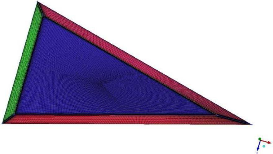
(b) Structured mesh on the surface of the model
