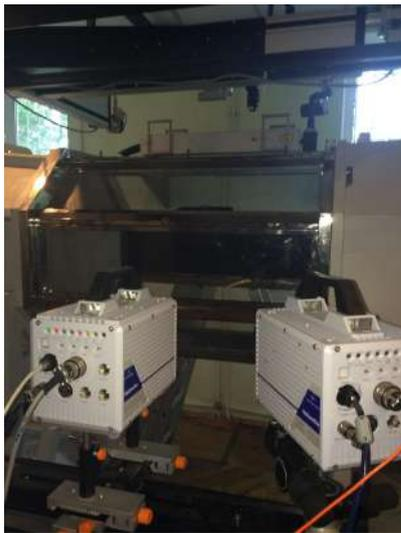
(a) Videogrammetry system in front of the wind tunnel
