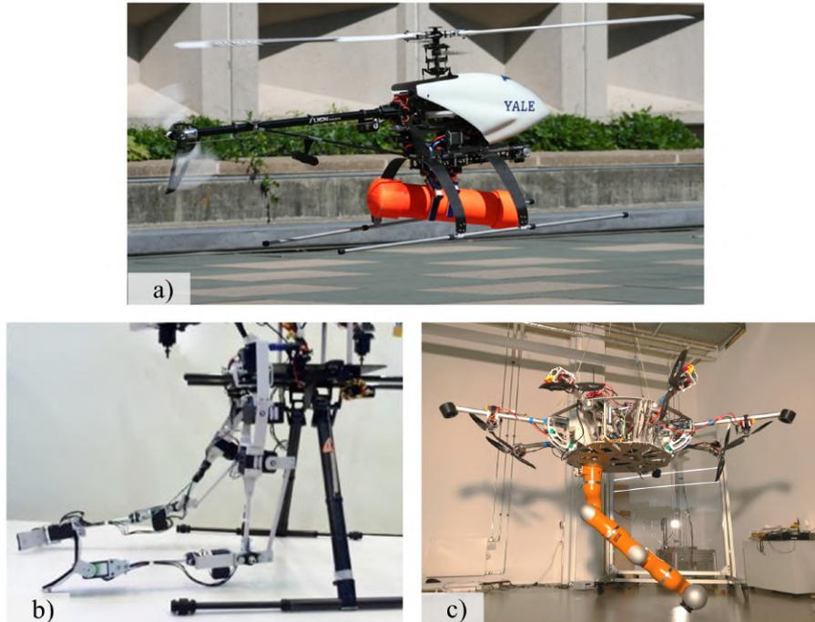
Figure 2-1: Types of aerial manipulators: (a) 1-DoF gripper [Pounds et al., 2011], (b) two multi-DoF robotic arms [Suarez et al., 2018], (c) cable-Suspended manipulator [Sarkisov et al., 2019].
