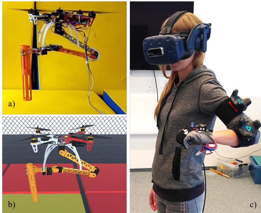
Figure 3-1: The flight test of the aerial manipulation. a) Robot during teleoperation. b) VR visualization in Unity. c) Operator with HMD and wearable interface.
