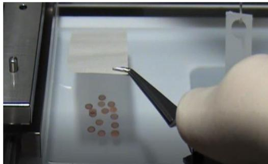
**Figure 19.** Transfer dendrimer film on copper grids for TEM analysis.
