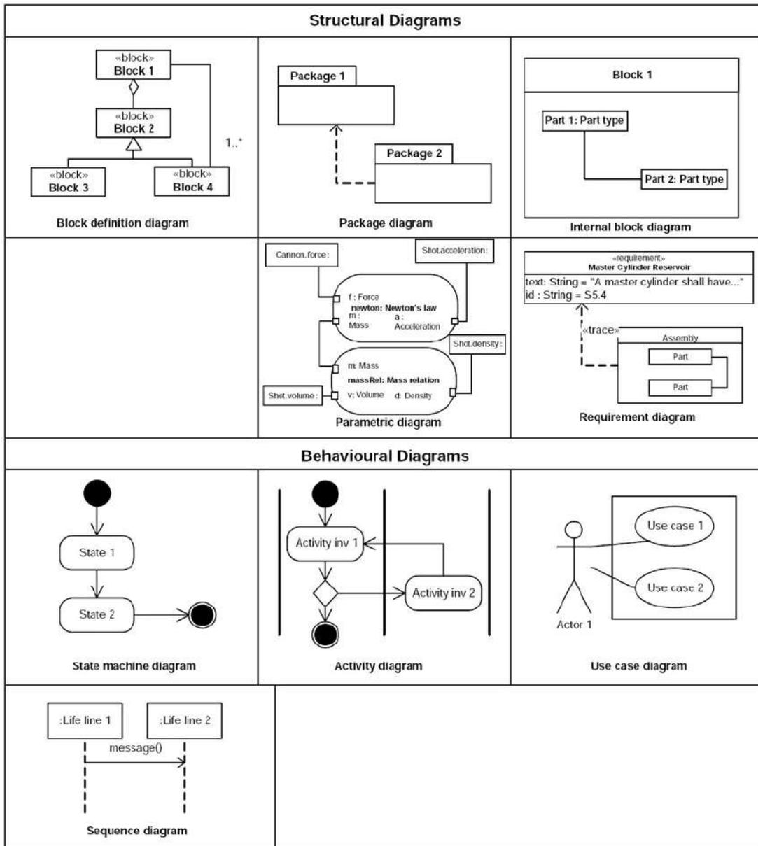
Figure 2.7: SysML diagrams (Holt and Perry 2008)
