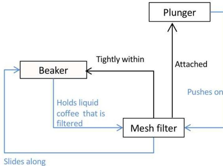
Figure 3.38: Structure and interactions for French Press concept
