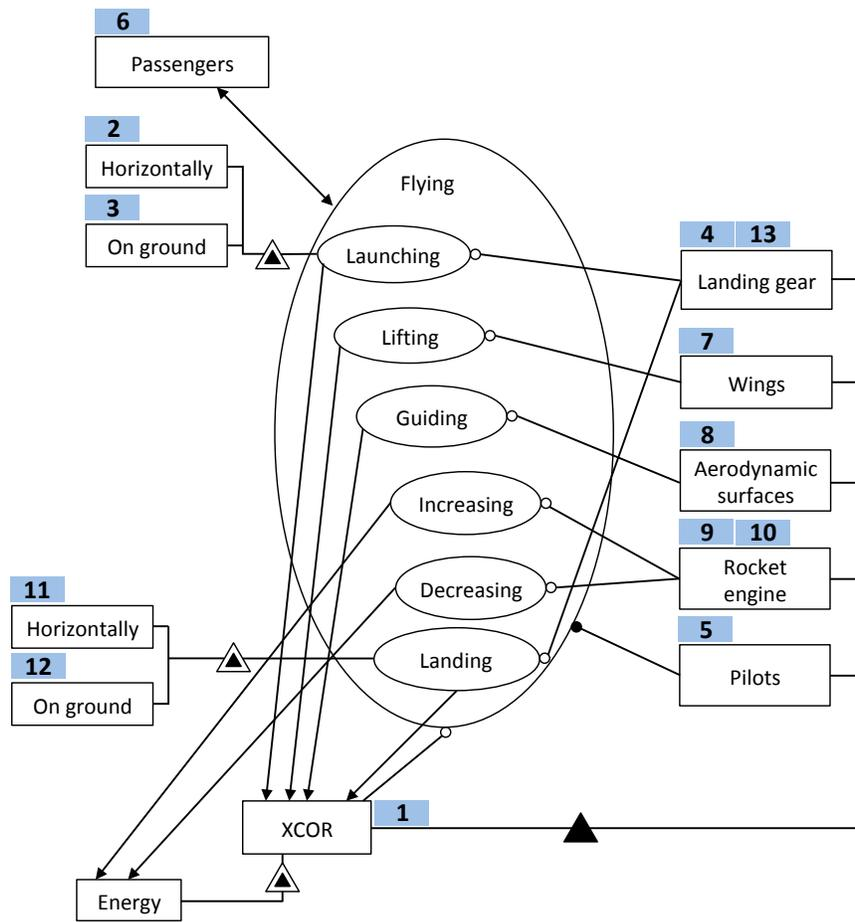
Figure 5.52: Architectural decisions in solution diagram for XCOR
