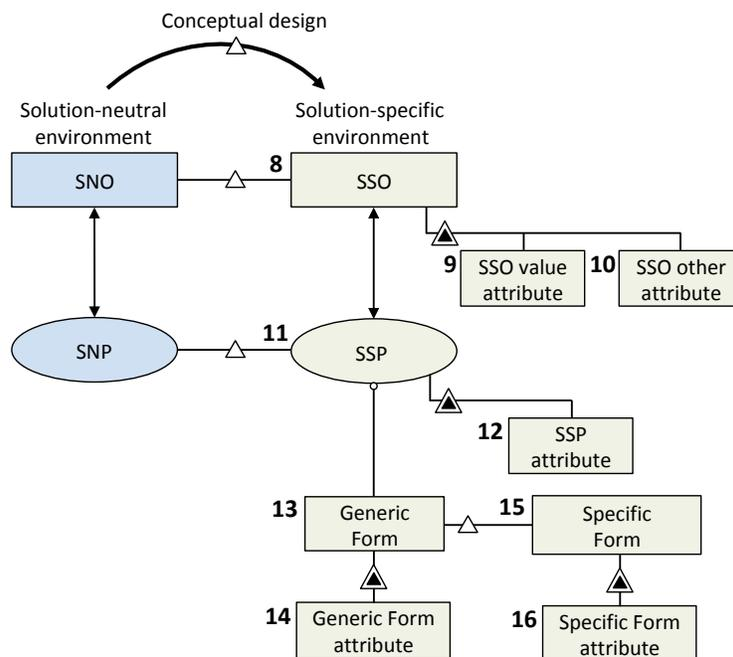
Figure 3.7: Model-based representation of conceptual design process
