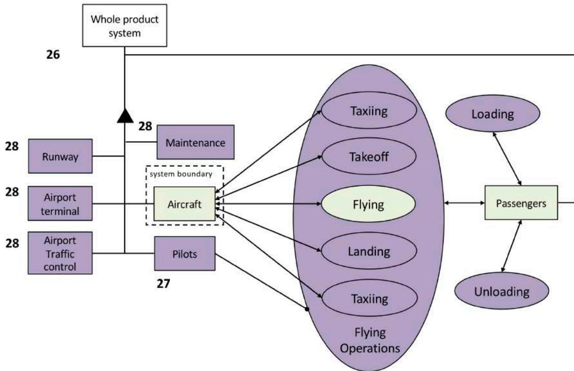
Figure 3.25: Concept of Operations for aircraft concept
