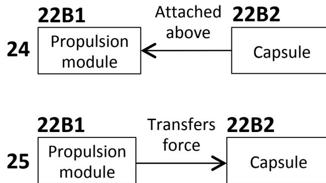
Figure 5.9: Structure and Interactions for Blue Origin concept
