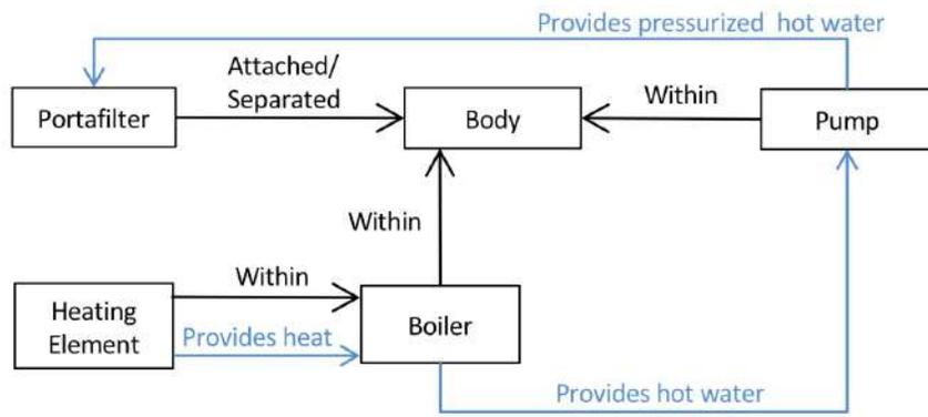
Figure 3.37: Structure and interactions for Espresso Machine concept
