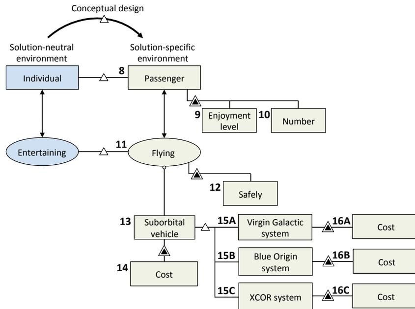
Figure 5.5: Solution-specific (III) proposition for suborbital concept
