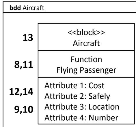
Figure 3.28: Solution-specific (III) proposition for aircraft concept in SysML
