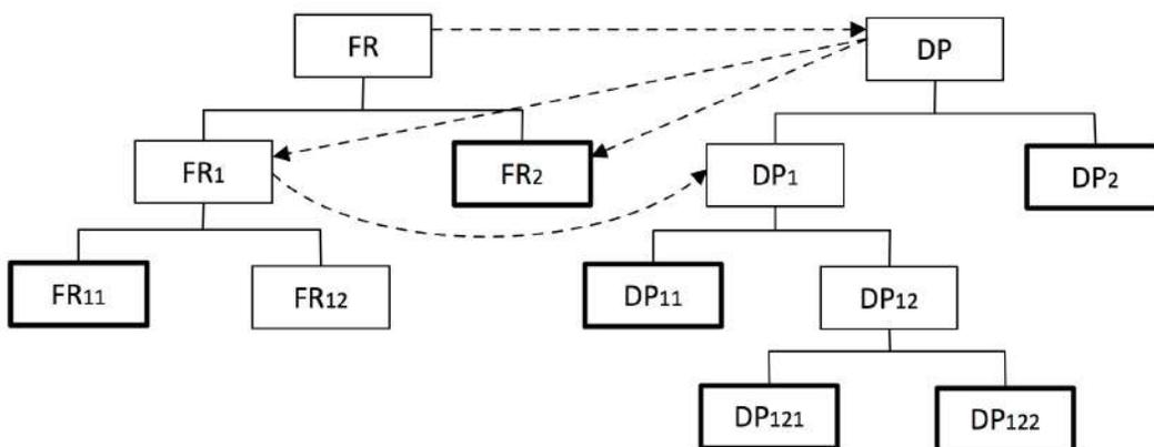
Figure 2.2: Zigzagging process
