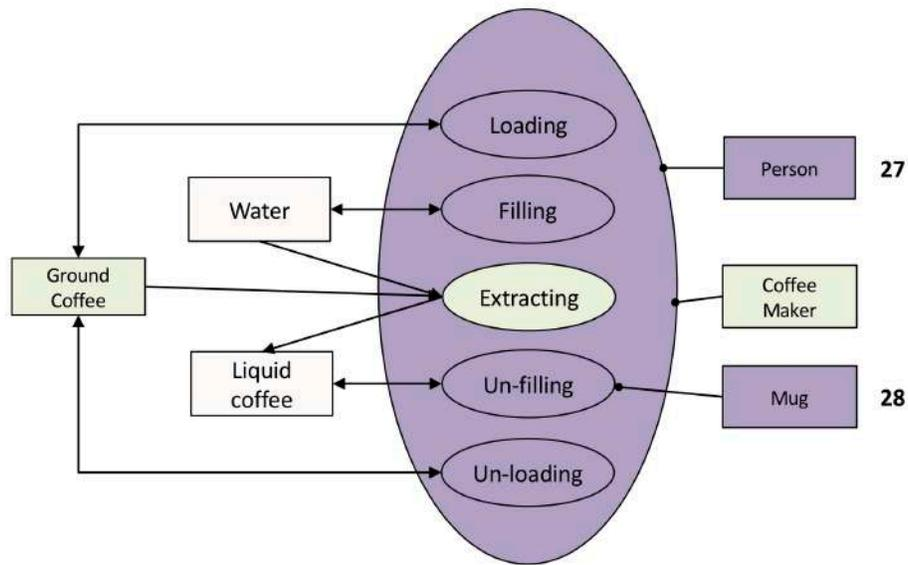
Figure 3.39: Concept of Operations for Coffee Maker concept
