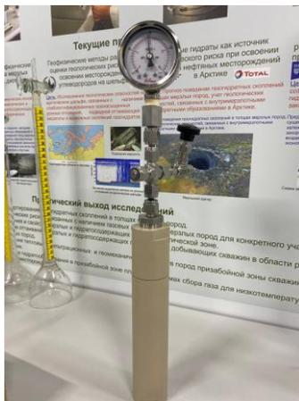
Figure 73: Manufactured high-pressure NMR cell for gas–pressure measurements.
