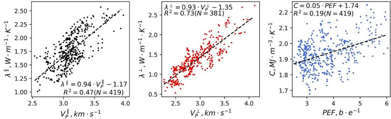
**Figure 5.** Results of correlation analysis between thermal conductivity and sonic velocity of rocks for parallel (left panel) and perpendicular (central panel) direction to the bedding plane and rock volumetric heat capacity and photoelectric factor (right panel). Dashed line represents the regression trend.
