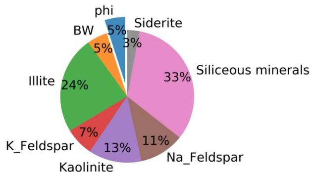
**Figure 13.** Pie chart of average volume fractions of rock-forming components of the investigating rocks inferred from high definition spectroscopy and nuclear magnetic resonance log data.
