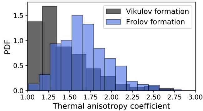
**Figure 33.** The histogram of thermal anisotropy coefficient for the Vikulov (black colour) and the Frolov (blue colour) formations.
