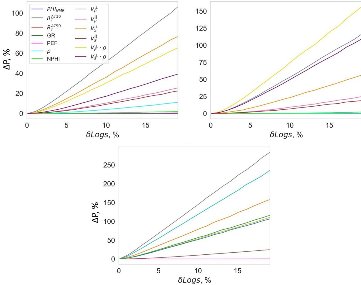
**Figure 10.** Results of sensitivity study of regression models of gradient boosting for determining thermal conductivity parallel (left panel) and perpendicular (right panel) to bedding plane and volumetric heat capacity (bottom panel) of carbonate rocks of heavy oil field.
