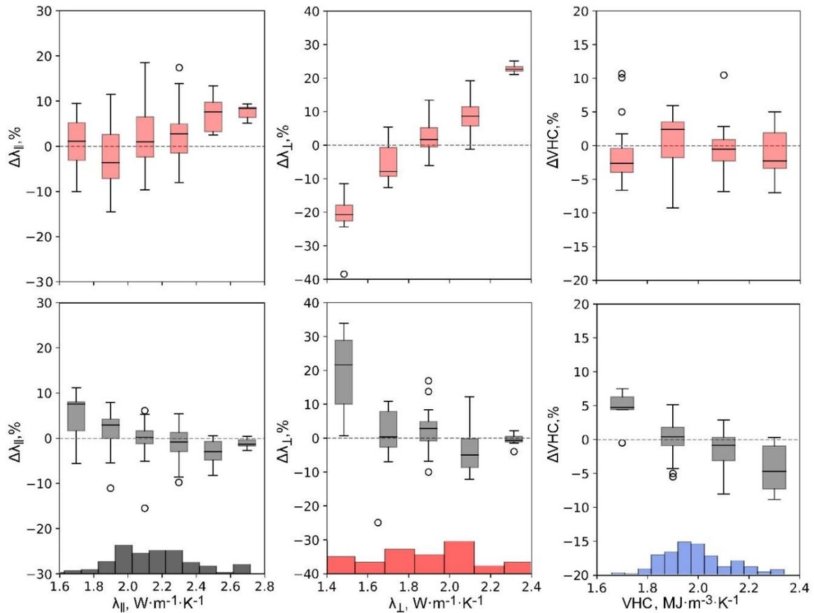
**Figure 25.** Boxplots of the relative discrepancies between the measured and predicted values of rock thermal properties for the Domanic Formation. Above, determinations based on the theoretical models; below, determinations based on the gradient boosting algorithm. Histograms of thermal properties from the test dataset are also shown.
