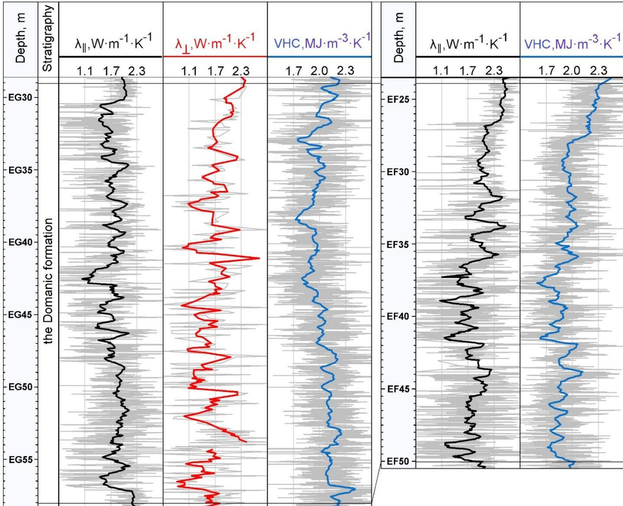
**Figure 22.** Results of rock thermal property measurements for wells F (left) and G (right).  $\lambda$  stands for rock thermal conductivity, subscripts  $\parallel$  and  $\perp$  stand for the thermal conductivity components in the directions parallel and perpendicular to the bedding plane, respectively; grey lines represent the original profiles of the rock thermal properties. Black, red and blue lines represent averaged thermal property profiles in a moving 0.5 window.
