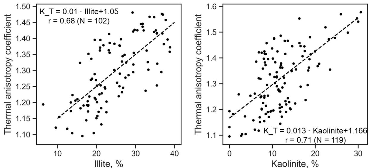
**Figure 26.** Cross-plots between thermal anisotropy coefficient and illite volume fraction (left panel) and thermal anisotropy coefficient and kaolinite volume fraction (right panel). The dashed lines represent the regression trend.
