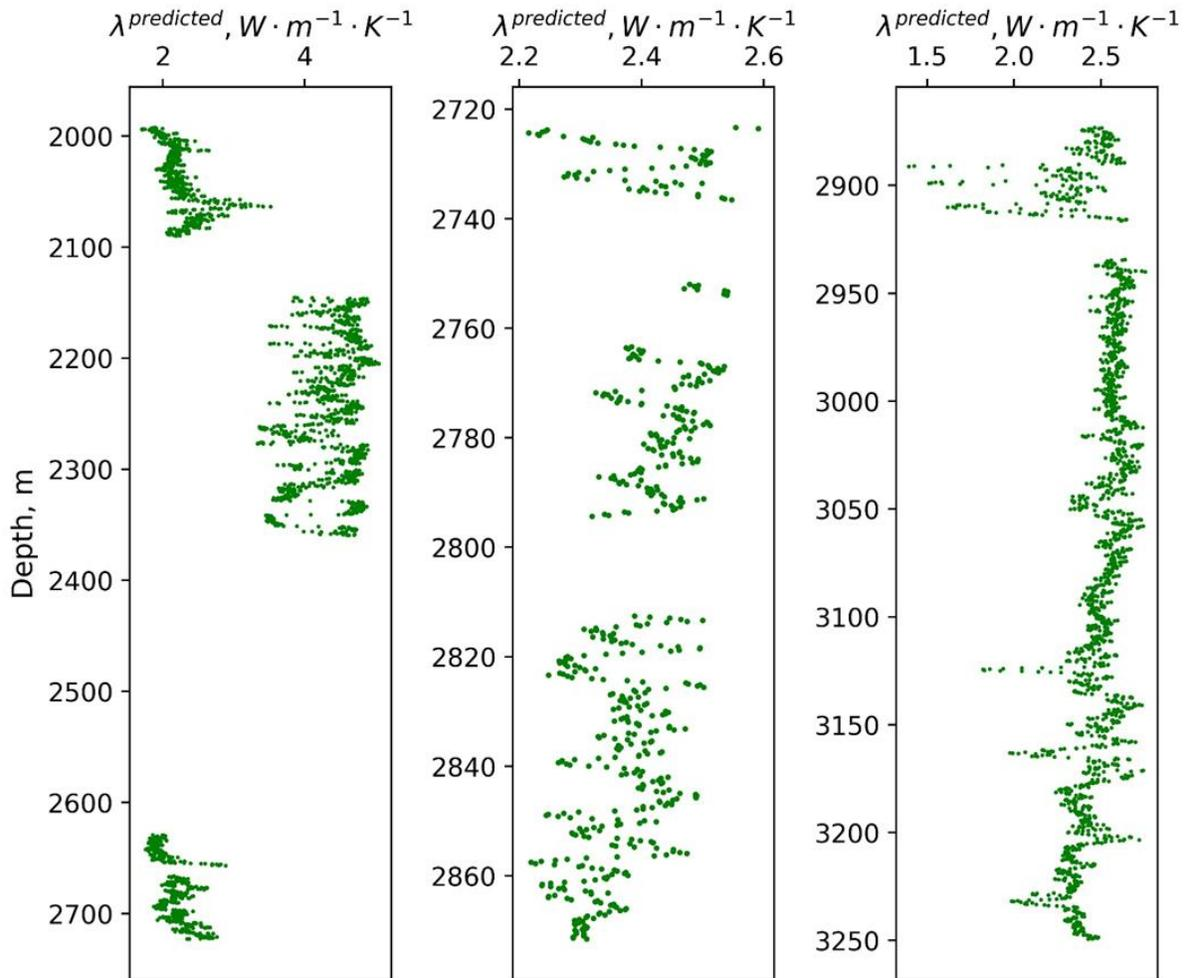
**Figure 45.** Thermal conductivity within not cored depth intervals predicted from well-logging data by means of the established regression equations.
