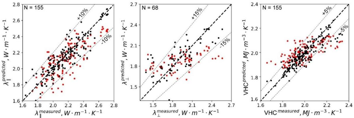
**Figure 24.** Experimental data of the rock thermal properties compared to the thermal properties predicted from well-logging data of training datasets for the Domanic Formation. Black dots present results with the gradient boosting method, red dots results via theoretical model. The dashed black line ( $y=x$ ) shows a perfect determination.
