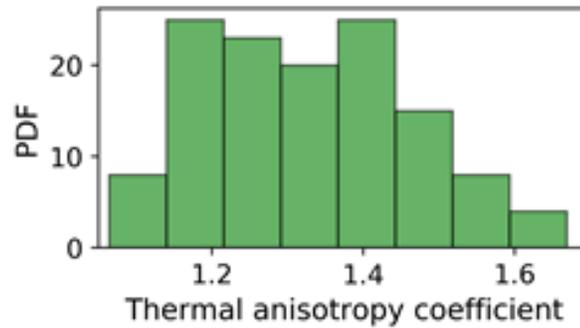
**Figure 15.** Histogram of thermal anisotropy coefficient inferred from thermal core logging for wells A and C.
