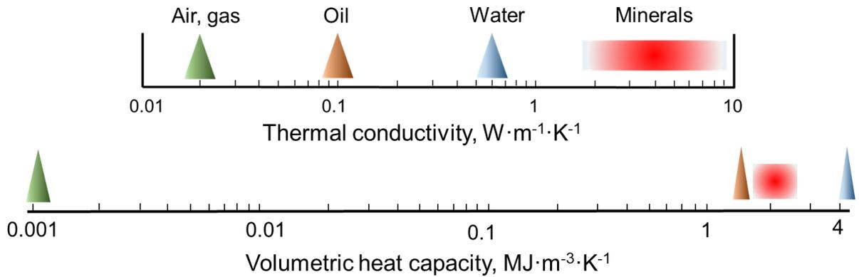
**Figure 2.** Thermal conductivity and volumetric heat capacity for rock-forming minerals and pore fluids.
