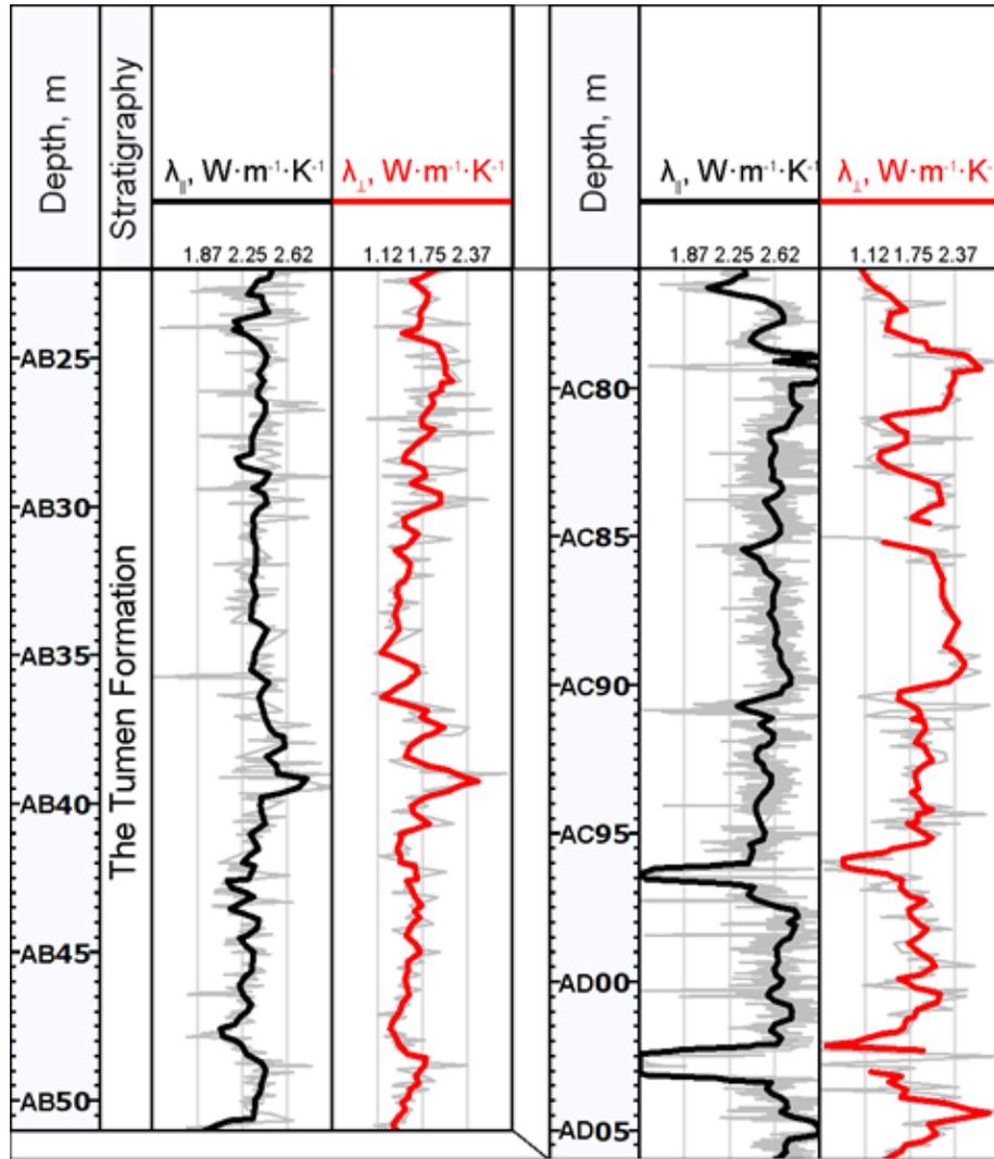
**Figure 14.** Results of rock thermal property measurements for wells A (left) and C (right).  $\lambda$  stands for rock thermal conductivity; subscripts  $\parallel$  and  $\perp$  stand for the thermal conductivity components in the directions parallel and perpendicular to the bedding plane, respectively; grey lines represent the original profiles of the rock thermal properties; black, red and blue lines represent averaged thermal property profiles in a moving 0.5 window.
