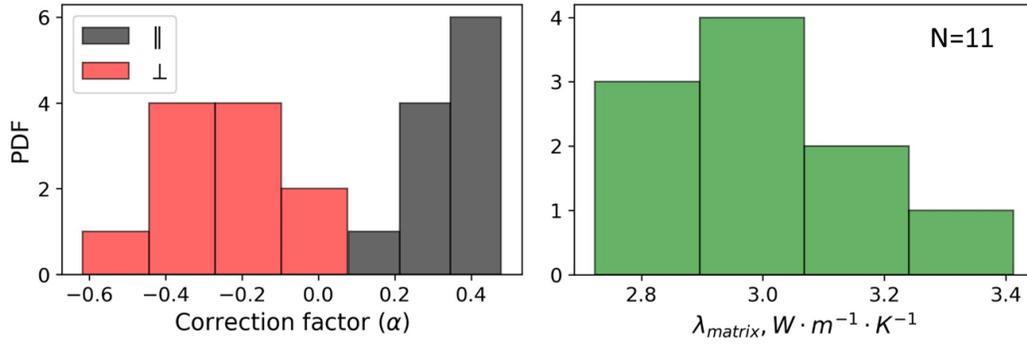
**Figure 34.** The histogram of the determined correction factors for parallel (black colour) and perpendicular (red colour) directions to the bedding plane and thermal conductivity of rock matrix (right panel).
