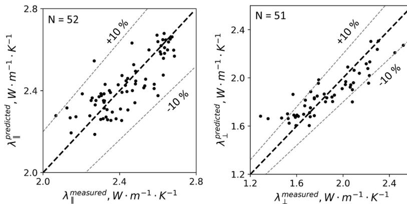
**Figure 16.** Experimental data of the rock thermal conductivity compared to the predicted thermal conductivity from well-logging data on test datasets. The dashed black line ( $y=x$ ) shows perfect determination. N stands for number of points.
