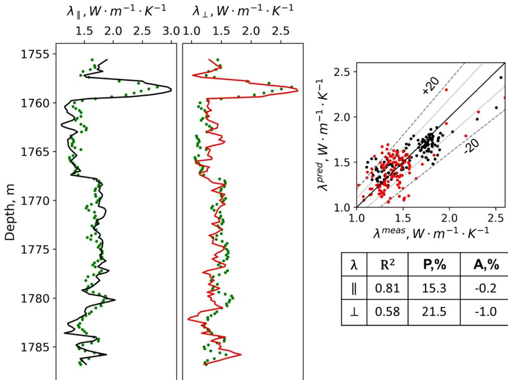
**Figure 35.** The results of predicting the thermal conductivity of rocks and assessment of determination quality for the Vikulov Formation. Black and red curves (left panel) represent measured values of thermal conductivity for parallel and perpendicular directions to the bedding plane, respectively. Green dots represent the predicted thermal conductivity. Determination quality is reported for a 0.95 confidence level.
