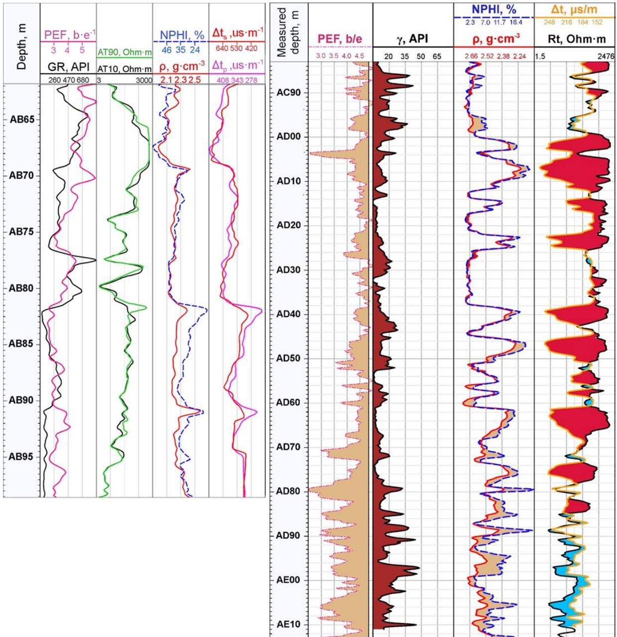
**Figure 8.** Results well logging for wells A (left panel) and E (right panel).
