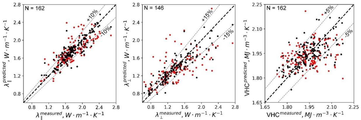
**Figure 11.** Experimental data of the rock thermal properties compared to the thermal properties predicted from well-logging data of training datasets for the Bazhenov Formation. Black dots present results with the gradient boosting method, red dots results via theoretical model. The dashed black line ( $y=x$ ) shows a perfect determination.
