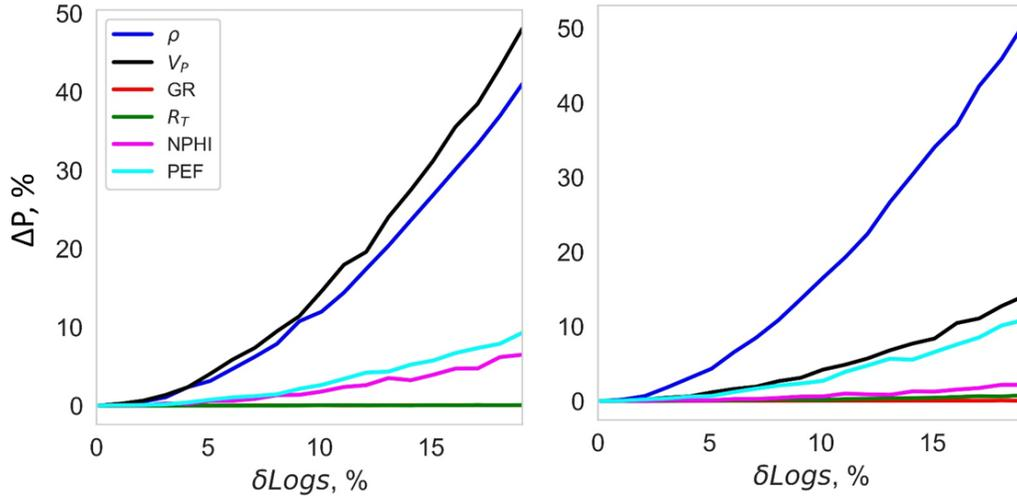
**Figure 9.** Results of sensitivity study of regression models of gradient boosting for determining thermal conductivity (left panel) and volumetric heat capacity (right panel) of carbonate rocks of the heavy oil field. The input well-logs are presented on the left panel.  $\Delta P$  stands for relative change of determination precision.  $\Delta Logs$  stands for input well-log with imposed uncertainty.
