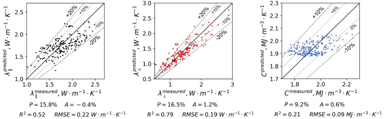
**Figure 6.** Results of determination of thermal conductivity for parallel (left panel) and perpendicular (central panel) direction to the bedding plane from sonic velocity and rock volumetric heat capacity from photoelectric factor (right panel). Solid line presents a perfect determination of rock thermal properties ( $x=y$ ), grey dashed lines present the determination uncertainty intervals.
