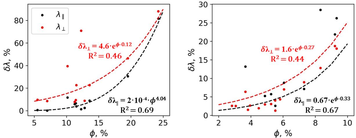
**Figure 31.** The dependency of relative increase of thermal conductivity after water saturation from porosity for the Vikulov and Frolov formations (left panel) and for the Abalak and Tyumen formations (right panel). Red colored dots and regression trend represent data for thermal conductivity perpendicular to the bedding plane. Black colored dots and regression trend represent data for thermal conductivity parallel to the bedding plane.
