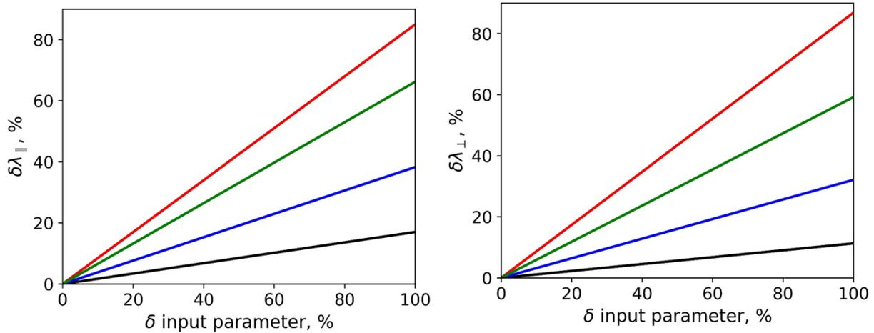
**Figure 17.** Results of assessing influence of uncertainty in thermal conductivity of rock matrix (red lines), porosity (green line), thermal conductivity of pore fluid (blue line), and correction factor (black line) on rock thermal conductivity for parallel (left panel) and perpendicular (right panel) directions to the bedding plane.
