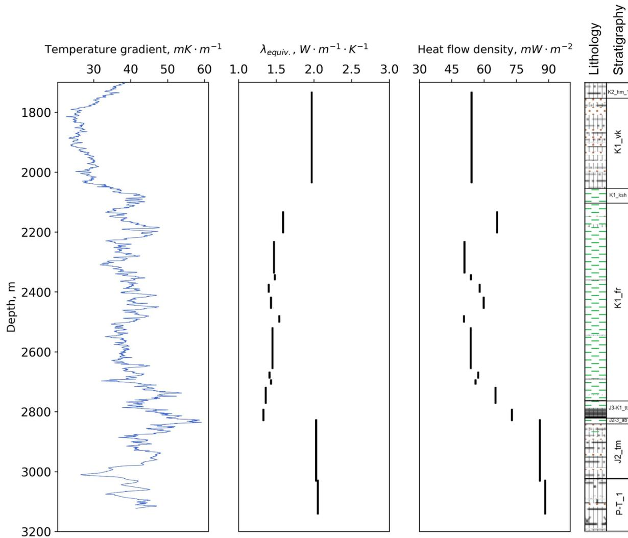
**Figure 39.** Results of determining temperature gradient, equivalent thermal conductivity of rocks and the heat flow density within 14 depth intervals. Lithology legend was given in Figure 38 (Popov et al., 2021a).
