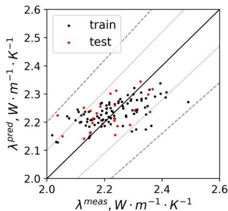
**Figure 36.** The cross-plot of measured and predicted values of thermal conductivity parallel to the bedding plane.
