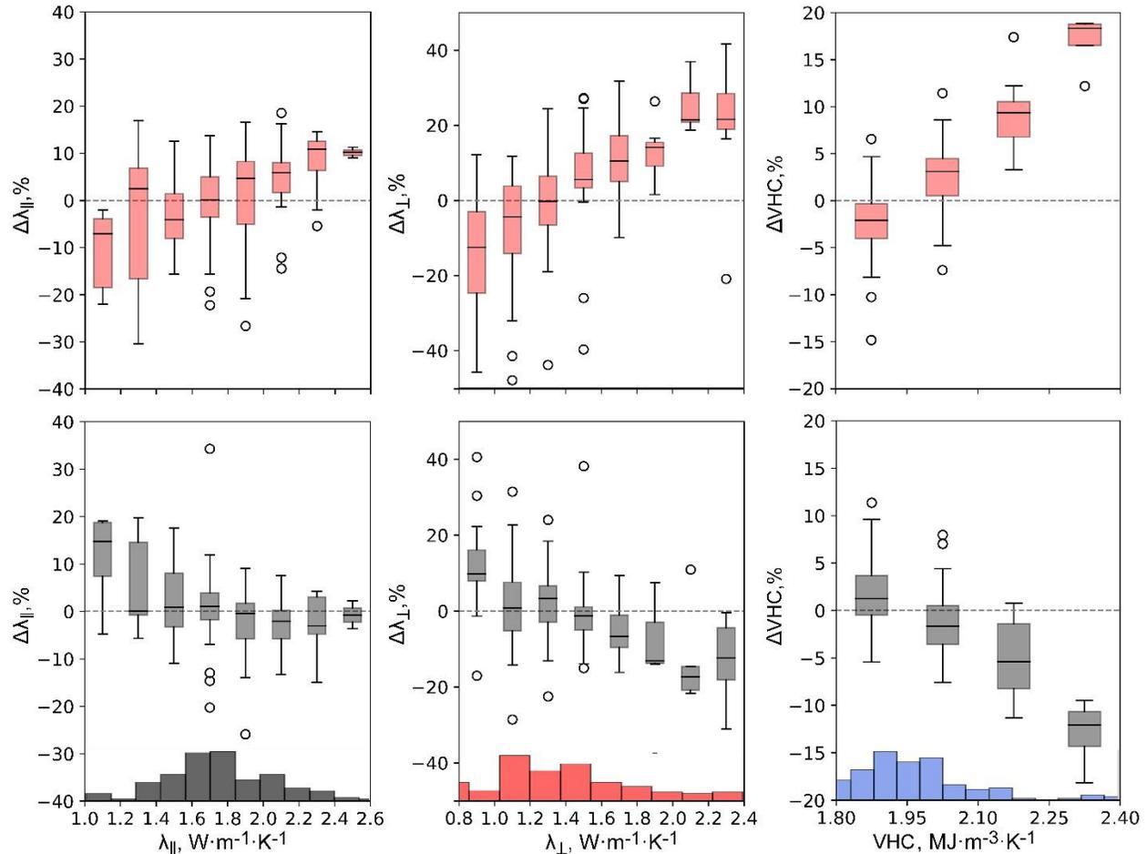
**Figure 12.** Boxplots of the relative discrepancies between the measured and predicted values of rock thermal properties for the Bazhenov Formation. Above, determinations based on the theoretical models; below, determinations based on the gradient boosting algorithm. Histograms of thermal properties from the test dataset are also shown.
