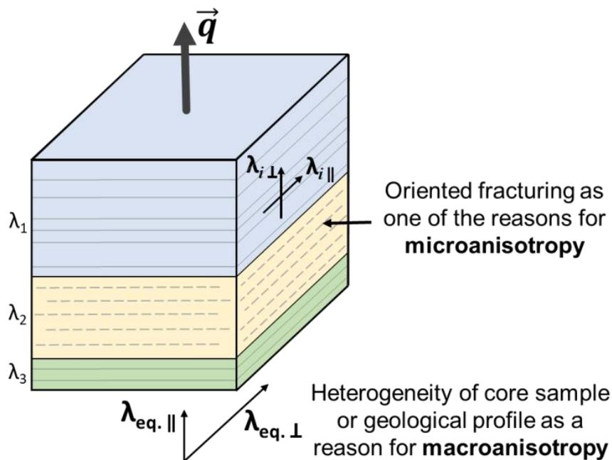
**Figure 46.** The reasons causing anisotropy of rocks that were accounted during determining equivalent thermal conductivity required for calculating heat flow density.  $\lambda_{eq.}$  – macroanisotropy,  $\lambda_{i\perp}$  - microanisotropy (Popov et al., 2021b).
