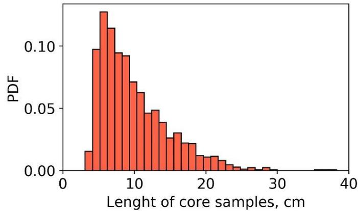
**Figure 42.** Distribution histogram for the length of full-sized cores under study (Popov et al., 2021b).
