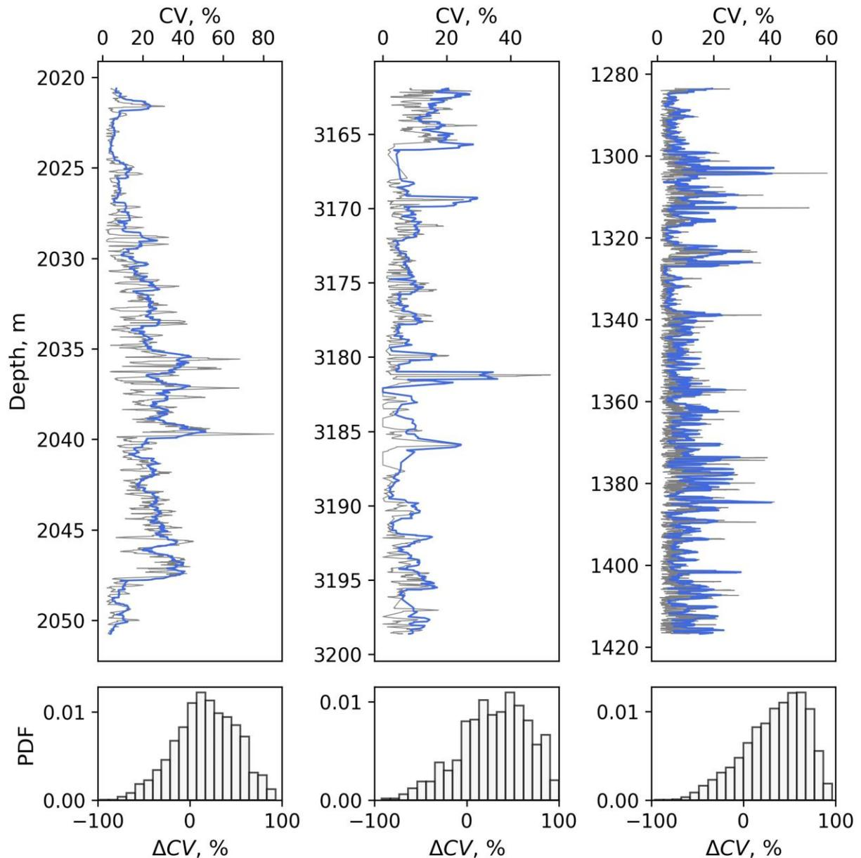
**Figure 1.** Coefficient of variation for rock thermal properties for two organic-rich shales (left and central panel) and carbonate rocks of heavy oil field (right panel) within moving windows of 0.1 m (grey colored line) and 0.5 m (blue) colored line. Histograms plot relative difference between variation coefficient calculated within 0.5 m and variation coefficient calculated within 0.1 m.
