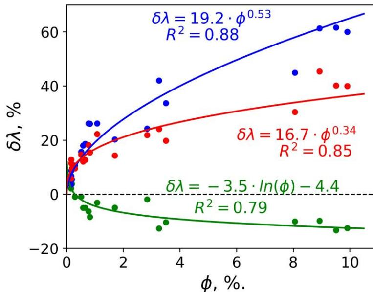
**Figure 44.** Thermal conductivity variations with porosity after drying core samples (green-coloured line) and after water saturation under vacuum (blue-coloured line) (Popov et al., 2021b). The red-coloured line characterizes the thermal conductivity change from «as received» state to «water-saturated».
