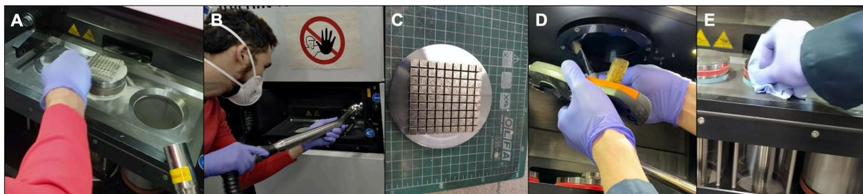
**Figure 2.13.** Exemplary machine recovery operations<sup>20</sup>: (a) brushing the excessive powder to the overflow hopper (note the vacuum cleaner head sucking the particles from the air, bottom right corner); (b) vacuuming the build chamber; (c) deinstalled build plate; (d) cleaning the lens; (e) wiping the hopper sealings with alcohol.
