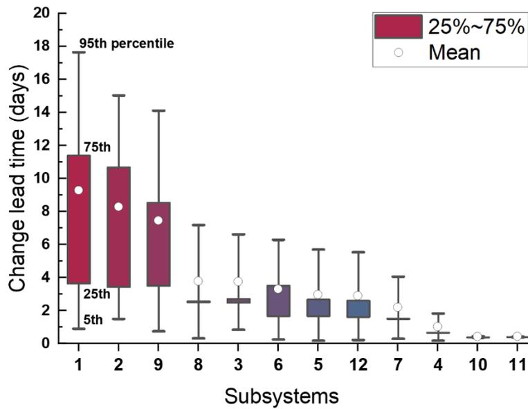
**Figure 5.10.** Simulation-based evaluations of change lead times for the pylon subsystems. Subsystems' numbers in the order of appearance on the X axis (left to right): (1) Front engine mount, (2) Firewall, (9) Fire extinguishing system (FireX), (8) Fire detection, (3) Rear engine mount, (6) Bleed air duct, (5) Fuel lines, (12) Skin and panels, (7) Hydraulic lines, (4) Trailing edge, (10) Leading edge, (11) Electric harnesses.
