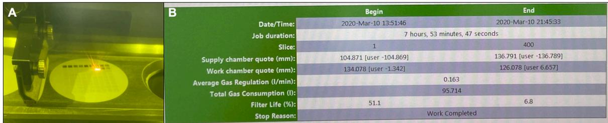
**Figure 2.12.** The LPBF process: (a) Photo of laser melting the powder; (b) fragment of the print statistics report<sup>19</sup>.
