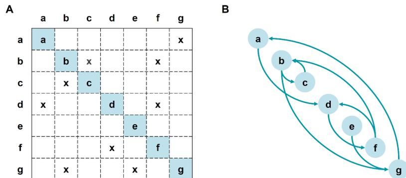
**Figure 4.1.** (a) binary DSM, (b) equivalent digraph form; adapted from (Eppinger and Browning, 2012).
