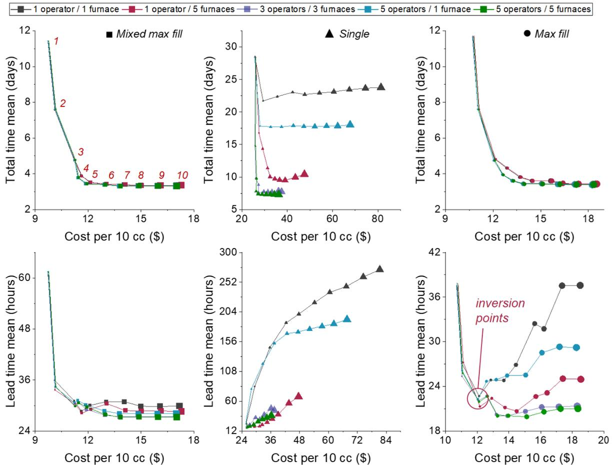
**Figure 4.17.** Comparison of average cost metric (\$/cc) versus average lead time and the total time of production. The symbol size designates an integer value of printers utilized: from the smallest for one machine to the largest for ten machines.
