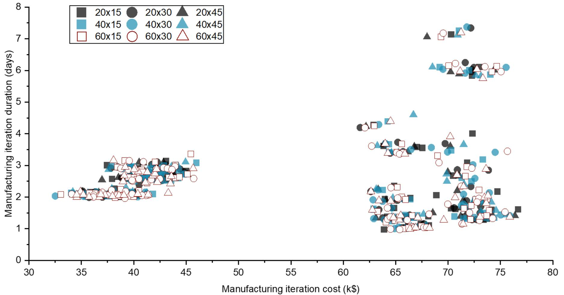
**Figure 5.27.** A time-cost map of possible configurations of the manufacturing system categorized by the layout parameters. A “60x15” configuration designates the system with 60 meters limit for the division width and 15 meters limit for the division length.
