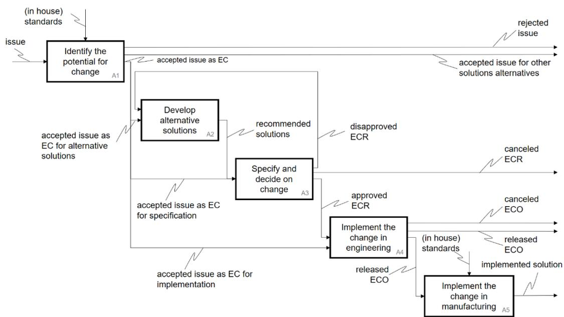
**Figure 2.4.** IDEF0 representation of the ECM reference process by SASIG, adapted from (VDA 4965, 2010c).
