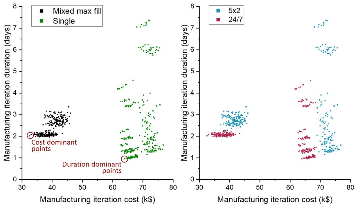
**Figure 5.25.** A time-cost map of possible configurations of the manufacturing system: (a) segregation of the points by the batching strategy; (b) segregation of the points by the shift mode.
