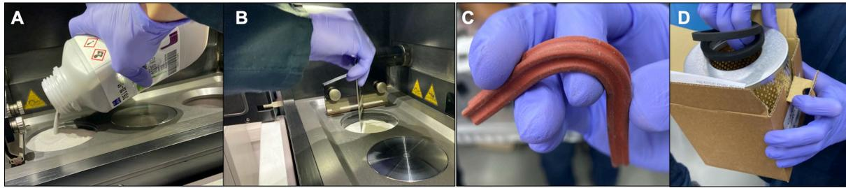
**Figure 2.11.** Exemplary machine setup operations<sup>18</sup>: (a) manual filling of the powder feed hopper; (b) manual compressing of the powder; (c) cracking defect on the blade resin gasket; (d) replaceable filter.
