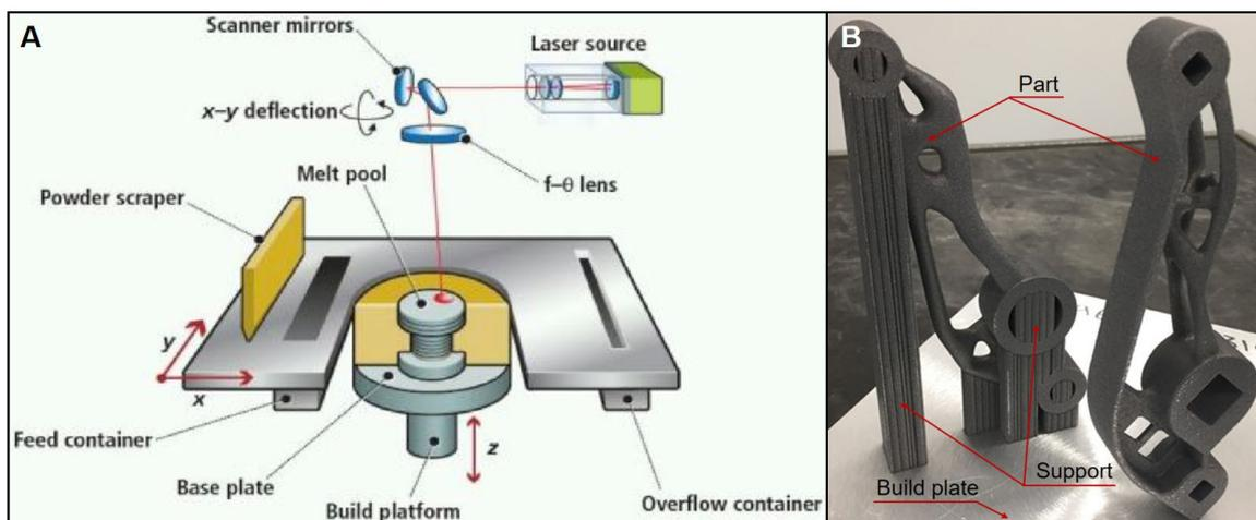
**Figure 2.10.** (a) LPBF principal scheme of operation (Schmidt *et al.*, 2017). (b) Two suspension bell-cranks produced via LPBF. Left: geometry-optimized bell-crank without manufacturing constraints applied. Right: geometry-optimized bell-crank with manufacturing constraints applied<sup>17</sup>.
