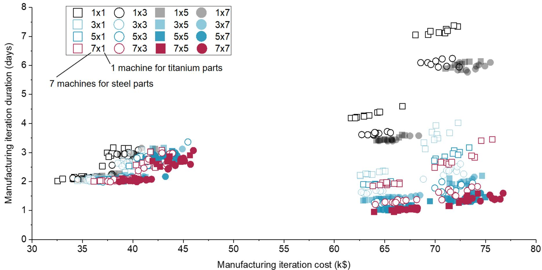
**Figure 5.26.** A time-cost map of possible configurations of the manufacturing system categorized by the number of printers in a system. A “7x1” configuration means that the system has seven machines for printing the steel parts and one machine for the titanium parts.
