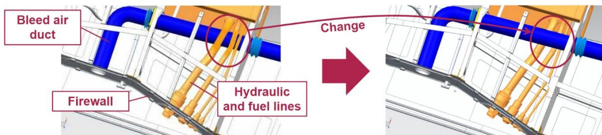
**Figure 5.4.** Use case change scenario: repositioning the hydraulic (6) and fuel lines (7) below the bleed air duct (2).
