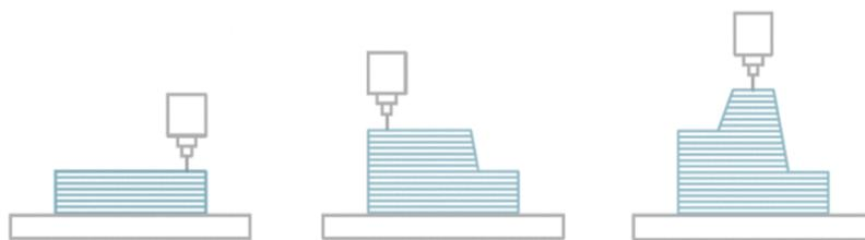
**Figure 1.6.** Additive manufacturing layer by layer principle, adapted from (Lang *et al.*, 2019).
