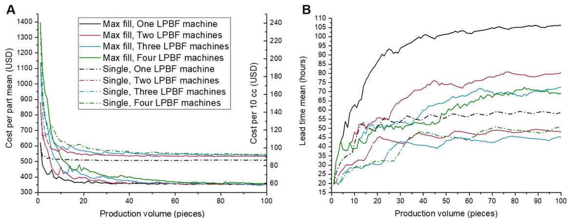
**Figure 4.15.** (a) Cost per part; (b) lead time versus production volume for a single part geometry.
