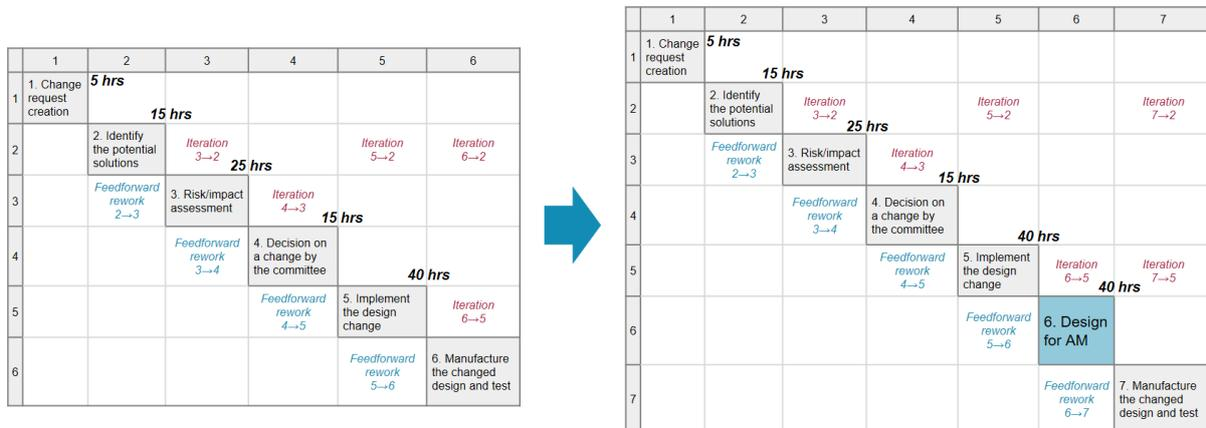
**Figure 5.18.** Adding the design for AM activity into the ICM reference process.
