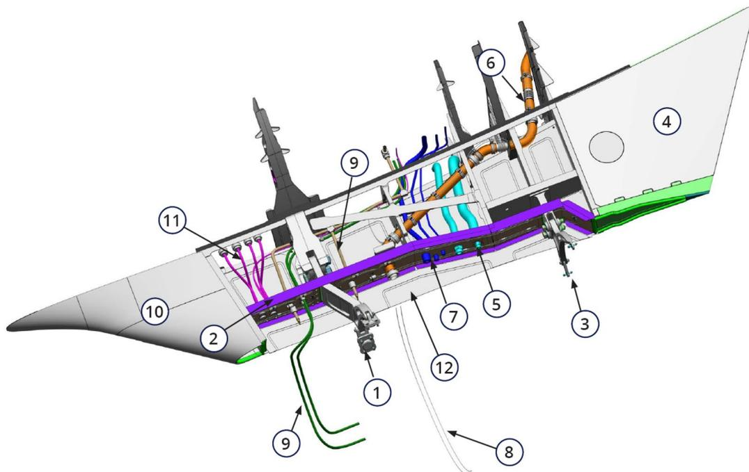
**Figure 5.2.** Pylon installation: (1) Front engine mount, (2) Firewall, (3) Rear engine mount, (4) Trailing edge, (5) Fuel lines, (6) Bleed air duct, (7) Hydraulic lines, (8) Fire detection, (9) Fire extinguishing system (FireX), (10) Leading edge, (11) Electric harnesses, (12) Skin and panels; retrieved from (Eagle Star Aviation, 2015).
