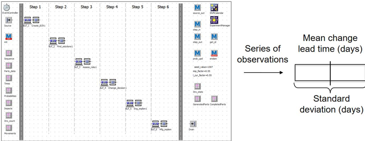
**Figure 4.5.** Overview of the proposed modeling framework; the discrete-event simulation model. The description of the major model objects will be given in Figure 4.10.
