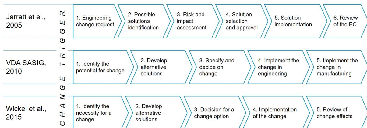
**Figure 2.3.** Comparison of the phases in generic representations of the ECM reference processes (iteration loops are not shown for figure clarity).
