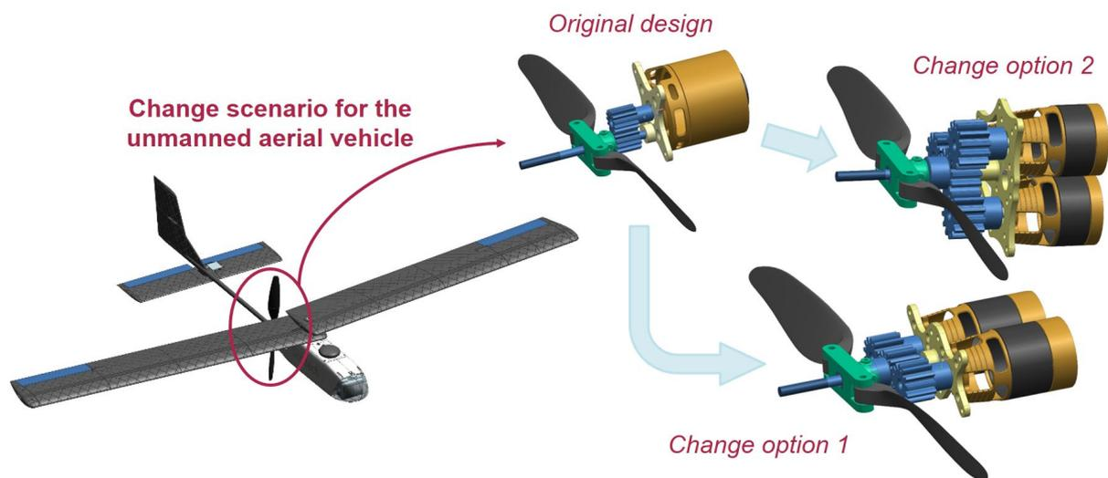
**Figure 3.3.** Change scenario for the unmanned aerial vehicle<sup>27</sup>.
