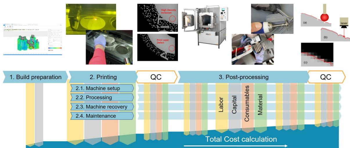
**Figure 4.8.** Accounting the costs of LPBF-based manufacturing workflow<sup>34</sup>.
