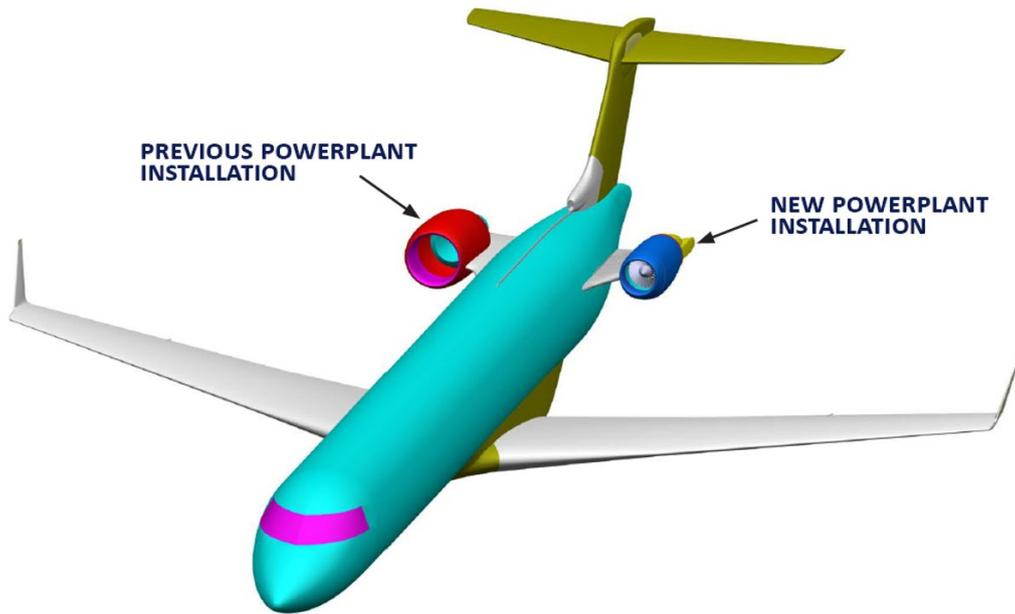
**Figure 5.1.** Installation of P&WC's PW305A turbofan on BA's CRJ700 aircraft; retrieved from (Eagle Star Aviation, 2015).
