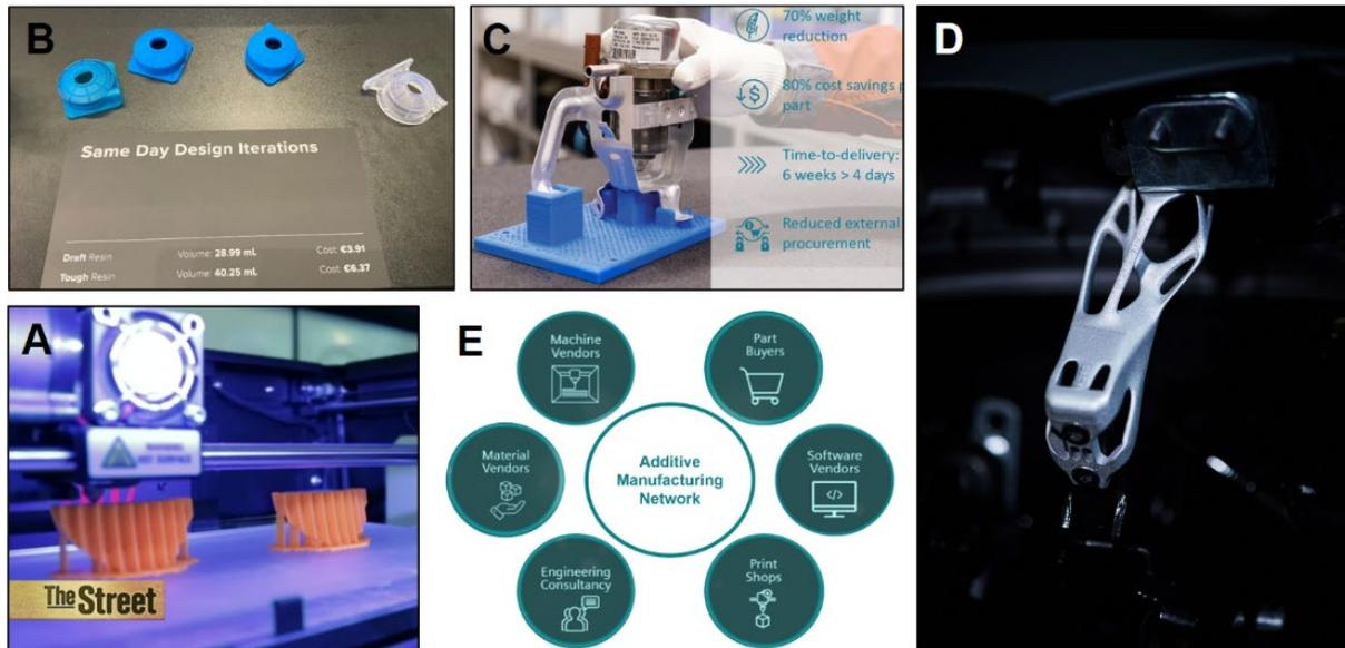
**Figure 1.5.** AM applications: (a) Potato chips prototyping<sup>2</sup>; (b) rapid functional prototyping; (c) 3D printed tooling for supporting the manufacturing process<sup>3</sup>; (d) serial production of end-use components<sup>4</sup>; (e) enabling the AM network<sup>5</sup>.
