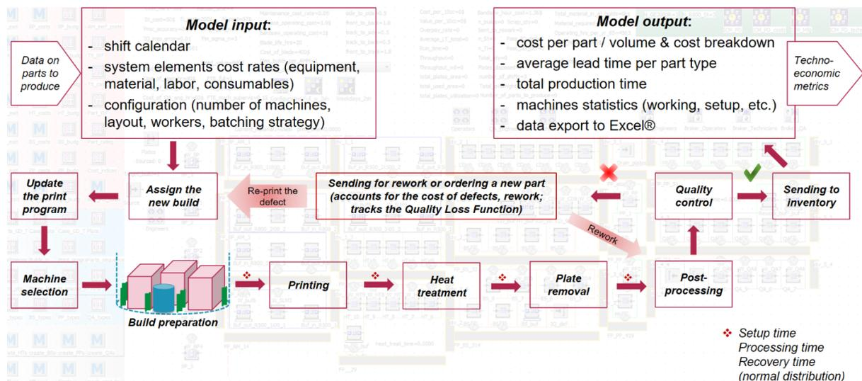
Figure 4.11. Process flow of the manufacturing modeling framework.
