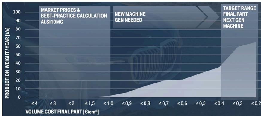
**Figure 1.9.** Production demand (tons per year) versus volume cost (EUR per ccm) feasibility range for laser powder-based fusion AM technology<sup>9</sup>.
