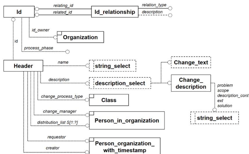
**Figure 4.6.** Excerpt of the Header data model, adapted from (VDA 4965, 2010c).
