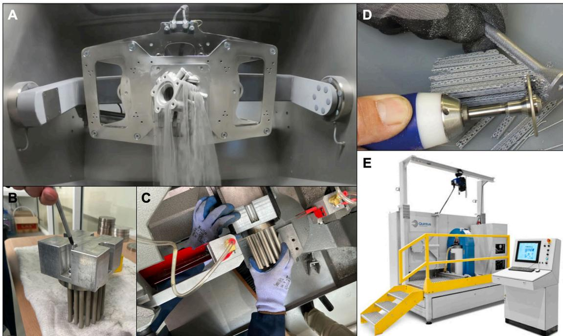
**Figure 2.14.** Post-processing of the printed components: (a) Automated depowdering machining<sup>22</sup>; (b) build plate installation on the bandsaw tooling<sup>23</sup>; (c) build plate separation using a bandsaw (top view)<sup>24</sup>; (d) metal supports manual removal<sup>25</sup>; hot-isostatic pressing (HIP) machine (e)<sup>26</sup>.
