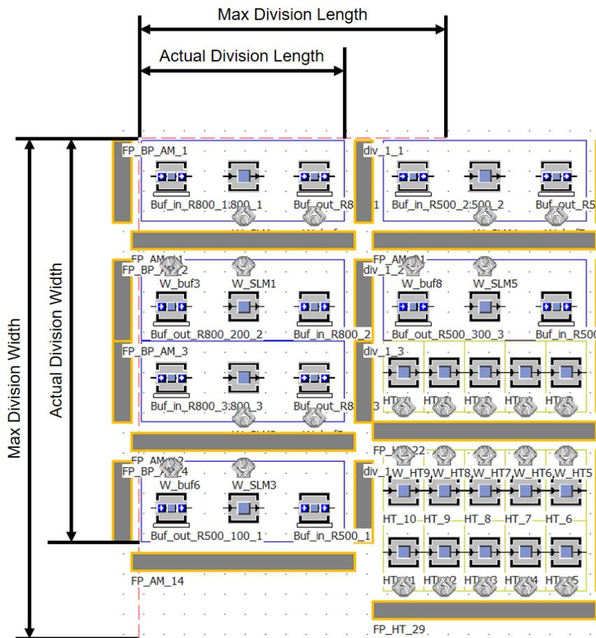
**Figure 4.12.** The maximum and actual length and width of one layout division (the example division demonstrated on the left includes the AM machines and the buffers for builds entrance and exit).
