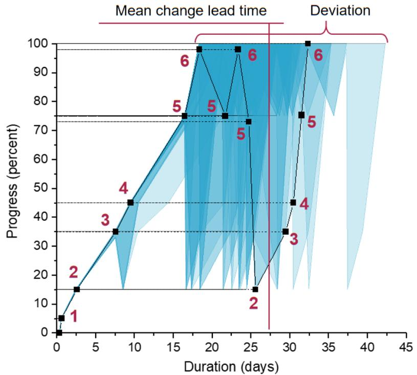
**Figure 5.13.** A simulation-based footprint of the process performance in lead time, illustrating the iterations along the change management progress. The red numbers in the Progress-Duration chart (bottom right) indicate the change progress (Y axis) as completion of the change process step – one of the six steps demonstrated in the modeling framework at the top – after a certain duration (X axis). The description of the major model objects is given in Figure 4.10.
