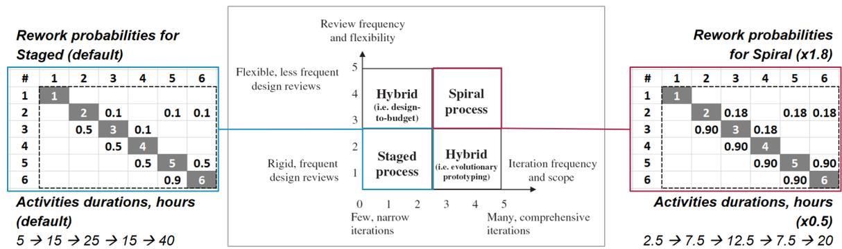
**Figure 5.11.** Comparison of the PD processes based on common review and iteration characteristics; adapted from (Unger and Eppinger, 2011). The matrices on the left and right indicate the rework probabilities between the ICM steps shown in Figure 5.5. The activities’ durations are given for the first five steps; the duration of the manufacturing step 6 is obtained from the simulation results.
