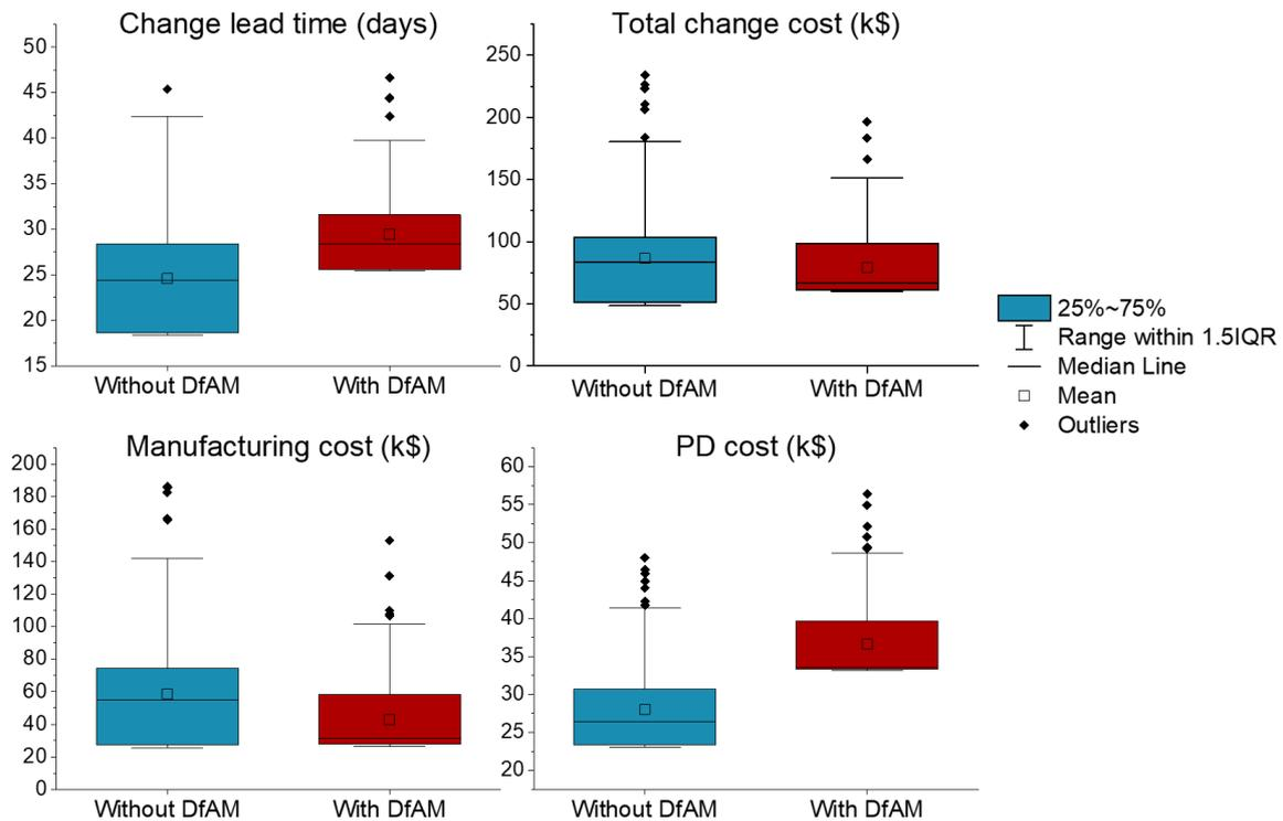
**Figure 5.19.** A time-cost comparison of the ICM processes without and with the design for AM (DfAM) activity to be performed by the AM technologist. IQR stands for interquartile range.
