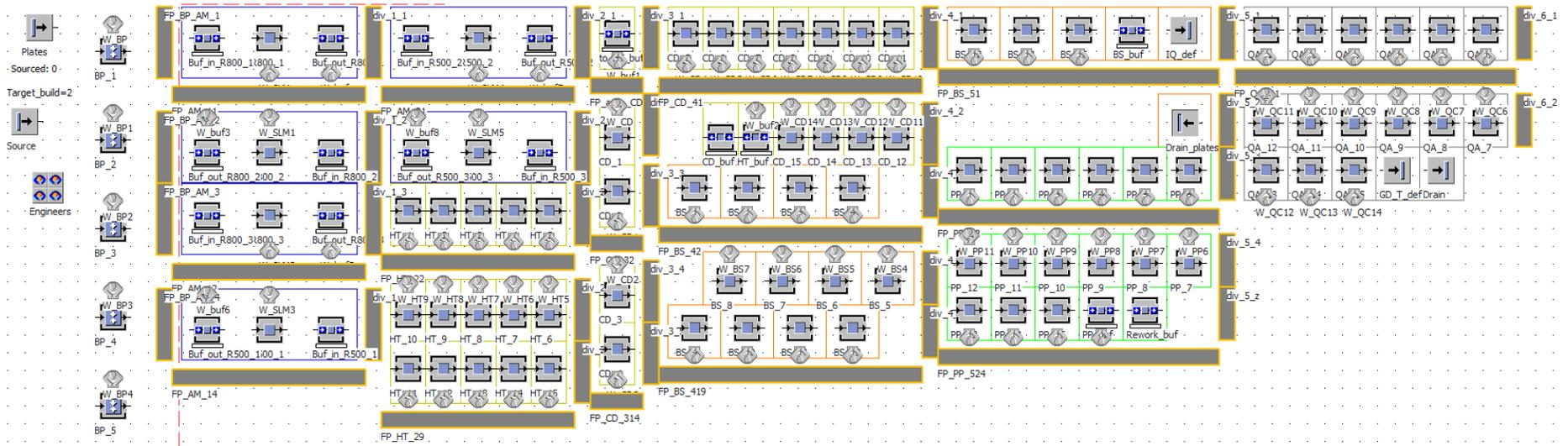
**Figure 5.12.** The manufacturing system configuration for studies ##2-7. The major in-model abbreviations are: *BP* for build preparation; *HT* for heat treatment; *CD* for cooldown; *BS* for build plate separation; *PP* for post-processing and manual supports removal in particular; *QA* for quality control and assurance; *FP* for foot path. The description of the major model objects is given in Figure 4.10.
