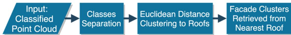
Figure 3-12. Instance segmentation workflow for buildings.
