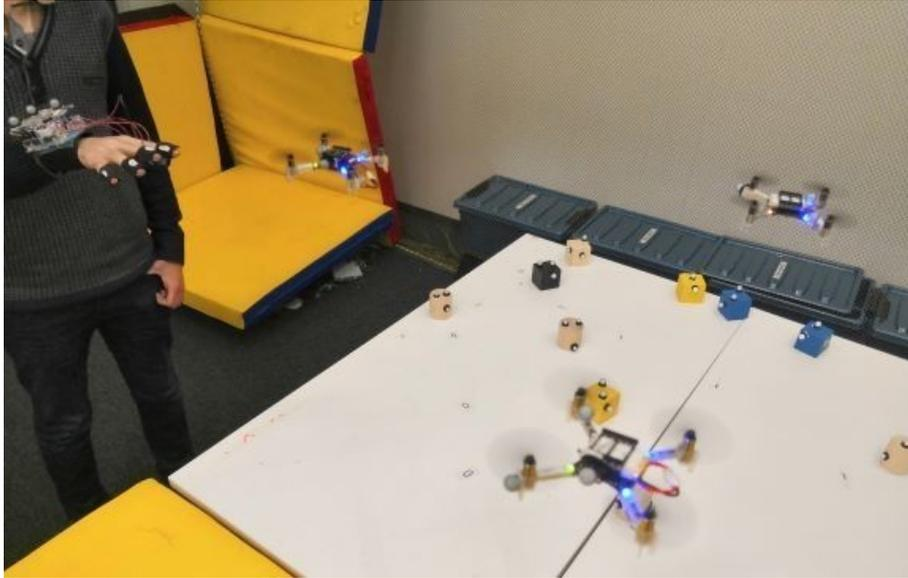
Figure 6-4: Human operator manipulates the formation of three quadrotors.
