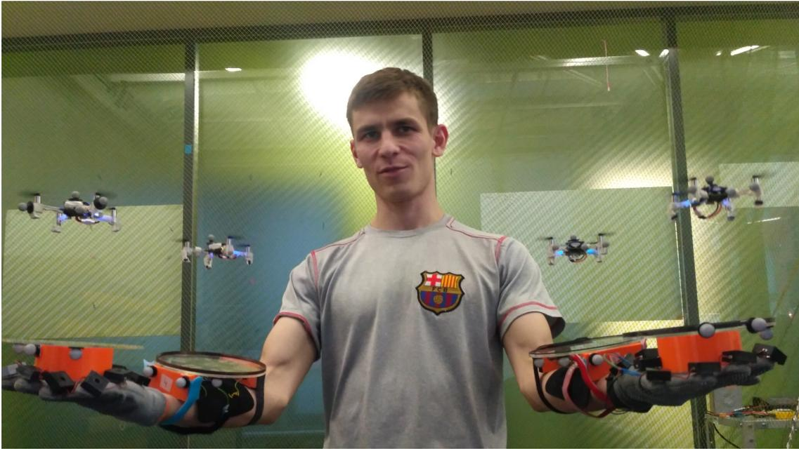
Figure 7-1: Deployment of four drones with wearable tactile display SwarmCloak.
