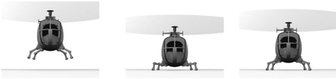
Figure 2-11: Robotic landing gear by [Kiefer et al. \[2016\]](#).
