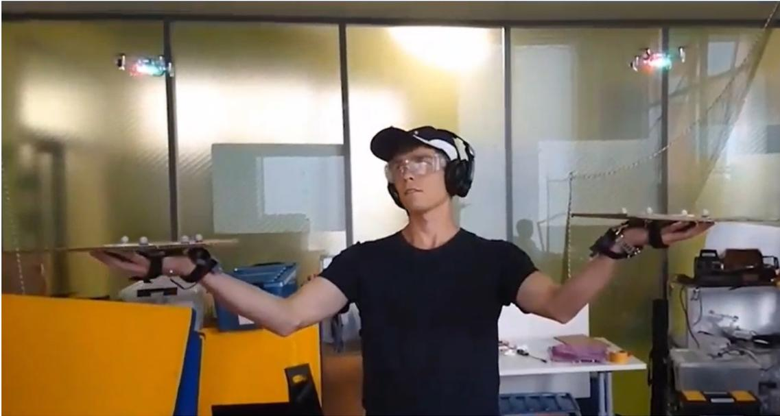
Figure 7-6: Landing of two drones using SwarmCloak (visual + tactile feedback condition).
