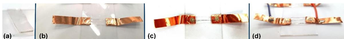
**Figure 15.** PDMS encapsulation process of the SWCNTs fiber. (a) A thin layer of PDMS is prepared. (b) Copper self-adhere tape is attached to the PDMS. (c) A SWCNT fiber is glued with silver conductive paste. (d) It is covered with liquid PDMS, then cured. In addition, wires are soldered to the copper tape.
