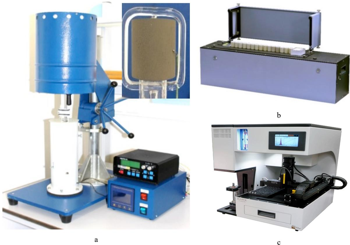
**Figure 7.** Main (a) and auxiliary equipment (b, c) used in the study; a - Quartz dilatometer with an installed core sample, b - Thermal Conductivity Scanner, c - HAWK pyrolysis instrument.
