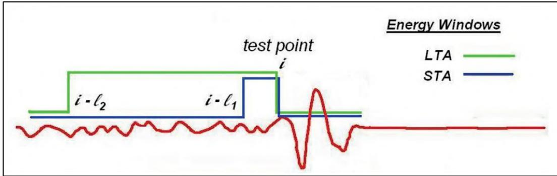
Figure 3-2: Single-station implementation of the STA/LTA approach. Red is signal, green and blue are respectively LTA and STA energy windows. LTA should be around 5 to 10 times the length of STA, while STA should be about 3 to 5 times the dominant period [Akram and Eaton, 2016]
