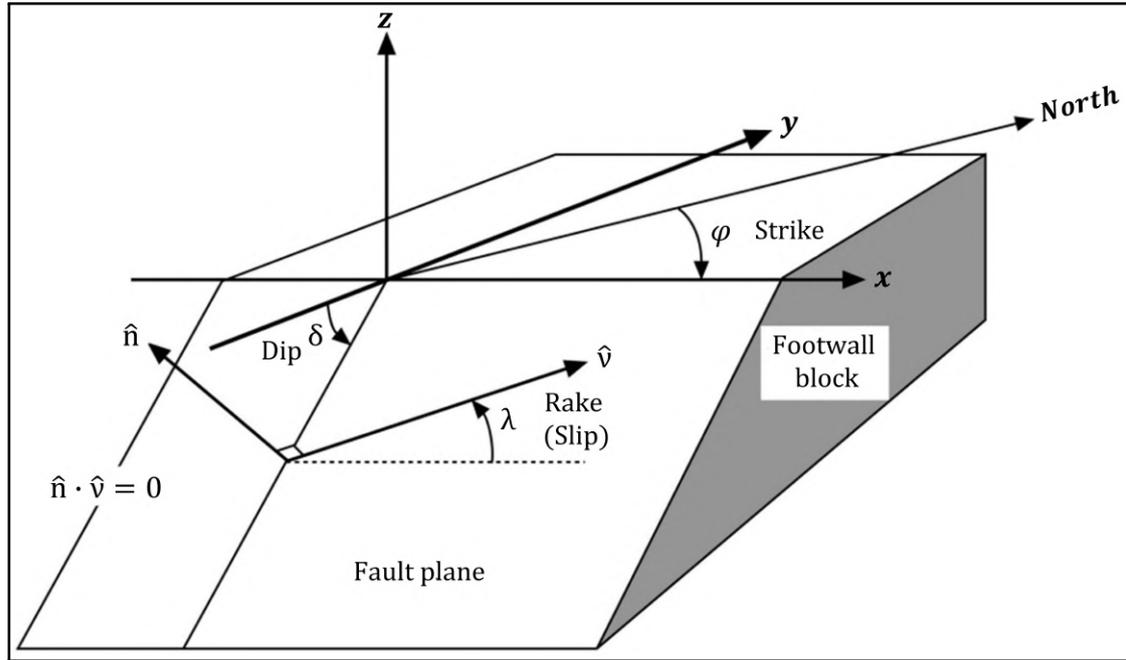
Figure 3-6: Schematic representation of fault geometry commonly used in seismic studies. The fault plane angles of strike, dip and rake are defined as shown on the diagram. Modified after [Kanamori and Cipar \[1974\]](#)
