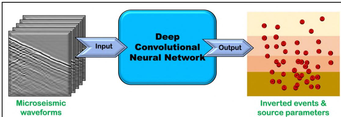
Figure 3-9: Schematic representation of inversion of microseismic events and source parameters from raw microseismic data using convolutional neural network. Adopted from [Wamriew et al., 2021b]
