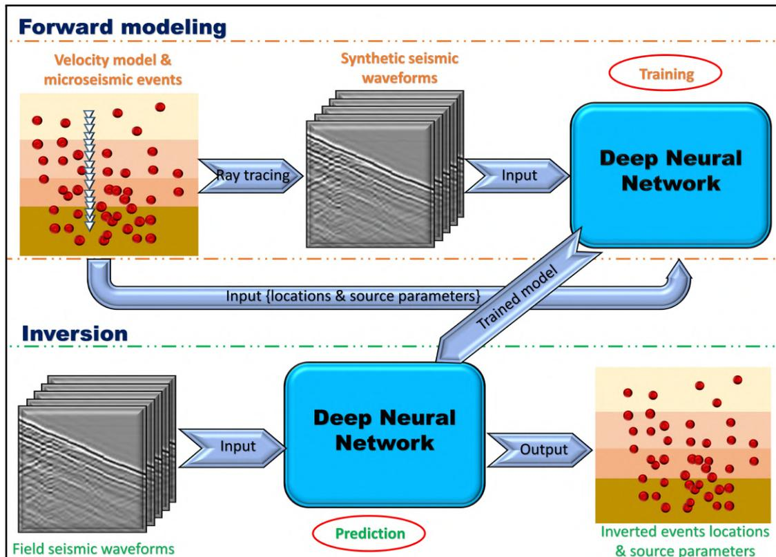
Figure 3-10: Flow chart depicting CNN-based microseismic events location and velocity model update network. The processes of training and prediction are highlighted and linked with the arrows. Red dots represent microseismic events. Modified after [Wamriew et al., 2021b]
