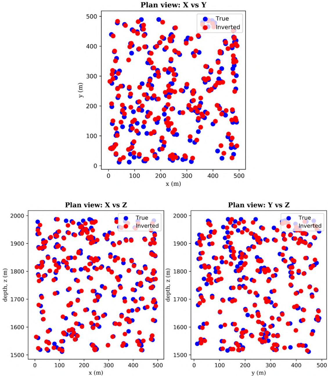
Figure 4-7: 2-D plan view plots of the ground-truth and inverted locations of the microseismic events. Here, the blue dots show the locations of the ground-truth events while the red dots are the inverted (predicted) locations by the neural network model. Adopted from [Wamriew et al., 2022a]
