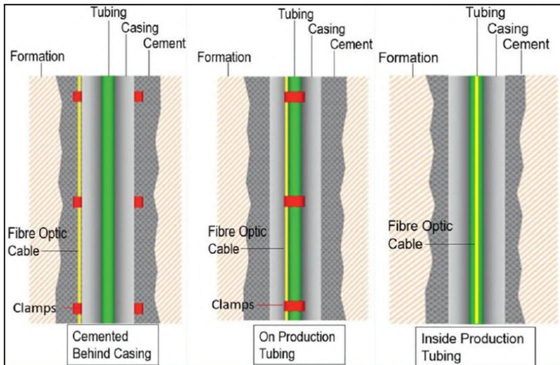
Figure 2-4: Fibre optic cable coupling options in a borehole survey. Modified from Fenta et al. [2021]
