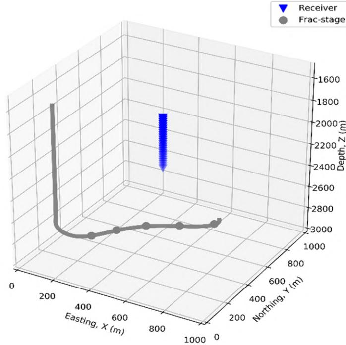
(a) Borehole - Receiver Set-up
