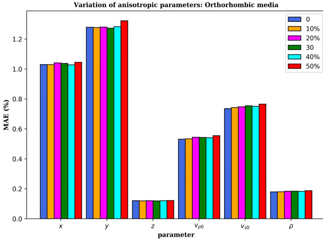
Figure 4-11: Comparison of location and velocity model parameters for orthorhombic medium inverted by the CNN trained on VTI data. Different colors represent various levels of perturbations of anisotropic parameters as indicated on the legend of the bar chart. Source: [Wamriew et al., 2022a]
