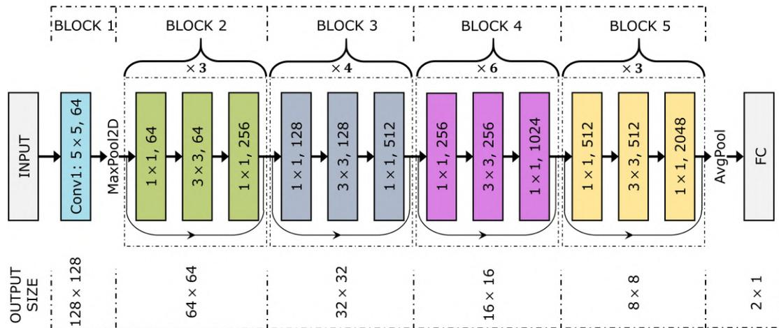
Figure 4-29: Architecture of the 50-layer deep neural network used in this study. Abbreviations: Conv—convolutional layer, MaxPool2D—two-dimensional maximum pooling layer, Avg-Pool—global average pooling layer, FC—fully connected layer. Source: [Wamriew et al., 2022b].
