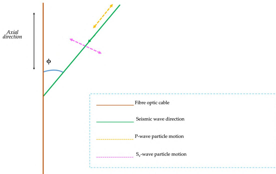
Figure 4-23: Directional sensitivity of DAS to body waves. DAS is most sensitive to the component of particle motion that is in the axial direction. Source: [Wamriew et al., 2021b].
