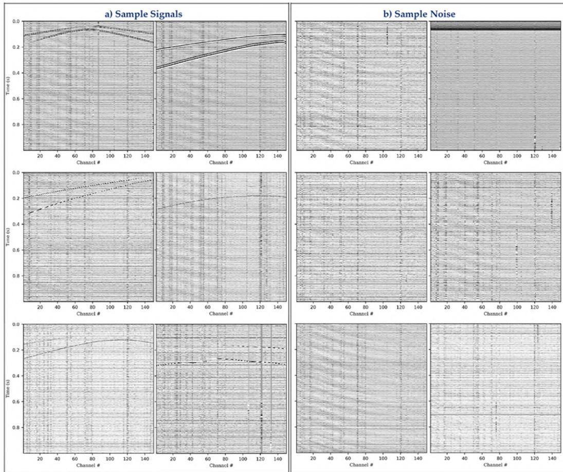
Figure 4-15: Sample synthetic data **(a)** DAS microseismic events contaminated with ambient noise from field data **(b)** sample DAS ambient noise from extracted from field data. Source: [Wamriew et al., 2021b].
