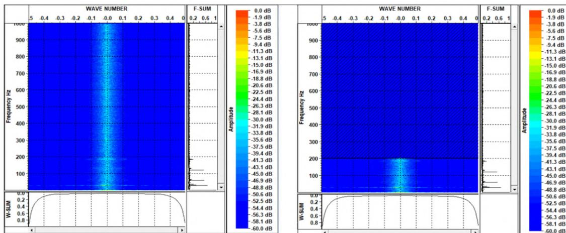
Figure 4-27: Original F-k area on the left. The right picture shows the horizontal box rejection zone. Source: [Wamriew et al., 2022b].
