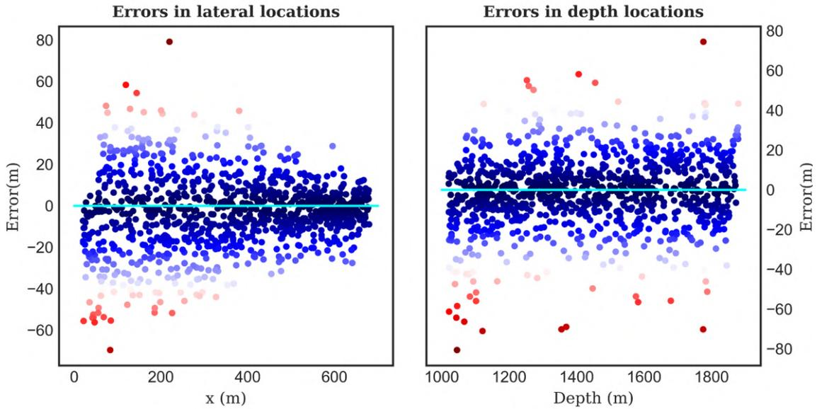
Figure 4-34: Errors in the locations of the microseismic events. Dark to medium blue are within two standard deviations from the mean, while red is more than two standard deviations from the mean. The events underlying the cyan line had no errors. Source: [Wamriew et al., 2022b].
