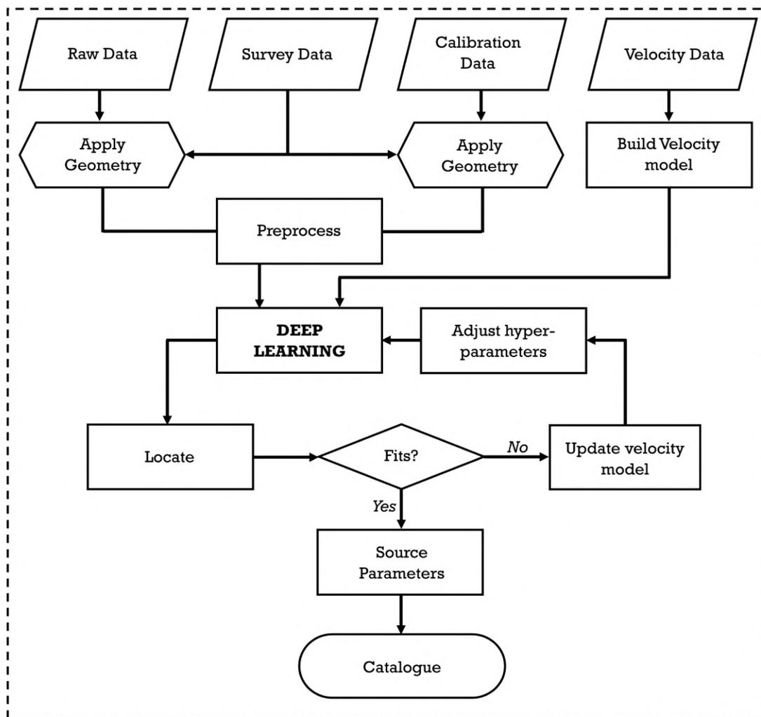
Figure 4-2: Deep learning based algorithm for processing borehole passive seismic data.
