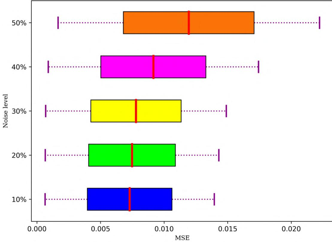
Figure 4-10: Box and whisker plot for the performance of the CNN on data contaminated with noise to the given percentages on the vertical axis. The red line in the middle of the plots represent the median while the left and right edges of the box are the lower- and upper-quartiles respectively while the left and right whiskers are the minimum and maximum mean squared errors respectively. Source: [Wamriew et al., 2022a]
