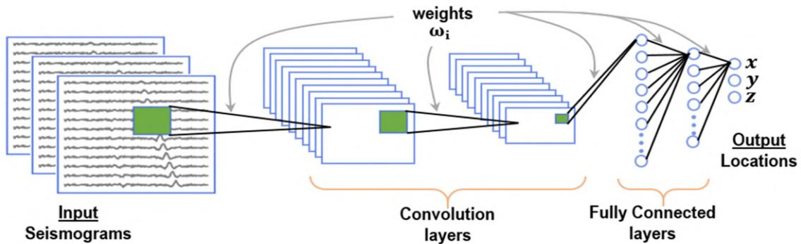
Figure 4-42: Convolutional neural network architecture. The network takes as input seismograms and outputs the locations  $(x, y, z)$  of the microseismic events. The network is elaborately discussed in subsection 4.5.5.1. Source: [Wamriew et al., 2020].
