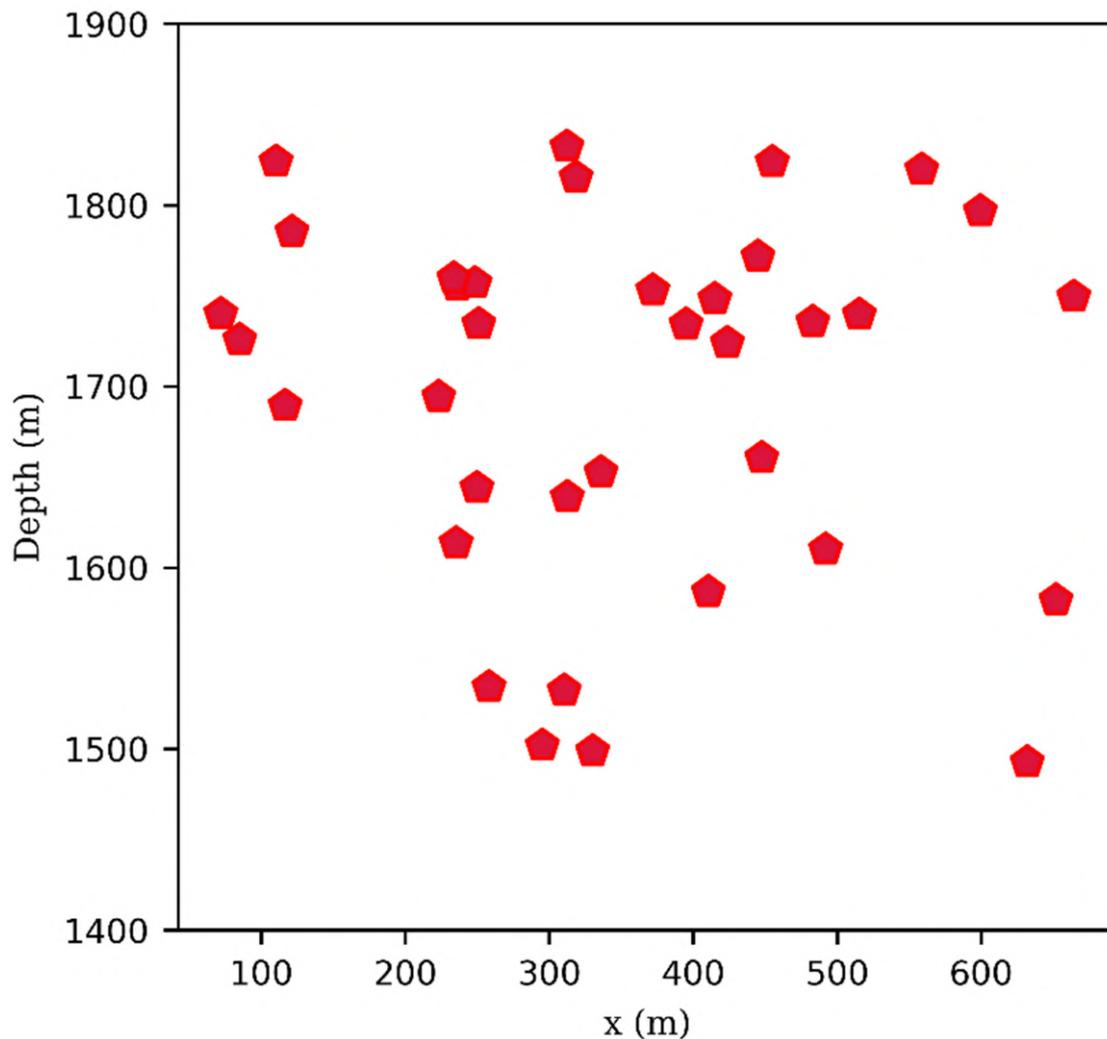
Figure 4-37: 2-D section view projection of the inverted locations of the microseismic events from the FORGE data. Source: [Wamriew et al., 2022b].
