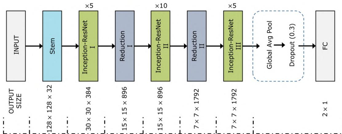
Figure 4-30: Architecture of the inception-ResNet. Abbreviations: FC—fully connected layer, Global Avg Pool—global average pooling. Source: [Wamriew et al., 2022b].
