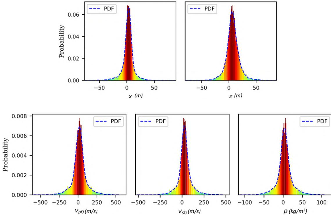
Figure 4-18: Residual diagnostic histograms for trained CNN model. The blue envelope represents the probability density function. The velocity model parameters of each histogram is indicated at the bottom center of each plot. Adopted from [Wamriew et al., 2021b].
