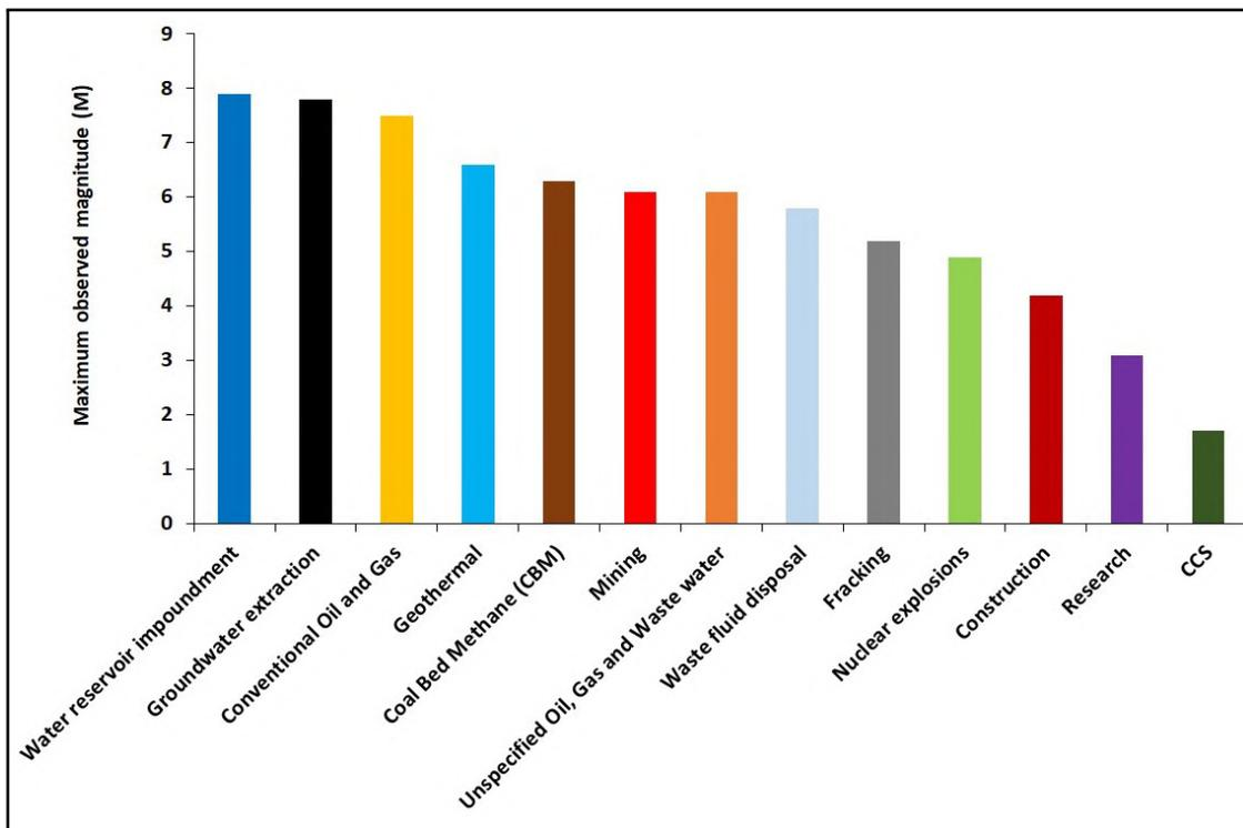
Figure 2-2: Maximum observed magnitudes of induced seismicity by different anthropogenic sources. Source: [Foulger et al., 2018]
