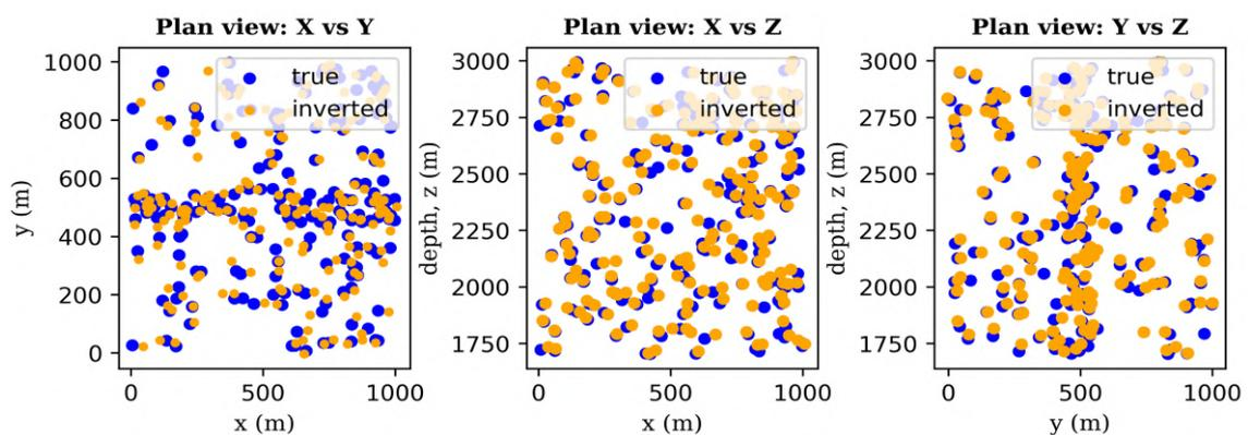
Figure 4-44: 2D plan-view plots showing the locations of the inverted (in orange) versus the ground-truth (in blue) microseismic events. The projections are indicated on the title of each plot. For purposes of clarity, only 200 events are shown on the plots. Source: [Wamriew et al., 2020].
