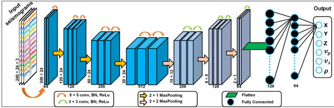
Figure 4-6: Architecture of the neural network used to locate the microseismic events and perform velocity model inversion. The blue and grey cuboids represent multiple channel feature maps with the number of channels indicated beneath the cuboids. The input dimensions of each layer is given along the lower left edge of the cuboids. The size and operations denoted by each kind of arrow are defined in the boxes beneath the network. Source: [Wamriew et al., 2022a]
