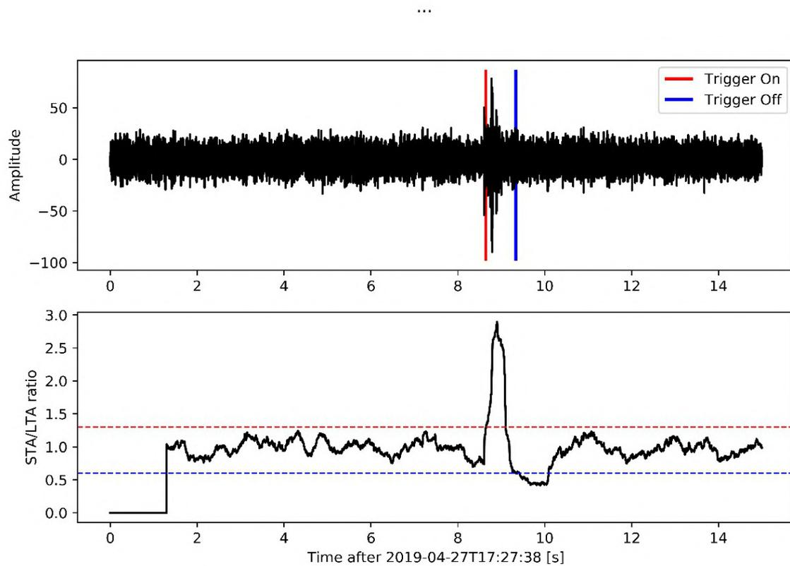
Figure 4-38: An example of the STA/LTA implementation for the detection of microseismic events. **(Top)** Amplitude spectrum of the waveform. **(Bottom)** STA:LTA ratio plot. An event is declared when the STA:LTA ratio exceeds 1.3. Red and Blue dotted lines indicate the thresholds above and below which the trigger is on and off respectively. Source: [Wamriew et al., 2022b].
