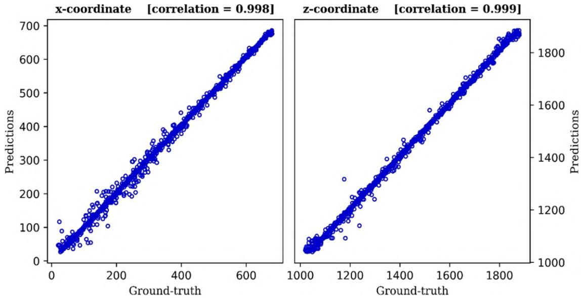
Figure 4-33: Correlation plot of the predicted versus ground-truth microseismic events after the exclusion of noise samples from the test dataset. Source: [Wamriew et al., 2022b].
