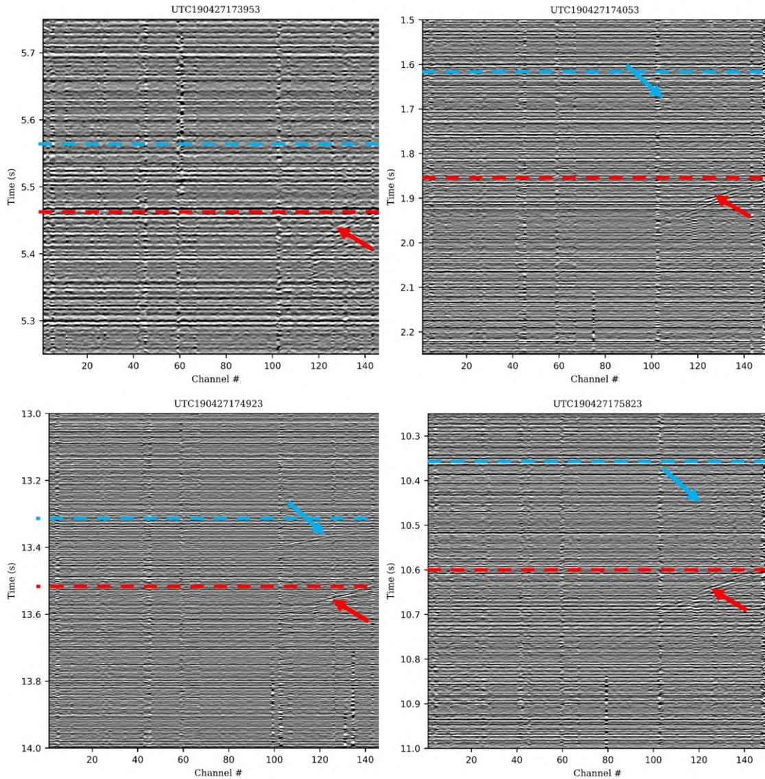
Figure 4-36: Sample of the low magnitude events detected by the CNN but were not in the events catalog. The red lines represent the S-wave arrival times while the cyan shows the estimated P-wave arrivals. Similarly, the cyan and red arrows show the P- and S-waves respectively. Source: [Wamriew et al., 2022b].
