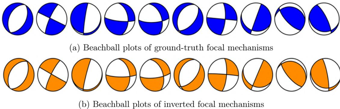
Figure 4-45: Sample fault plane solutions of 10 randomly selected events from the test dataset. **(a)** Beachball plots of ground-truth focal mechanisms generated by forward modelling. **(b)** Beachball plots of the inverted focal mechanisms obtained from the neural network. Source: [Wamriew et al., 2020].
