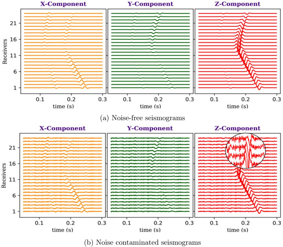
Figure 4-41: **(a)** Sample 3-C synthetic seismograms of an event recorded by the receivers in the borehole. **(b)** Noise contaminated seismogram of the same event. A zoom has been made on the Z-component to give a clear picture of the noise level in the data. The waveforms are sampled at an interval of 1 ms for a duration of 0.6s and are plotted for a window of 0.05 – 0.3 seconds. Source: [Wamriew et al., 2020].
