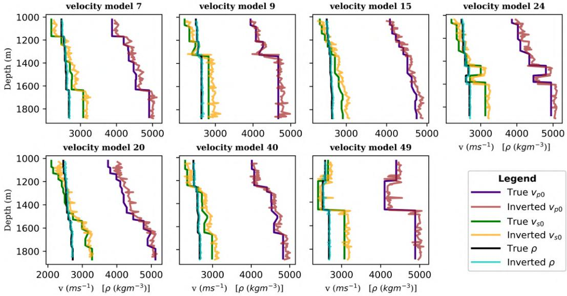
Figure 4-20: 1-D velocity model profiles for prediction versus ground-truth values. Blue, green and black represent ground-truth  $v_{p0}$ ,  $v_{s0}$  and  $\rho$  values respectively, while red, orange and cyan the corresponding inverted values. Source: [Wamriew et al., 2021b].
