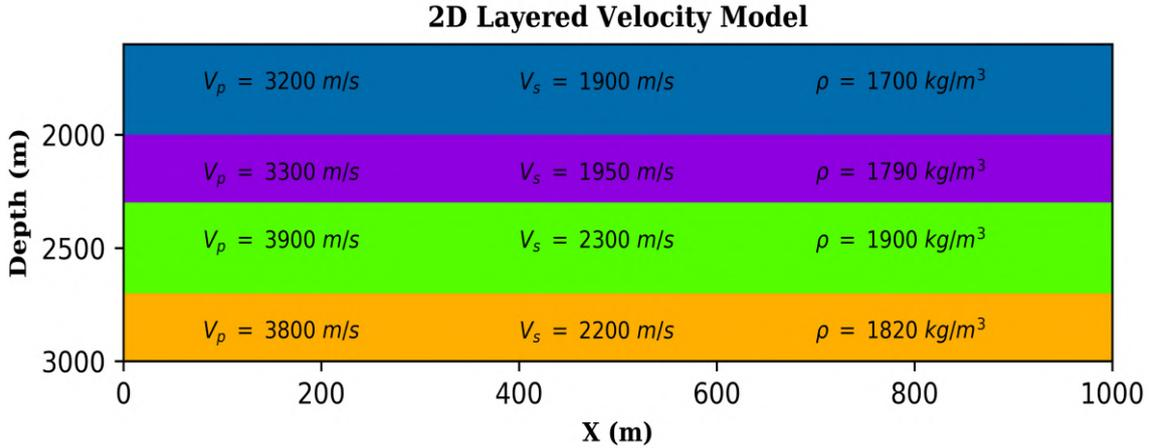
Figure 4-39: Velocity model used in the forward modeling to produce synthetic seismograms by ray tracing. Source: [Wamriew et al., 2020].
