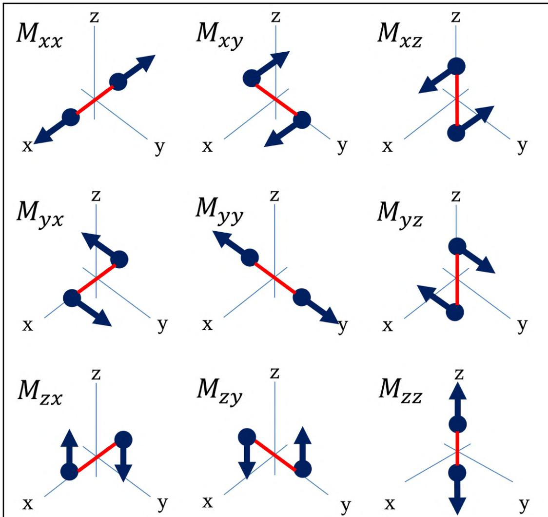
Figure 3-4: Schematic representation of the nine generalized force couples that make up the seismic moment tensor in Cartesian coordinate system. Adopted from Aki and Richards [2002]
