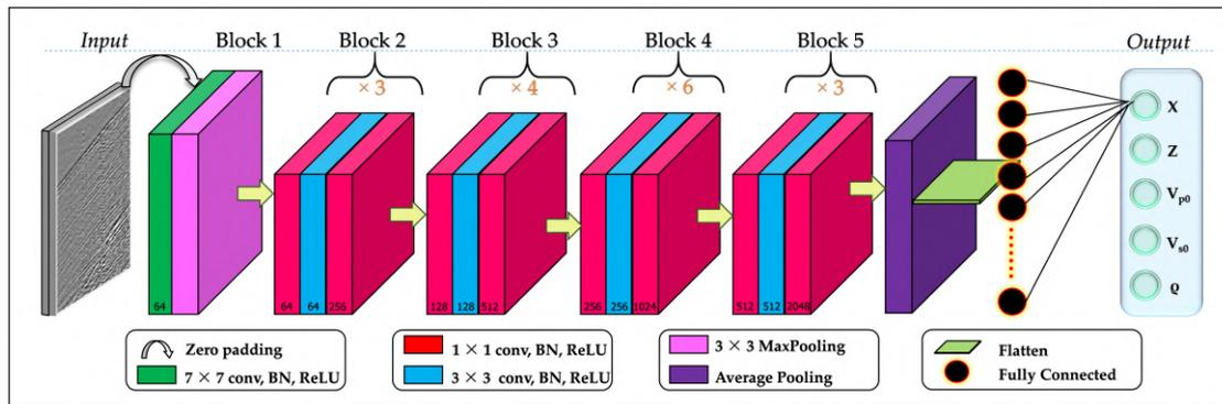
Figure 4-16: Deep convolutional neural network architecture used in the study. Green, blue and red cuboids represent multi-channel feature maps with number of channels shown at the bottom of the cuboids. The input dimensions of each layer is given in Table 4.3. Source: [Wamriew et al., 2021b].
