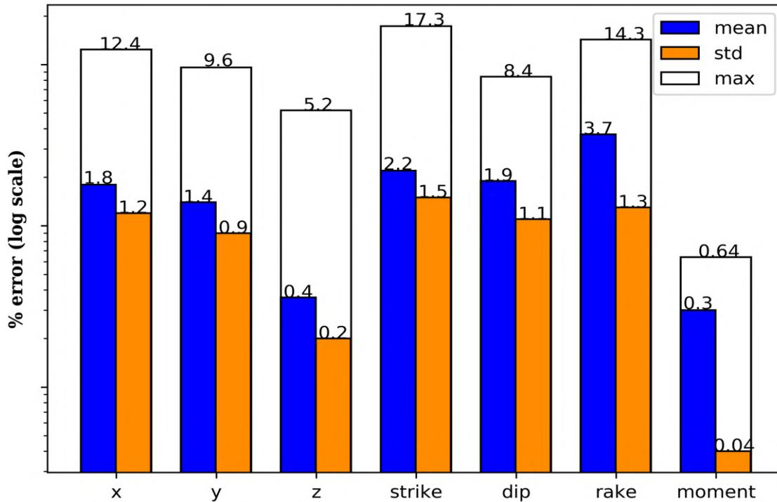
Figure 4-46: Error plot for the seven location and source parameters inverted by deep learning. The vertical scale is logarithmic. Source: [Wamriew et al., 2020].
