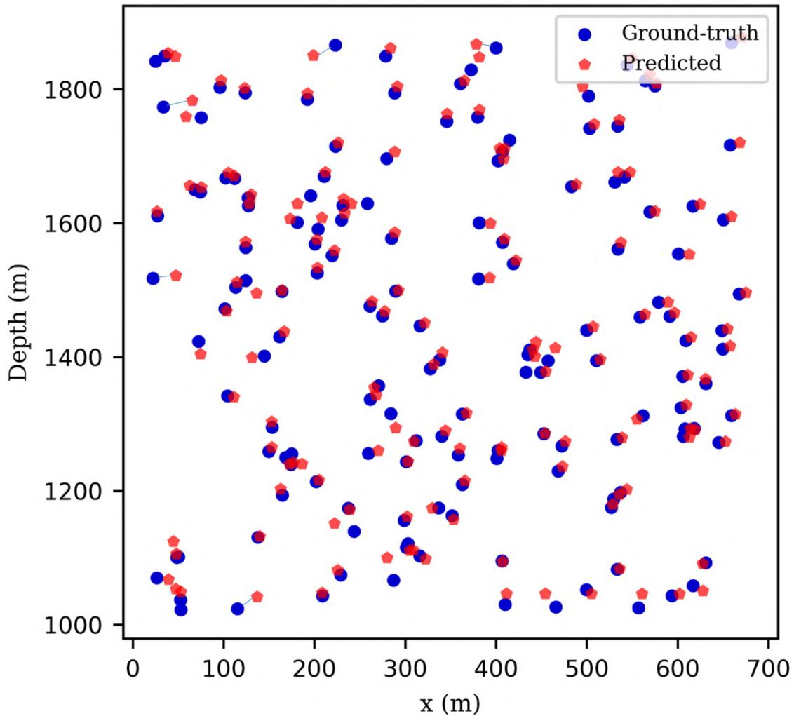
Figure 4-35: 2-D section view project of the predicted versus ground-truth microseismic events. Blue dots represent the ground-truth locations while the red pentagons represent the inverted events. Source: [Wamriew et al., 2022b].
