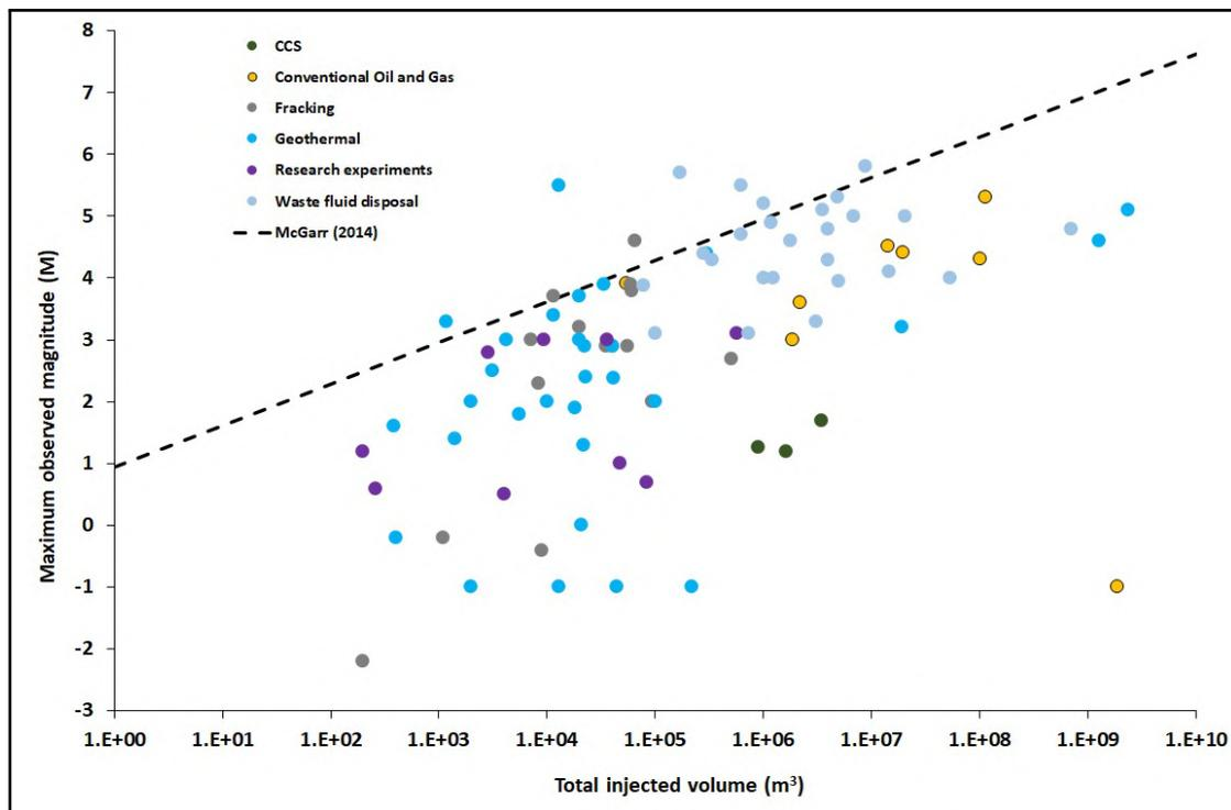
Figure 2-3: Maximum observed magnitudes versus total volume of injected fluids for sixty-nine induced seismic events. The dotted line indicates the upper-limit of the magnitudes based on theoretical consideration by McGarr [2014]. This theoretical consideration holds for many cases, although there are certain outliers which it does not account for. Source: [Foulger et al., 2018]
