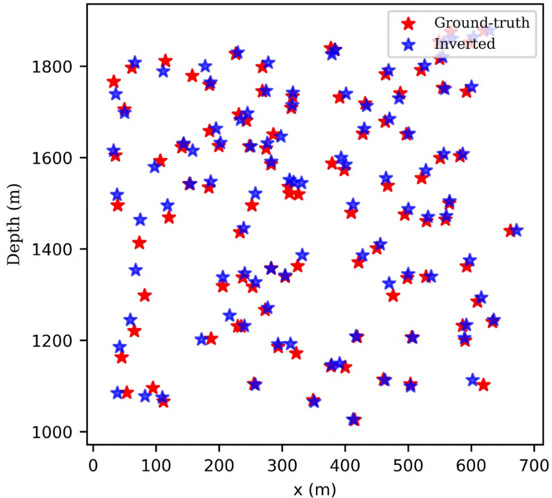
Figure 4-19: 2-D plan view projection of the inverted DAS microseismic depth locations (blue stars) versus ground-truth locations (red stars). Only 100 events from one velocity model are displayed. Source: [Wamriew et al., 2021b].
