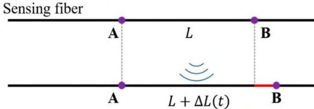
Figure 3-8: The sensing principle of the fiber-optic distributed acoustic sensing system. Source: Sun et al. [2022]
