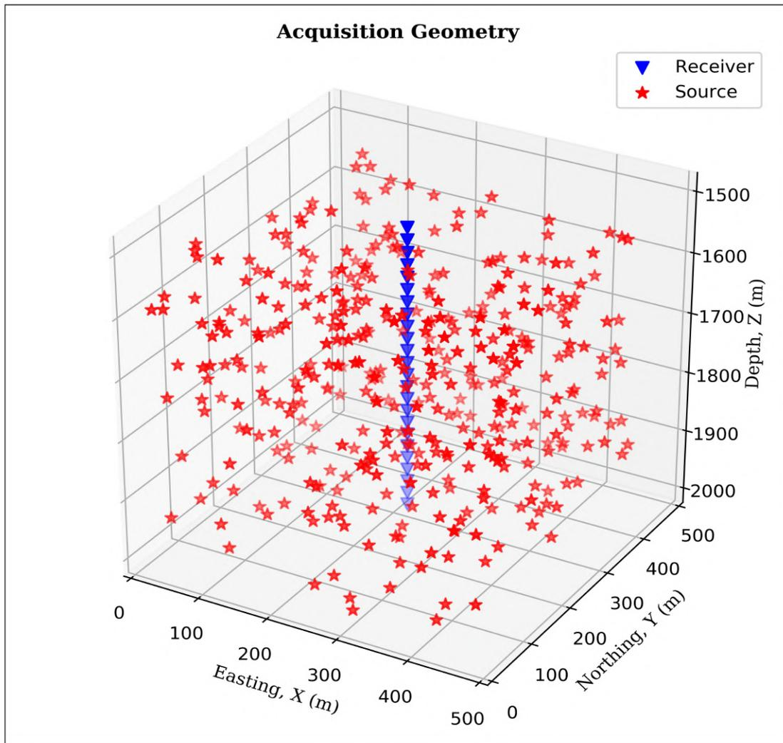
Figure 4-4: Acquisition geometry comprising of 24 3-C receivers in a downhole array (blue triangles) at intervals of 20 m, and 200 microseismic events (red stars) randomly distributed within the cube of sides 500m. The events had varying moment magnitudes in the range  $-2.0 \leq M_w \leq 0$ . Source: [Wamriew et al., 2022a]
