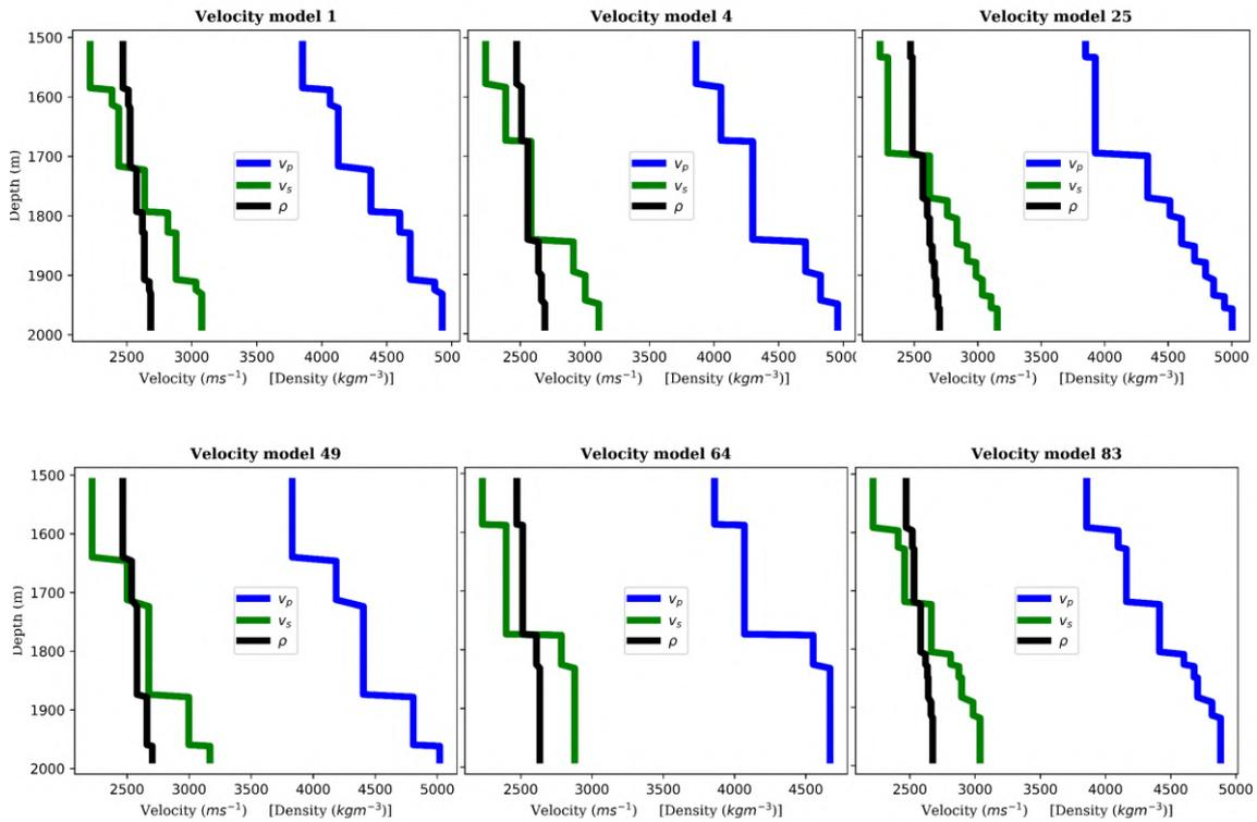
Figure 4-3: Sample velocity parameters for various models considered. The number of layers vary between 4 and 11. Blue and green curves represent P- and S-wave velocities in each layer while black represents the layer density.
