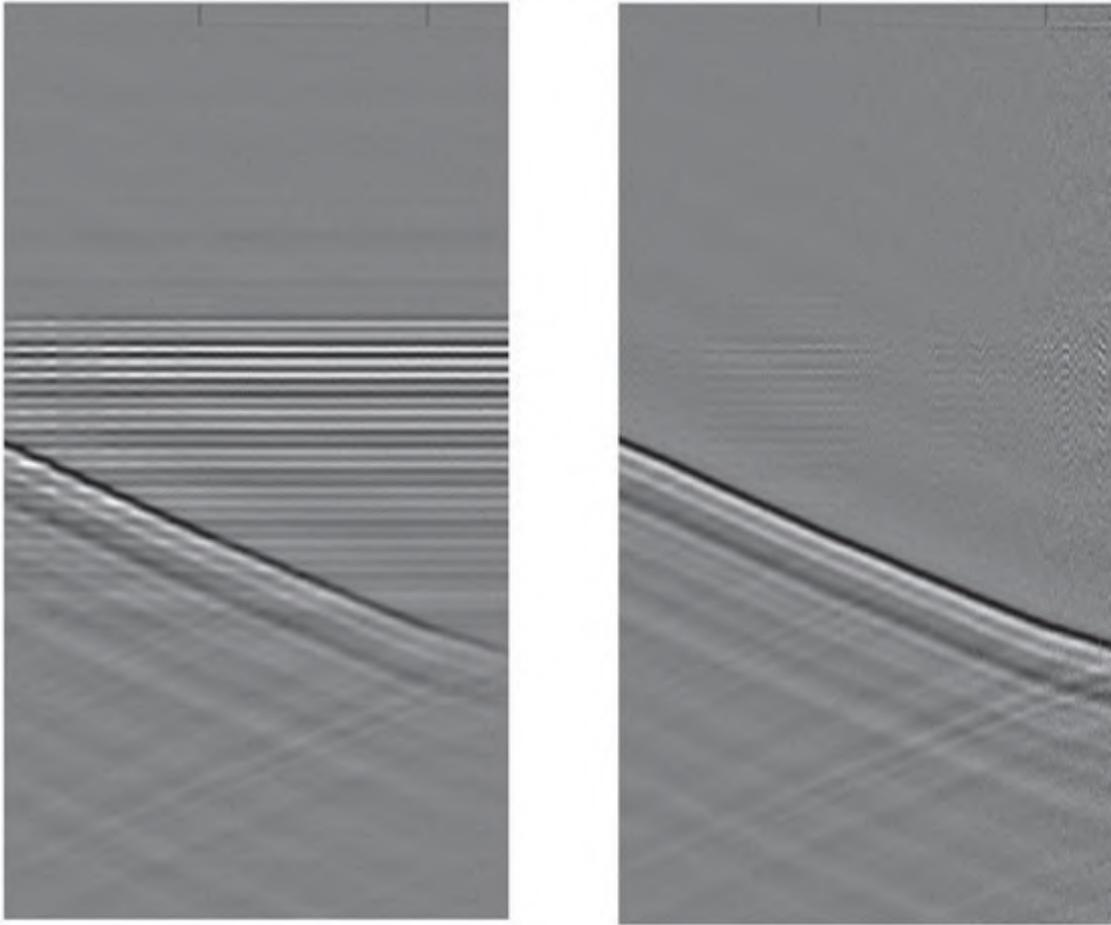
Figure 3-11: (Left) DAS record of strain rate showing common-mode noise; (right) same record after removal of the common-mode noise. Source: [Li et al. \[2022b\]](#)
