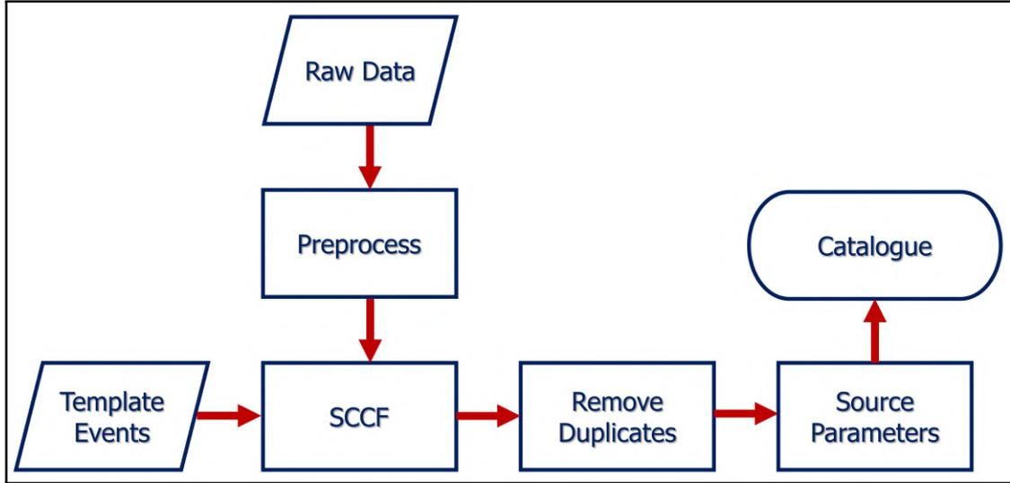
Figure 3-3: Event detection workflow using the matched filtering template matching approach for downhole microseismic data.
