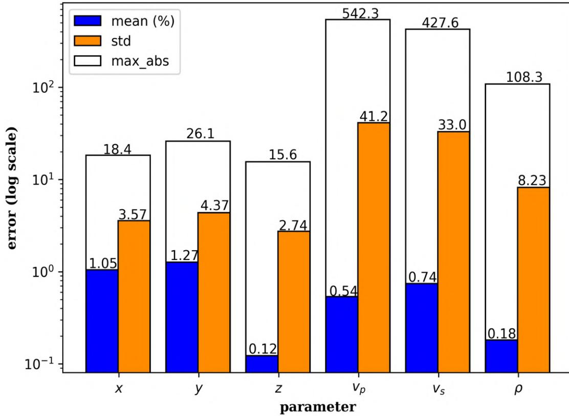
Figure 4-9: Percentage error bar graph for the location and velocity model parameters inverted by deep learning. The vertical scale is logarithmic while the parameters are shown on the horizontal axis with their respective values at the top of each bar. Blue, orange and white bars represent the mean, standard deviation and maximum errors respectively. Source: [Wamriew et al., 2022a]
