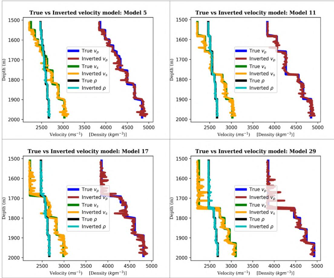
Figure 4-8: Sample inverted and ground-truth velocity model parameters: Blue, Green and Black staircases represent ground-truth P- and S-wave velocities and layer density respectively while brown, yellow and cyan their corresponding predicted values by the deep neural network. The number of layers vary in each plot between 4 and 12. Adopted from [Wamriew et al., 2022a]
