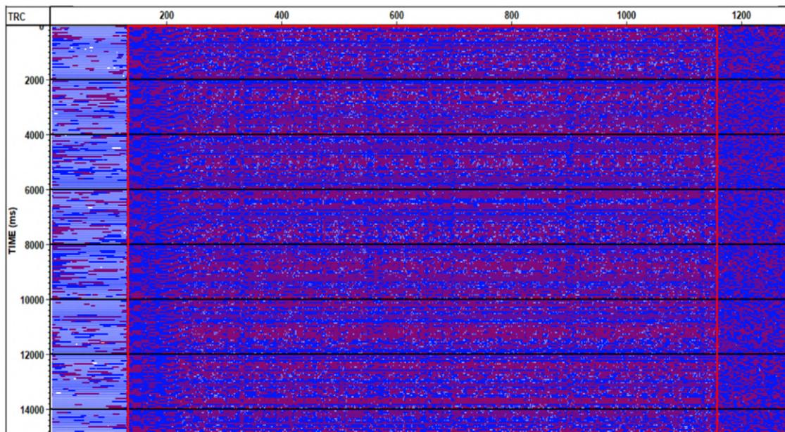
Figure 4-24: A fragment of the DAS record before processing. The area of interest highlighted in red is due to the technical peculiarities of the data collection. Source: [Wamriew et al., 2022b].
