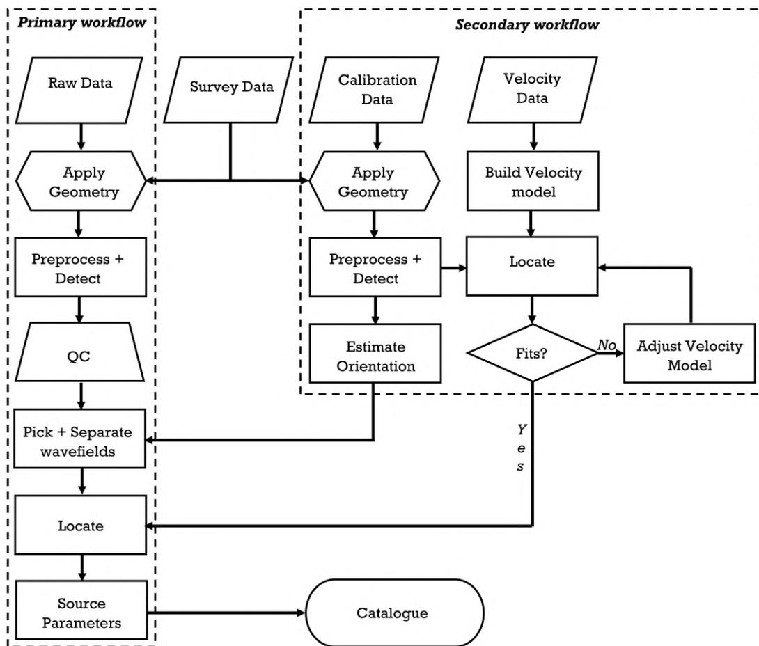
Figure 4-1: Conventional algorithm for processing borehole passive seismic data. Modified from [Eaton, 2018].
