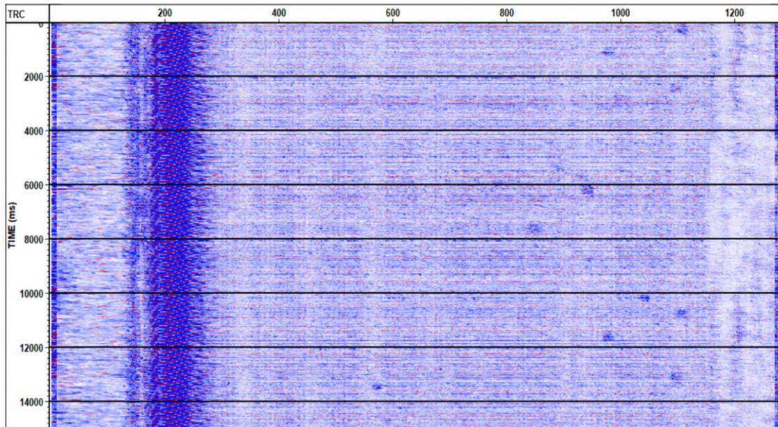
Figure 4-28: Result of the DAS data processing using the presented workflow. Source: [Wamriew et al., 2022b].
