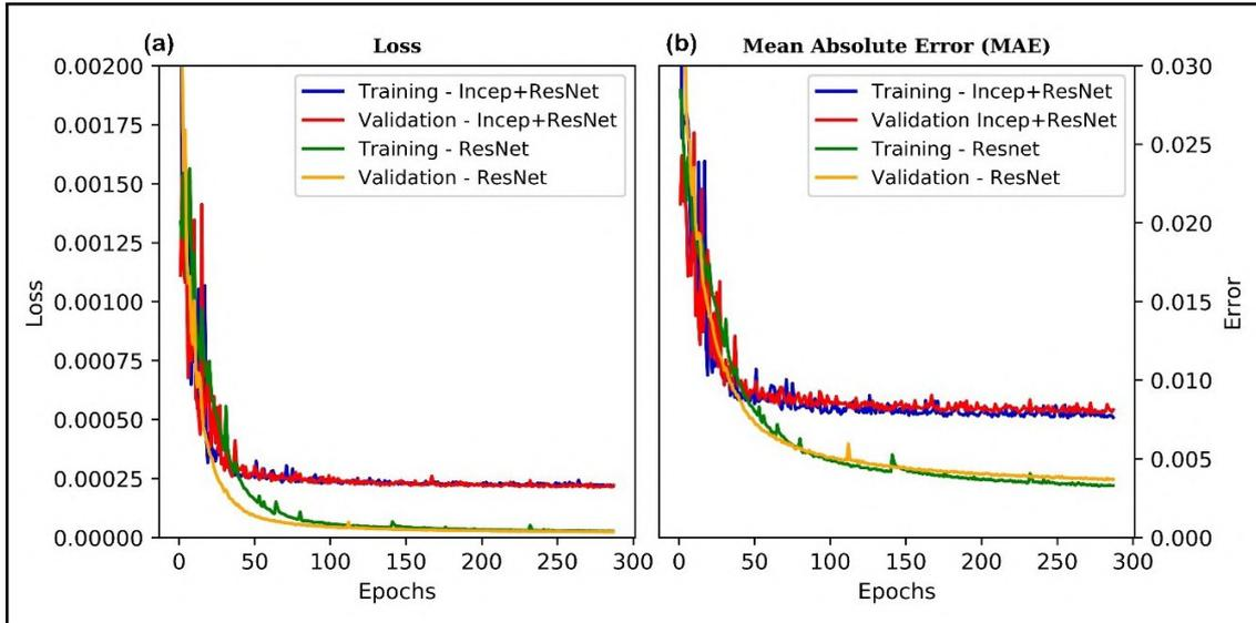
Figure 4-31: Training and validation metrics for both the ResNet and inception-ResNet models: (a) training and validation loss; (b) training and validation mean absolute errors. Source: [Wamriew et al., 2022b].
