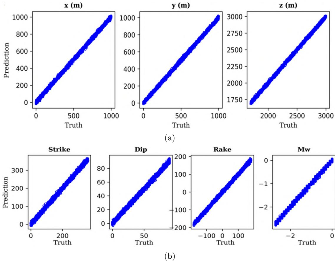
Figure 4-43: (a) Scatter plots of each coordinate location of the microseismic events predicted by the CNN versus its ground-truth value from the test set of synthetic events. (b) Scatter plots of the predicted versus the actual source parameters (strike, dip, rake and moment magnitude). A positive correlation between the predicted and true values is evident on each of the seven plots. Source: [Wamriew et al., 2020].
