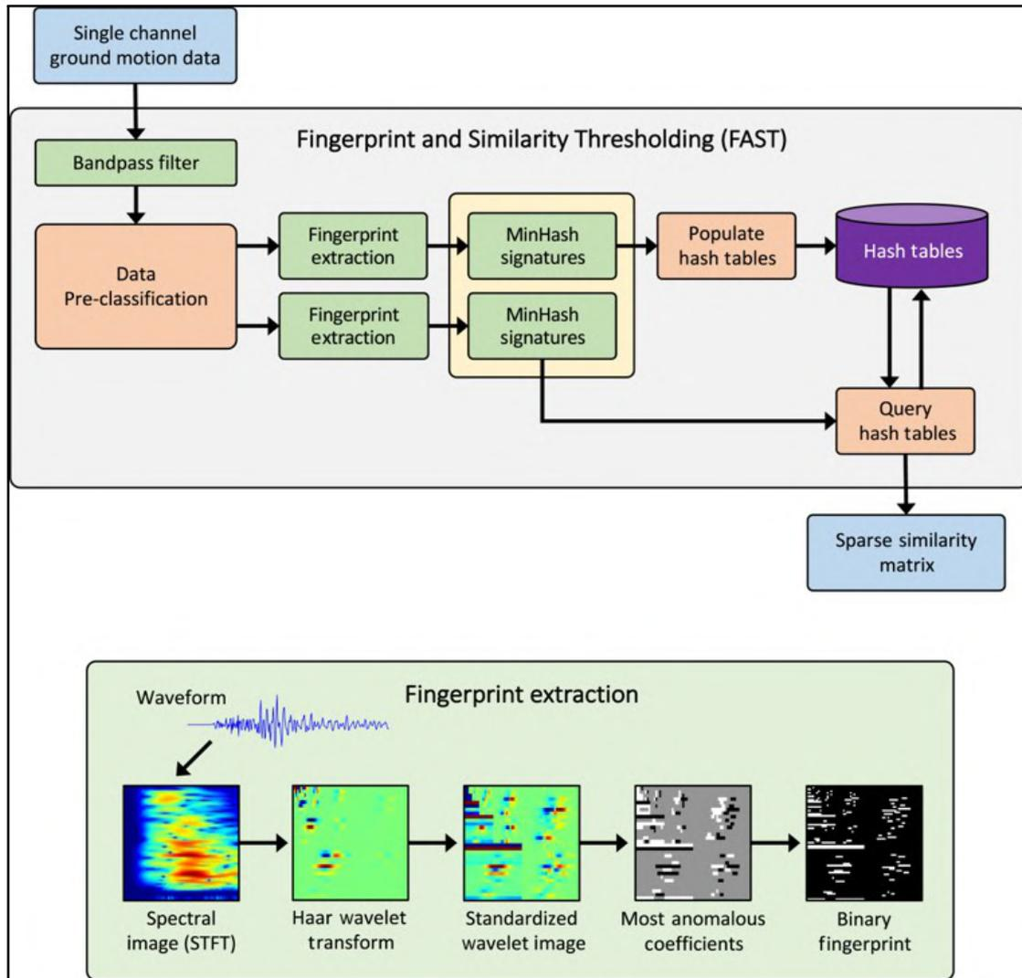
Figure 3-1: Single-station implementation of the FAST approach. **Top:** Illustration of the main workflow in the FAST algorithm. **Bottom:** Fingerprint extraction and conversion into binary format. Source: [Bergen and Beroza, 2018]
