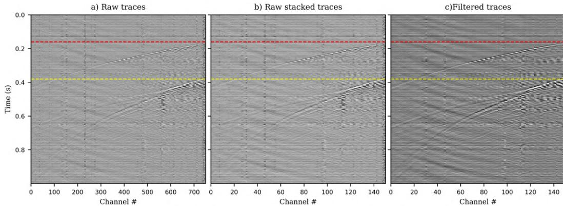
Figure 4-13: Sample detected event (a) raw DAS traces before stacking (b) raw traces after stacking (c) same traces after 300  $Hz$  minimum phase low-pass and 2-D spatial filtering. P-wave arrival (red) and S-wave arrival (yellow). Source: [Wamriew et al., 2021b]
