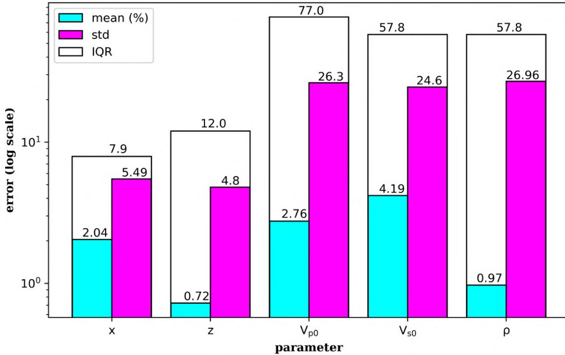
Figure 4-21: Error bar graph for the location and velocity model parameters inverted by deep learning. The vertical scale is logarithmic while the parameters are shown on the horizontal axis with their respective values at the top of each bar. Cyan, purple and white bars represent the mean absolute error, standard deviation and the interquartile ranges respectively. Source: [Wamriew et al., 2021b].
