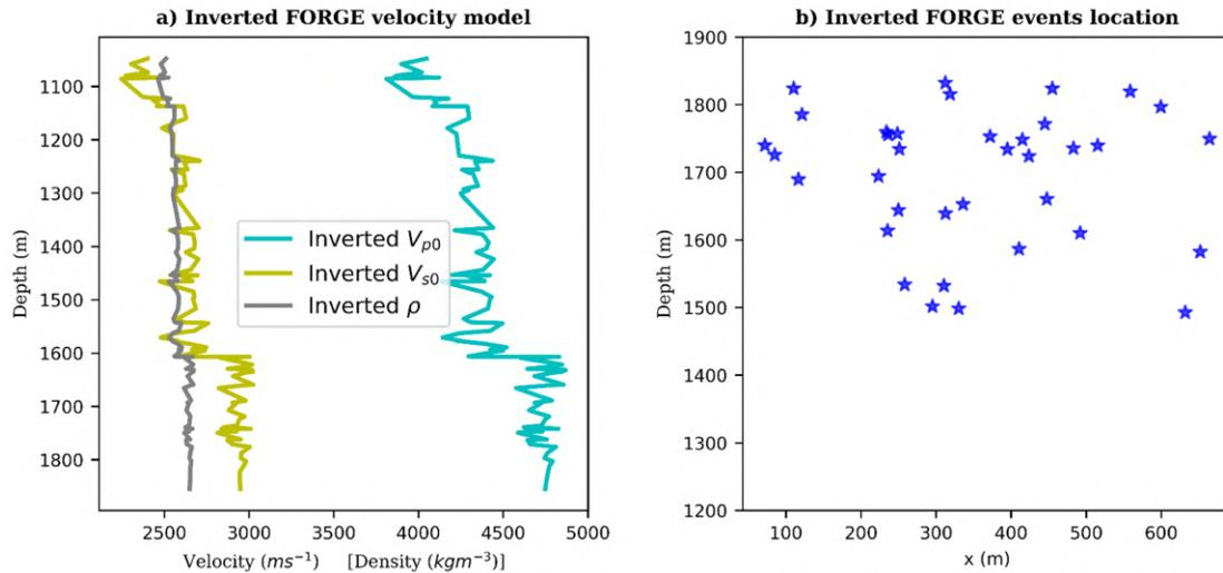
Figure 4-22: Inversion results: (a) Velocity model of FORGE estimated by the neural network. Cyan, yellow and grey curves are the raw patterns output of  $v_{p0}$ ,  $v_{s0}$  and  $\rho$  by the network, (b) Events locations. Source: [Wamriew et al., 2021b].
