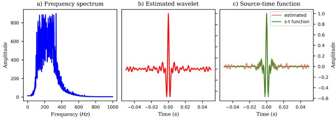
Figure 4-14: Statistical wavelet estimate from field data (a) mean frequency spectrum of field signal (b) estimated wavelet from field data (c) source time function used in generating synthetic data. Source: [Wamriew et al., 2021b]
