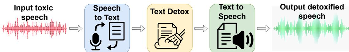
Figure 8-8: The pipeline of speech detoxification based on the already implemented text detoxification technologies.
