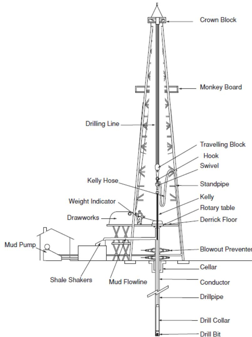
Figure 1 – Drilling rig components ([5]).
