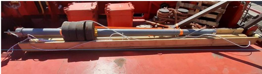
Figure 18. A sampling of bottom sediments by a gravitational steel pipe.
