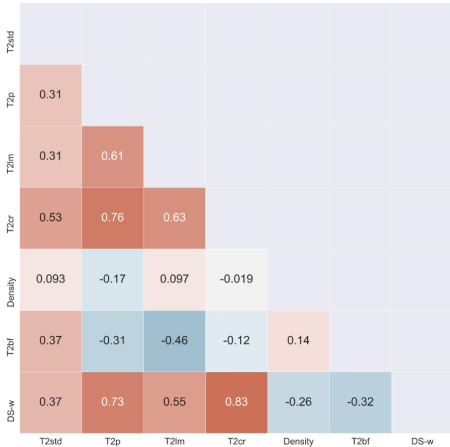
Figure 30: The diagonal correlation matrix shows the linear dependence between six input features with Dean-Stark water content (DS-w) in the training set. Scores represent Pearson's correlation coefficient and are color-coded (heatmap).
