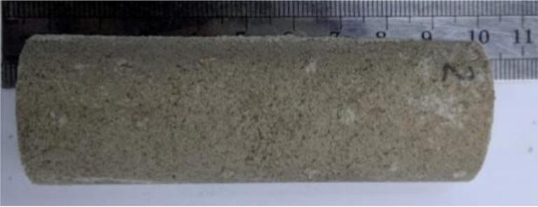
Figure 17. The appearance of frozen sand filled with pore hydrate after extraction from the pressure cell.
