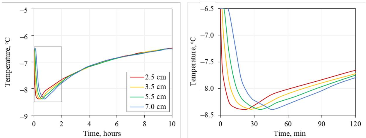
Figure 33. Dynamics of temperature change in time in a frozen hydrate-containing sample ( $S_h^{in}=38\%$ ,  $S_i^{in}=15\%$ ) on the distance 2.5; 3.5; 5.5 and 7.0 cm from the contact zone with 1 N NaCl solution ( $t_{in}= -6.5\text{ }^{\circ}\text{C}$ ,  $P=0.1\text{ MPa}$ ).
