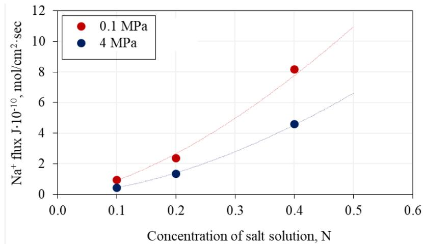
Figure 56. Influence of contact solution concentration on the average Na<sup>+</sup> flux in frozen hydrate-saturated sample (fine sand-2) after 4 hours of the interaction ( $t = -6^{\circ}\text{C}$ ,  $P = 0.1 \text{ MPa}$  and  $4.0 \text{ MPa}$ ).
