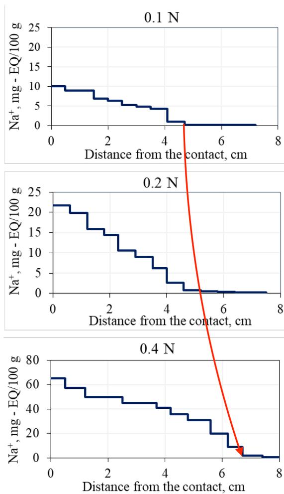
Figure 52. Effect of contact solution concentration on the accumulation of salt ions ( $\text{Na}^+$ ) in frozen hydrate-containing samples (fine sand-2) after 4 hours of interaction with NaCl solution ( $t=-6^\circ\text{C}$ ,  $P=0.1$  MPa).
