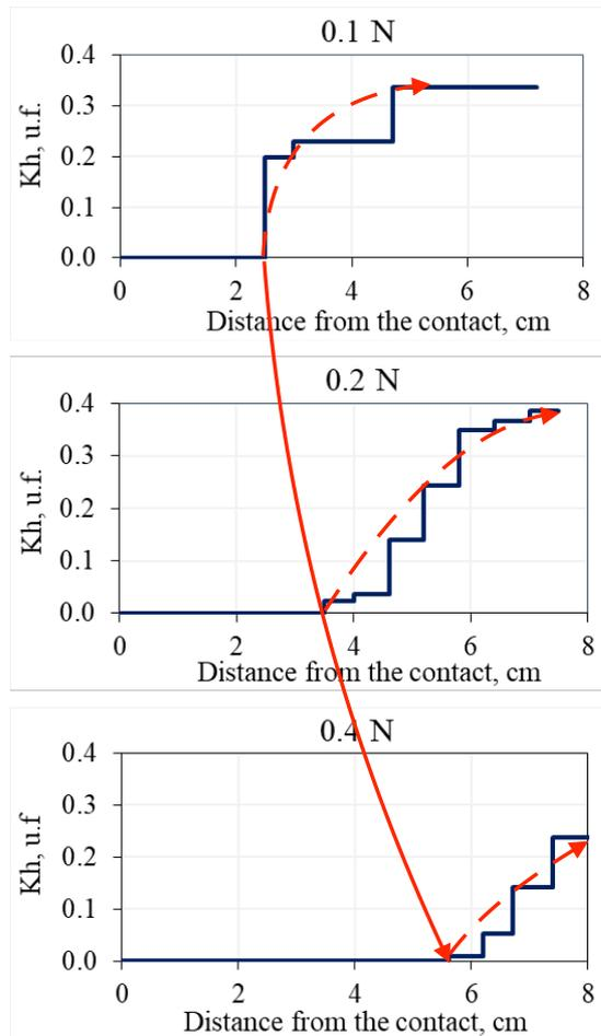
Figure 53. Influence of NaCl contact solution concentration on the distribution of hydrate coefficient ( $K_h$ ) along the length of frozen hydrate-containing samples (fine sand-2) ( $K_h^{\text{in}} \sim 0.4$ ,  $W=12\%$ ) after 4 hours of interaction ( $t=-6^\circ\text{C}$ ,  $P=0.1$  MPa).
