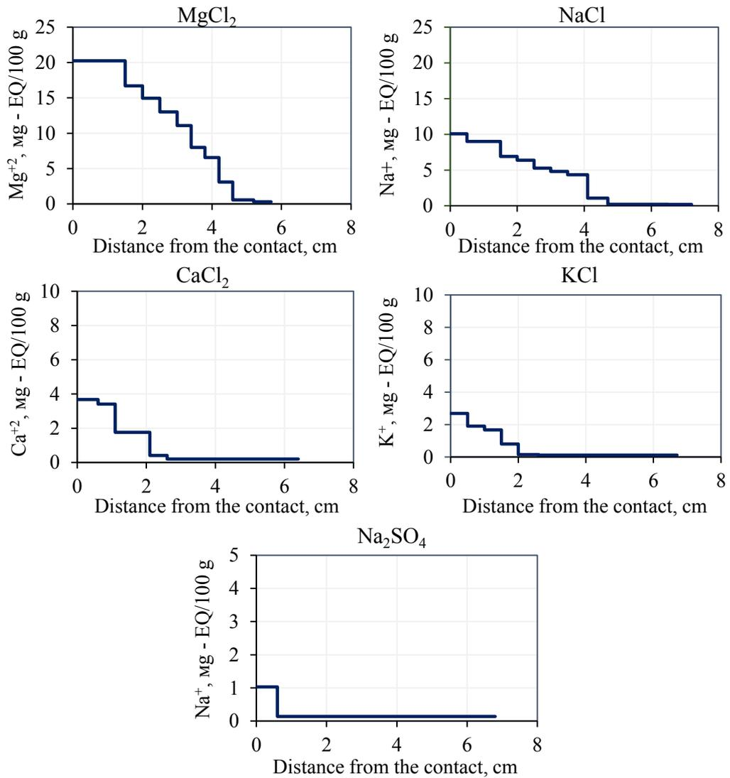
Figure 58. Accumulation of Na<sup>+</sup> ions in samples of frozen hydrate saturated sand (fine sand-2, W=12%) after 4 hours of contact with 0.1N NaCl solution of different composition ( $t = -6^{\circ}\text{C}$ ,  $P = 0.1\text{MPa}$ ).
