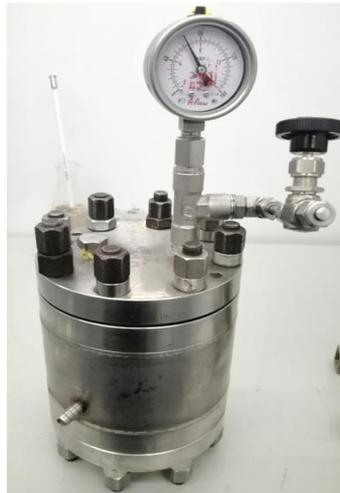
Figure 16. Equipment (pressure cell) for saturation of sediment by hydrate.
