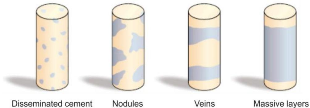
Figure 12. Hydrate distribution in sediments [12].
