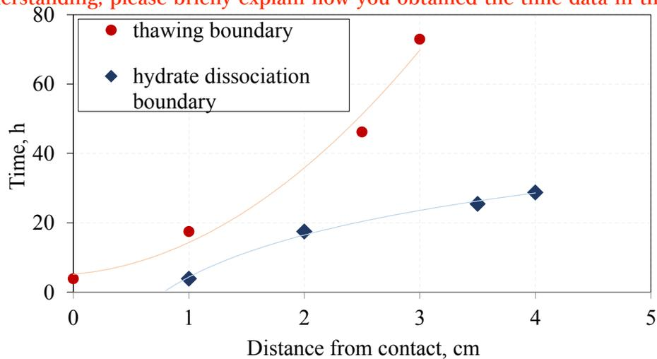
Figure 28. Experimental evaluation of the decomposition front of porous gas hydrates and the thawing front in frozen hydrate-containing sand samples (sand-1,  $W = 12\%$ ) when interacting with 0.1 N NaCl salt solution at a temperature  $-6^{\circ}\text{C}$  and pressure 0.1MPa.
