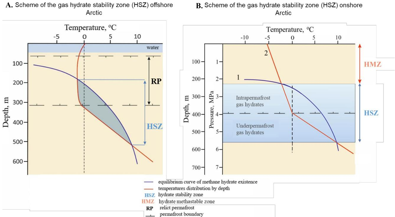
Figure 11. Existence of methane hydrate in natural permafrost conditions (modified from [17,223]).
