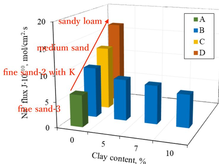
Figure 74. Influence of fineness and amount of clay particles (kaolinite) on the average migration flow of Na<sup>+</sup> in frozen hydrate-saturated samples interacting with NaCl solution 0.1 N for 4 hours at t= -6°C: A – fine sand-3; B – fine sand-2 with kaolinite (from 0 to 10%); C – medium sand; D – sandy loam.
