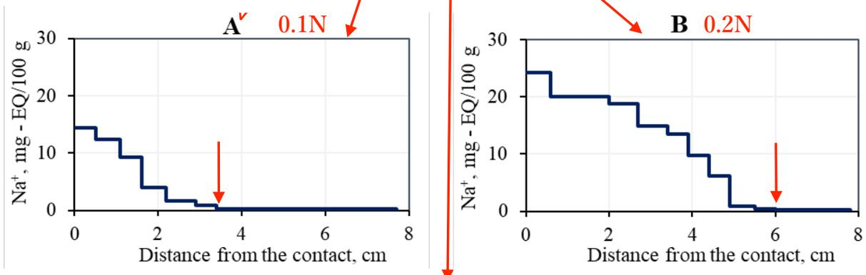
Figure 54. Influence of the contact solution concentration on the accumulation of salt ions ( $\text{Na}^+$ ) in frozen hydrate-containing samples (fine sand-2) interacting for 4 hours under a pressure of 4.0 MPa with a NaCl solution ( $t=-6^{\circ}\text{C}$ ).
