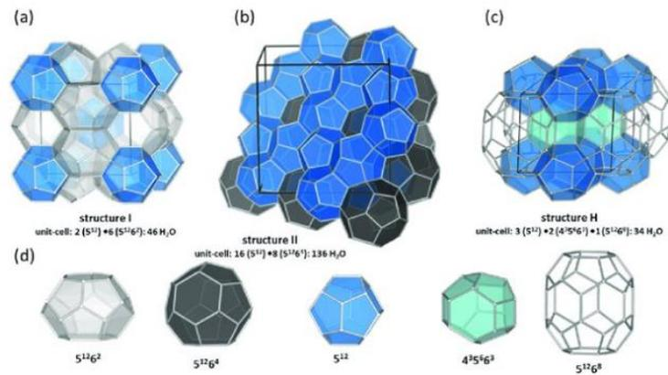
Figure 4. Different crystalline arrangement of hydrates: a – structure I, b – structure II, c – structure H and d – host cages of water. Dense line is the hydrate unit-cell [145].
