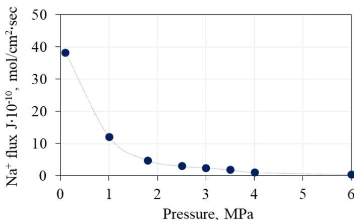
Figure 44. Influence of gas pressure on the flux density of Na<sup>+</sup> ions through the cross section of a frozen hydrate-containing sample 4 hours after the start of interaction with a frozen salt solution 0.1 N NaCl (t= -6°C).
