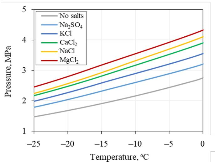
Figure 57. Influence of a chemical composition of salt solution ( $\text{Na}_2\text{SO}_4$ ,  $\text{KCl}$ ,  $\text{CaCl}_2$ ,  $\text{NaCl}$ ,  $\text{MgCl}_2$ ) with a concentration of 5% on the conditions of methane hydrate stability in the range of negative temperatures from 0 to  $-20^\circ\text{C}$  (calculations were made in the “HydraFlash” software).
