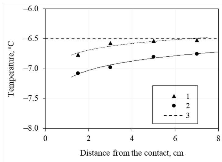
Figure 32. Temperature distribution along the length of a frozen sample (fine sand-2), not containing (1) and containing gas hydrate (2) after 0.6 h of interaction with 0.4 N. NaCl solution at atmospheric pressure. The dotted line - 3 shows the initial temperature  $t_{in} = -6.5^{\circ}\text{C}$ .
