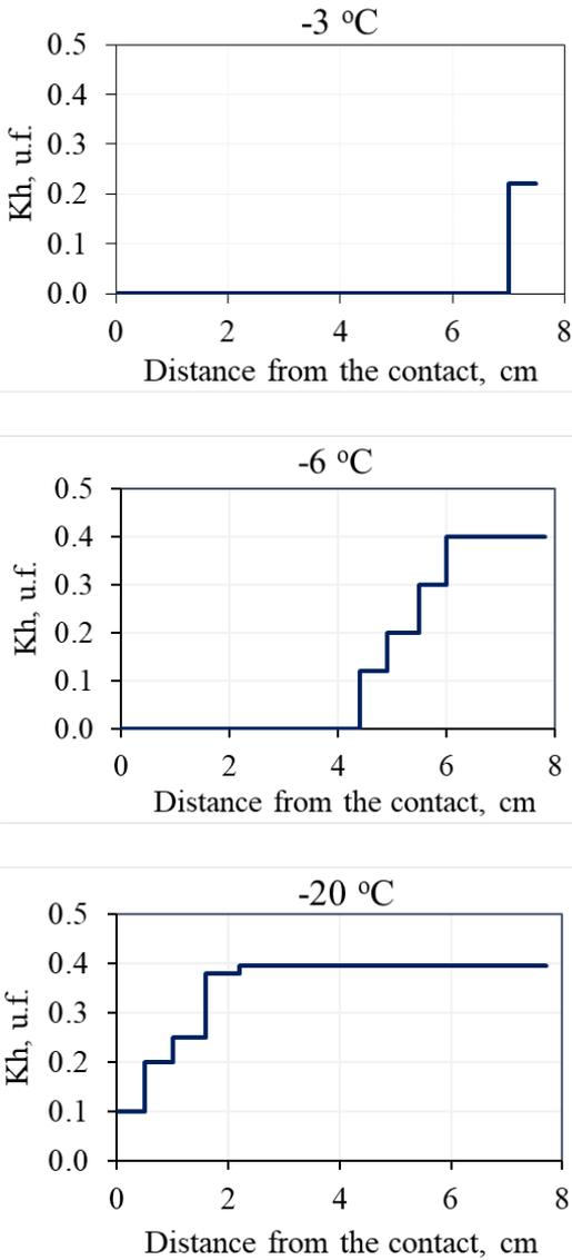
Figure 48. The effect of temperature (-3, -6, -20°C) on the decrease in the hydration coefficient ( $K_h$ ) in samples of frozen hydrate-containing fine sand-2 ( $K_h^{in} \sim 0.4$ ,  $W=12\%$ ) 2 hours after the start of interaction with frozen 0.2 N NaCl salt solution.
