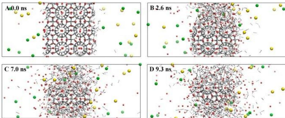
Figure 10. Hydrate decomposition in water by NaCl ions migration in time by mathematical modeling (red – methane, green – Na<sup>+</sup>, yellow – Cl<sup>-</sup>) [201].
