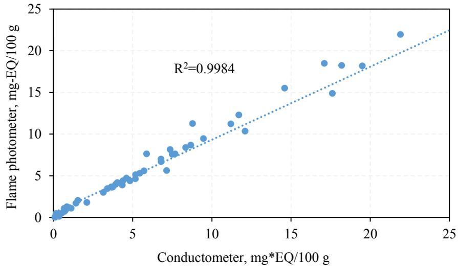
Figure 24. Comparison of the measurement results of the Na<sup>+</sup> concentration by a flame photometer and a conductometer.
