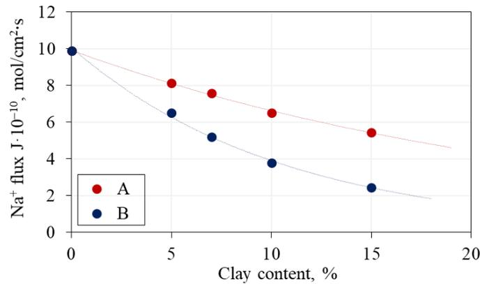
Figure 68. Influence of the content of clay particles of various compositions (kaolinite and montmorillonite) in quartz sand (fine sand-2) on the average flux density of Na<sup>+</sup> ions into a frozen hydrate-containing sample over 4 hours of interaction with a frozen salt solution of 0.1N NaCl (p=0.1MPa, t= -6°C): A – kaolinite; B – montmorillonite.
