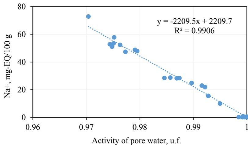
Figure 25. Pore moisture activity versus Na<sup>+</sup> ion concentration.
