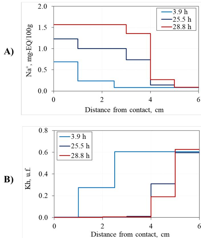
Figure 27. Accumulation of Na<sup>+</sup> ions (A) and changes in the hydrate coefficient (B) in samples of frozen hydrate-containing sand-1 ( $K_h^{in} = 0.6$ ,  $W=12\%$ ) at different times after interaction with NaCl solution 0.1 N ( $P=0.1$  MPa,  $t=-6$  °C).
