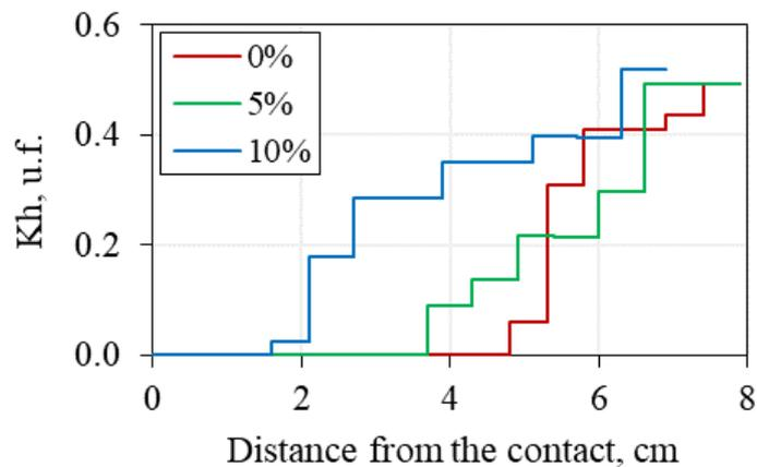
Figure 62. Effect of kaolinite content in sand (fine sand-2) on hydrate dissociation in a frozen hydrate-saturated sample ( $K_h^{\text{in}} \sim 0.5$ ,  $W=12\%$ ) 4 hours after the start of interaction with a frozen salt solution of 0.1 N NaCl at  $-6^\circ\text{C}$ .
