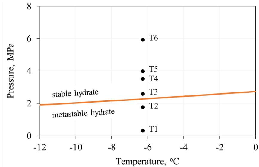
Figure 42. Modeling P-T conditions of methane hydrate stability in the HydraFlash program and thermobaric conditions for conducting experiments on the migration of salt ions in frozen hydrate-saturated sediments (T1-T6).
