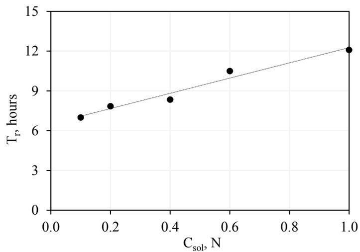
Figure 38. Influence of concentration on the time taken for the temperature of the sample to return to the initial value ( $T_r$ ) after the cooling period caused by the interaction of hydrate-containing frozen sand with saline solution ( $t_{in} = -6.5^\circ\text{C}$ ,  $P = 0.1$  MPa).
