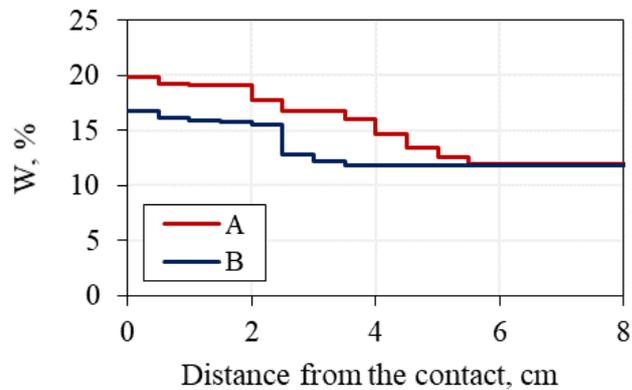
Figure 67. Influence of the mineralogical composition of clay in quartz sand (fine sand-1) on the accumulation of moisture in a frozen hydrate-saturated sample ( $W=12\%$ ) after 4 hours of interaction with a frozen salt solution of 0.1 N NaCl at  $-6^\circ\text{C}$ : A - kaolinite; B - montmorillonite.
