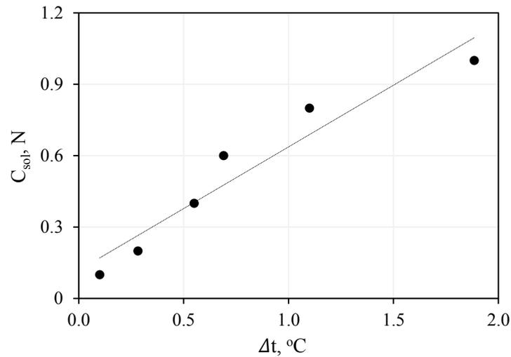
Figure 36. Influence of the contact solution concentration on the maximum temperature drop ( $\Delta t=t_{in}-t_{min}$ ) in frozen hydrate saturated fine sand-2 ( $C_{sol}$  from 0.1 to 1 N,  $t_{in}=-6.5^{\circ}\text{C}$ ,  $P=0.1\text{MPa}$ ).
