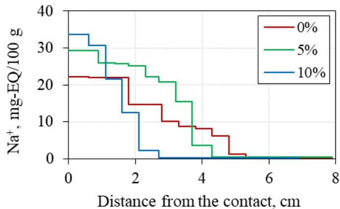
Figure 61. Influence of kaolinite content in fine-grained sand (fine sand-2) on the accumulation of  $\text{Na}^+$  ions in frozen hydrate-saturated samples 4 hours after interaction with 0.1 N NaCl solution at  $-6^\circ\text{C}$ .
