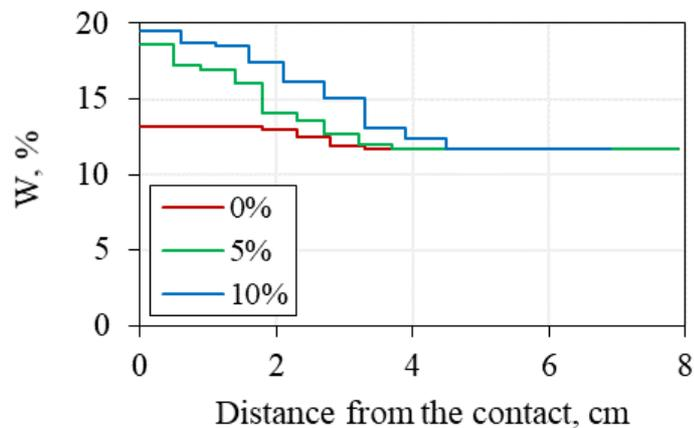
Figure 63. Influence of kaolinite content in sand (fine sand-2) on moisture accumulation in a frozen hydrate-saturated sample ( $W=12\%$ ) after 4 hours of interaction with salt solution of 0.1 N NaCl at  $-6\text{ }^{\circ}\text{C}$ .
