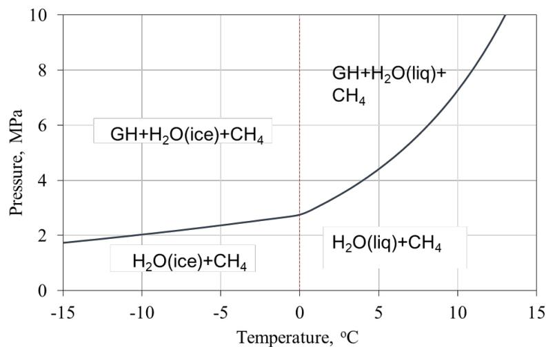
Figure 6. Stability of CH<sub>4</sub> hydrate curve (build in HydraFlash): GH – gas hydrate; liq – liquid water.
