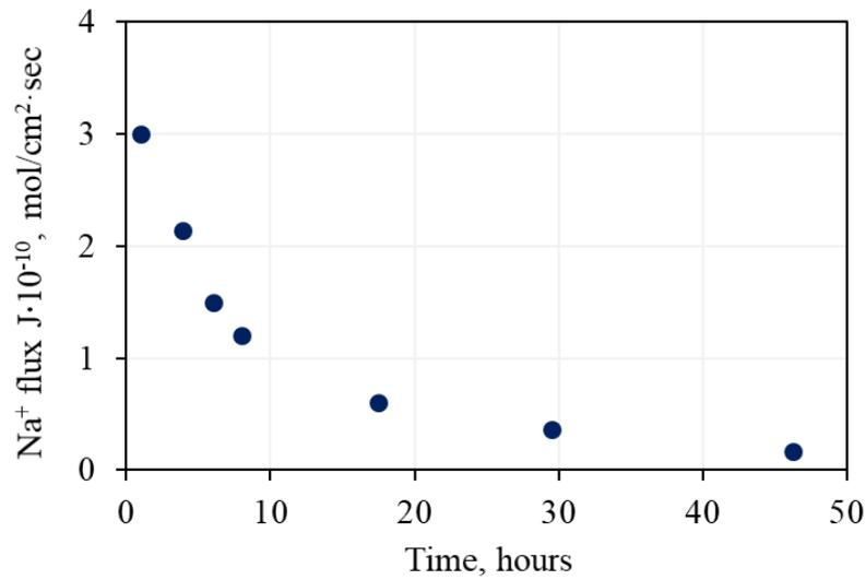
Figure 30. Average Na<sup>+</sup> flux change in time during interaction of frozen hydrate saturated sediment (fine sand-1) with NaCl solution of 0.1N at -6 °C and 0.1 MPa.
