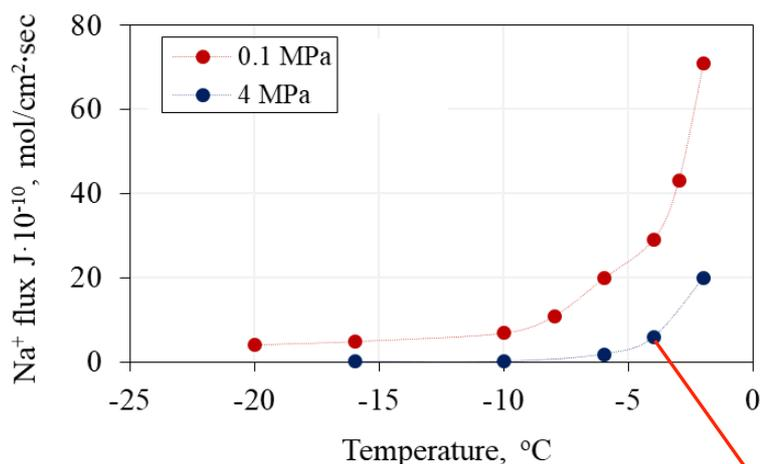
Figure 49. Effect of temperature on the average Na<sup>+</sup> flux into a frozen hydrate-containing sample (fine sand-2) for 4 hours of interaction with a frozen salt solution of 0.1N NaCl (P=0.1MPa).
