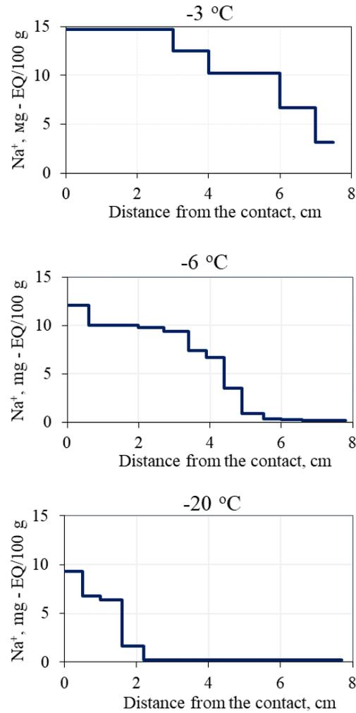
Figure 47. Effect of temperature on the accumulation of salt ions ( $Na^+$ ) in frozen hydrate-containing samples (fine sand-2) after 2 hours of interaction with 0.2 N NaCl solution.
