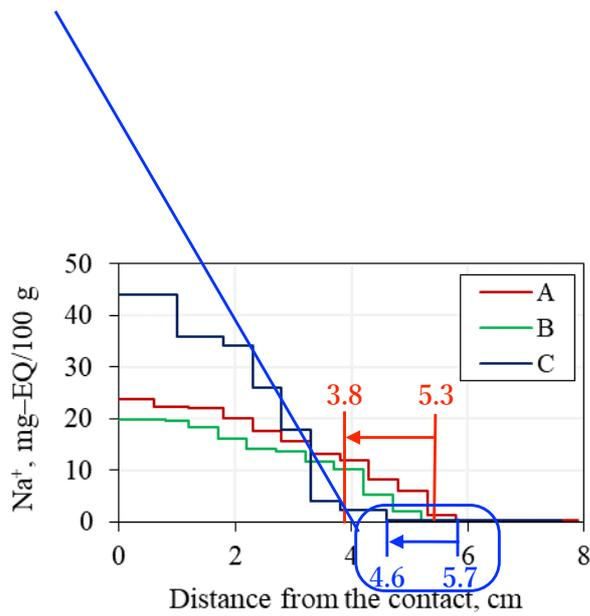
Figure 71. Influence of silt content on the accumulation of salt ions in frozen hydrate-containing samples 4 hours after interaction with 0.1 N NaCl solution at  $t = -6^{\circ}\text{C}$ : A – fine sand-2 (silt ~ 1%); B – fine sand-3 (silt ~ 5%); C – sandy loam (silt ~ 18%).
