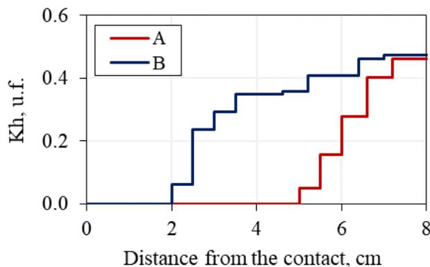
Figure 66. Influence of the mineralogical composition of clay in quartz sand (fine sand-2) on the decrease in the hydration coefficient ( $K_h$ ) in frozen hydrate-containing samples ( $K_h^{\text{in}} \sim 0.4$ ,  $W=12\%$ ) 4 hours after the start of interaction with frozen salt solution 0.1 N NaCl at  $t=-6^\circ\text{C}$ : A – kaolinite; B, montmorillonite.
