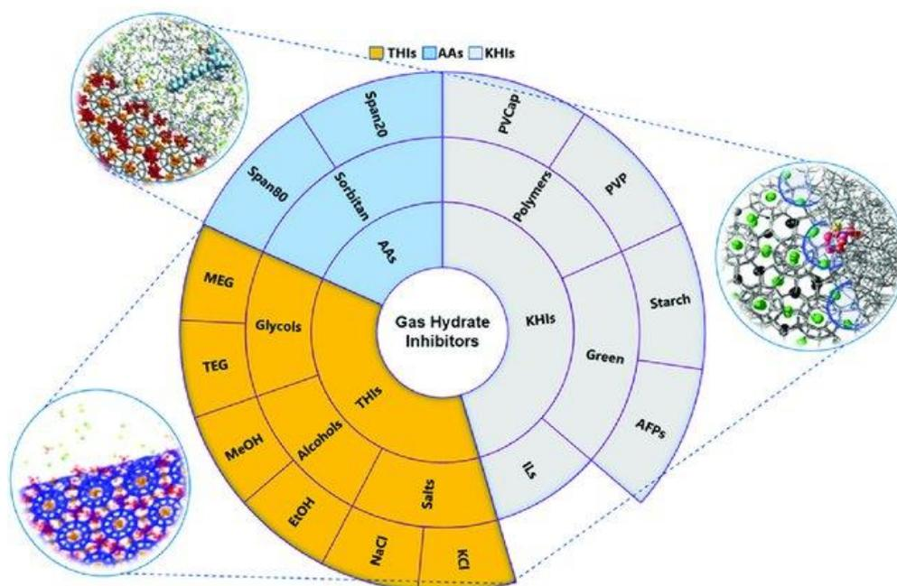
Figure 9. Different hydrate inhibitors and scheme of their work principle [145].
