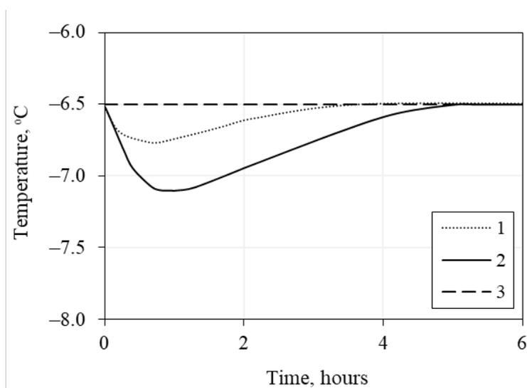
Figure 31. Dynamics of temperature change in time in the near-contact area (2.5 cm from the contact) in frozen sand samples (fine sand-2) interacting with 0.4 N saline solution at atmospheric pressure: 1 – non-hydrate-containing frozen sample (dotted line); 2 - hydrate-containing (solid line); 3 - initial temperature (tin) -6.5 °C (dashed line).
