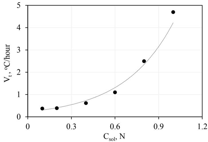
Figure 37. Influence of contact solution concentration on the rate of temperature decrease ( $V_t$ ) of frozen hydrate-saturated fine sand-2 ( $C_{sol}$  from 0.1 to 1 N,  $t_{in} = -6.5^\circ\text{C}$ ,  $P = 0.1$  MPa).
