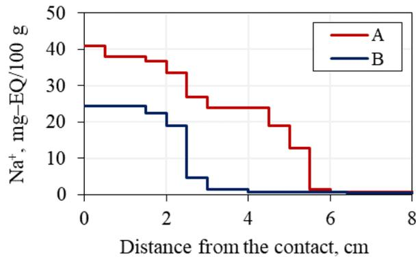
Figure 65. Influence of the mineralogical composition of clay in quartz sand (fine sand-2 with 5% additives) on the accumulation of  $\text{Na}^+$  ions in frozen hydrate-saturated samples after 4 hours of interaction with 0.1 N NaCl solution at  $t=-6^\circ\text{C}$ : A – kaolinite; B – montmorillonite.
