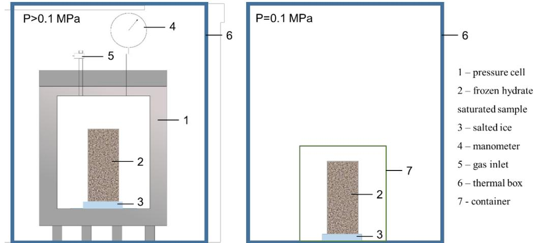
Figure 19. Scheme of the installation for the interaction of frozen hydrate-saturated and non-hydrate-saturated sediments with salt solutions under pressure.
