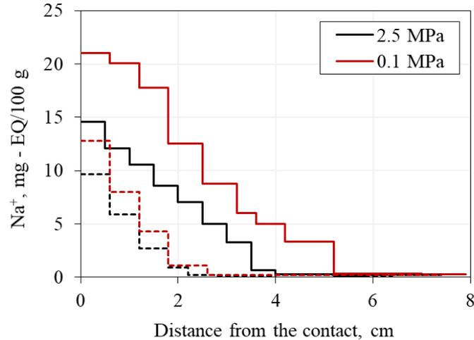
Figure 26. Effect of gas pressure on the accumulation of salt ions ( $\text{Na}^+$ ) in frozen sand (fine sand -1) samples ( $W=12\%$ ) containing (solid line) and not containing (dashed line) gas hydrates 4 hours after interaction with 0.2 N NaCl solution ( $t=-6\text{ }^\circ\text{C}$ ).
