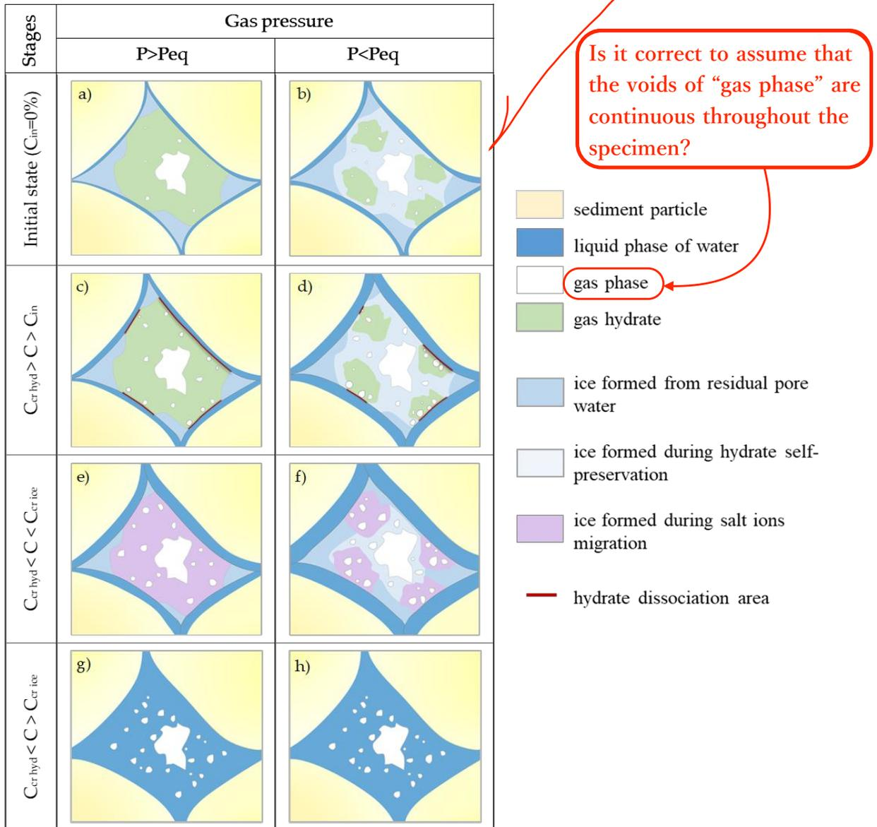
Upon reaching a certain critical salt concentration ( $C > C_{cr\ hydr}$ ) there is a sharp increase in the rate of hydrate dissociation, which leads to its complete decomposition. The moisture formed in this case under conditions of negative temperature and the endothermic effect of dissociation is supercooled and then frozen (Table 9e).
