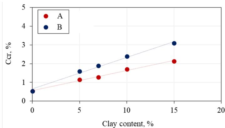
Figure 69. Influence of the content of clay particles of different mineral composition in quartz sand (fine sand-2) on the critical concentration ( $C_{cr}$ ) causing the decomposition of pore hydrate in a frozen sand sample (t= -6°C, p=0.1MPa, C<sub>sol</sub>=0.1N): A – kaolinite; B – montmorillonite.
