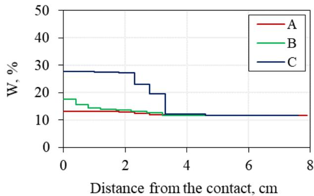
Figure 73. Influence of silt content on moisture accumulation in a frozen hydrate-saturated sample ( $W=12\%$ ) after 4 hours of interaction with a frozen salt solution of 0.1 N NaCl at  $-6\text{ }^{\circ}\text{C}$ : A – fine sand-2 (silt  $\sim 1\%$ ); B – fine sand-3 (silt  $\sim 5\%$ ); C – sandy loam (silt  $\sim 18\%$ ).
