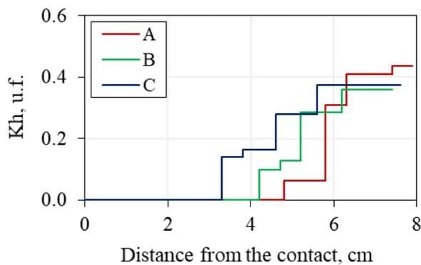
Figure 72. Influence of silt content on the hydrate coefficient ( $K_h$ ) of frozen hydrate-containing samples ( $K_h^{in} \sim 0.4-0.5$ ,  $W=12\%$ ) 4 hours after interaction with 0.1 N NaCl solution at  $t = -6^{\circ}\text{C}$ : A – fine sand-2 (silt ~ 1%); B – fine sand-3 (silt ~ 5%); C – sandy loam (silt ~ 18%).
