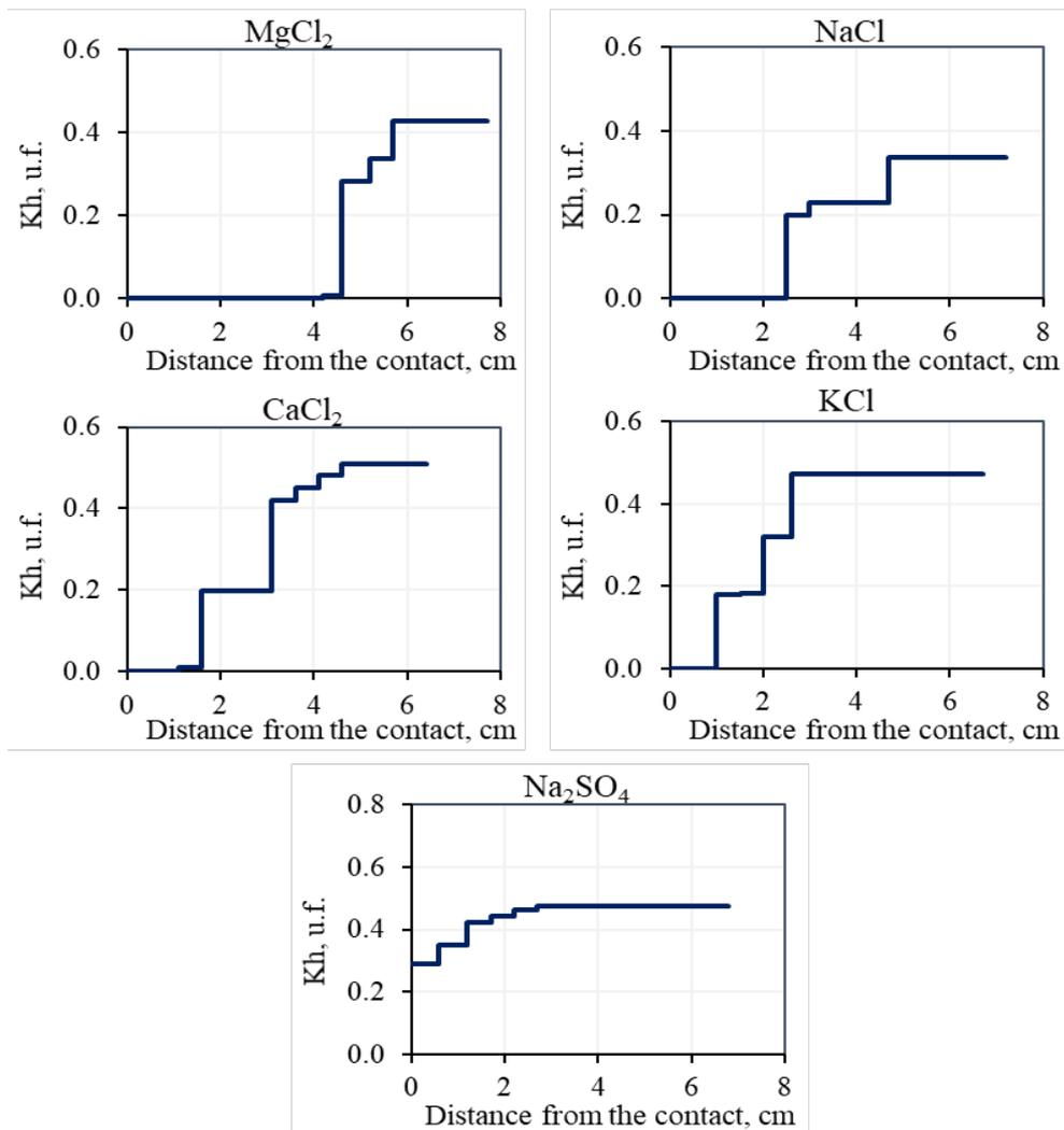
Figure 59. The influence of the chemical composition of the contact salt solution on the decrease in the hydrate coefficient ( $K_h$ ) in frozen hydrate-containing samples (fine sand-2,  $K_h^{\text{in}} \sim 0.5$ ,  $W=12\%$ ) after 4 hours of interaction with the frozen salt solution ( $t=-6.5^\circ\text{C}$ ,  $C_{\text{sol}}=0.1\text{N}$ ,  $P=0.1\text{MPa}$ ).
