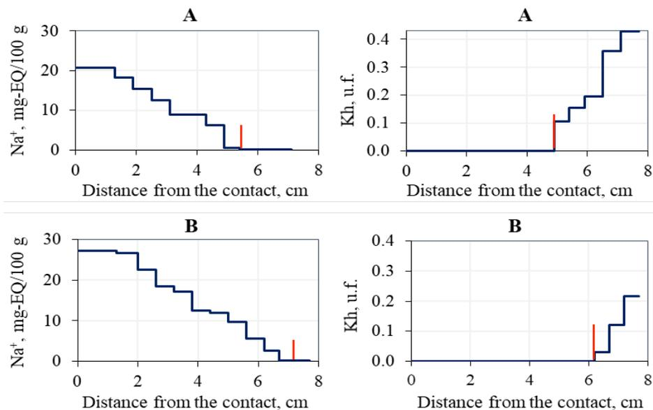
Figure 70. Influence of the size of sand particles on the accumulation of salt ions ( $\text{Na}^+$ ) and the decrease in the hydrate coefficient ( $K_h$ ) in frozen hydrate-containing samples ( $K_h^{\text{in}} \sim 0.4$ ,  $W=12\%$ ,  $t=-6^{\circ}\text{C}$ ) 4 hours after the start of interaction with frozen salt solution 0.1 N NaCl: A - fine sand-2 (0.1-0.2 mm ~ 80%); B – medium sand (0.2-0.5 mm ~ 60%).
