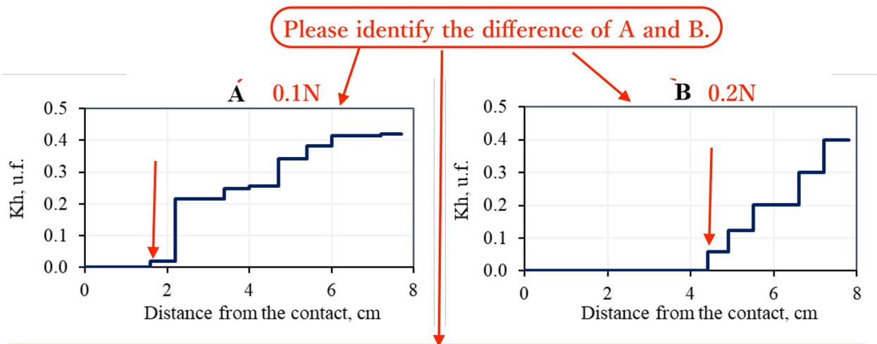
Figure 55. Effect of contact solution concentration on distribution of hydrate coefficient ( $K_h$ ) along the height of frozen hydrate-containing sample (fine sand-2,  $K_h^{in} \sim 0.4$ ,  $W=12\%$ ) after 4 hours of the interaction with frozen NaCl salt solution ( $t=-6^\circ\text{C}$ ,  $P=4.0$  MPa).
