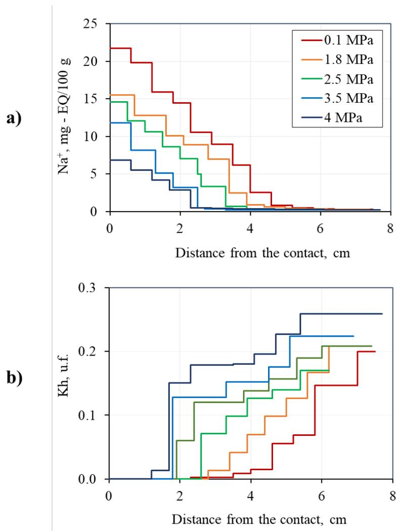
Figure 43. The effect of pressure on the accumulation of salt ions ( $\text{Na}^+$ ) (a) and the decrease in the hydrate coefficient ( $K_h$ ) (b) in samples of frozen hydrate saturated fine sand-2 ( $K_h^{in} \sim 0.3$ ,  $W=12\%$ ) at non-equilibrium and equilibrium pressure 4 hours after the start of interaction with a frozen NaCl solution 0.1 N ( $t=-6^\circ\text{C}$ ).
