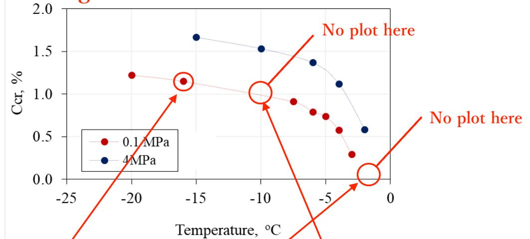
Figure 50. Effect of temperature on the critical concentration (Ccr) causing decomposition of pore hydrate in a frozen sand sample (fine sand-2, P=0.1 and 4MPa, C<sub>sol</sub>=0.1N).
