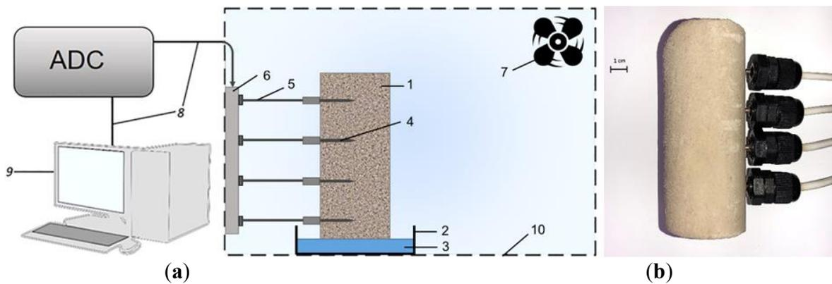
Figure 20. Scheme of Kriolab Tbf system for temperature field change investigation (a) and picture of the frozen hydrate saturated sand sample with temperature sensors (b). 1 - frozen hydrate-saturated sediment; 2 - solution container; 3 - NaCl solution; 4 - temperature sensors; 5 - thermistor streamer; 6 - branch box; 7 - fan; 8 - USB cable; 9 - PC with Kriolab Tbf software; 10 - cooling chamber. Modified after [309].
