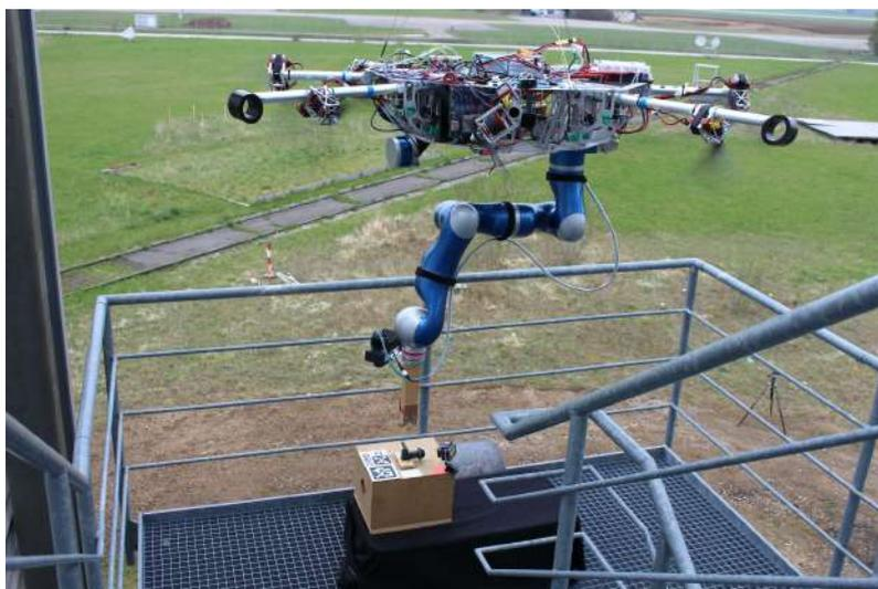
Figure 7-14: The setup for turning the valve.
