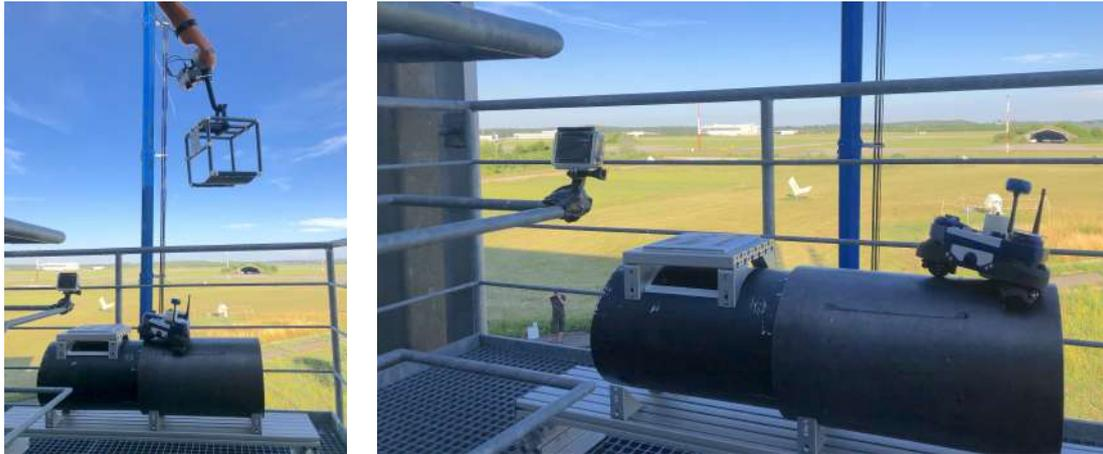
(a) The crawler after the cage lifting
