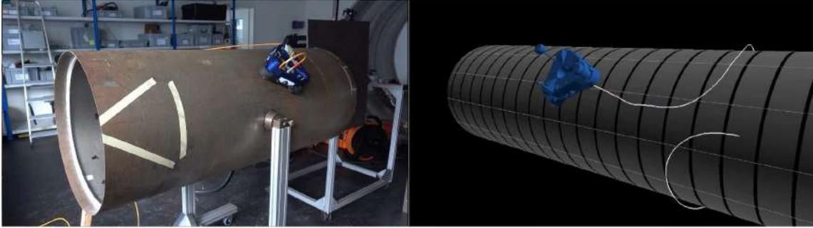
Figure 7-2: The crawler TRIC operates on the pipe (left) and simultaneously localizes itself (right).
