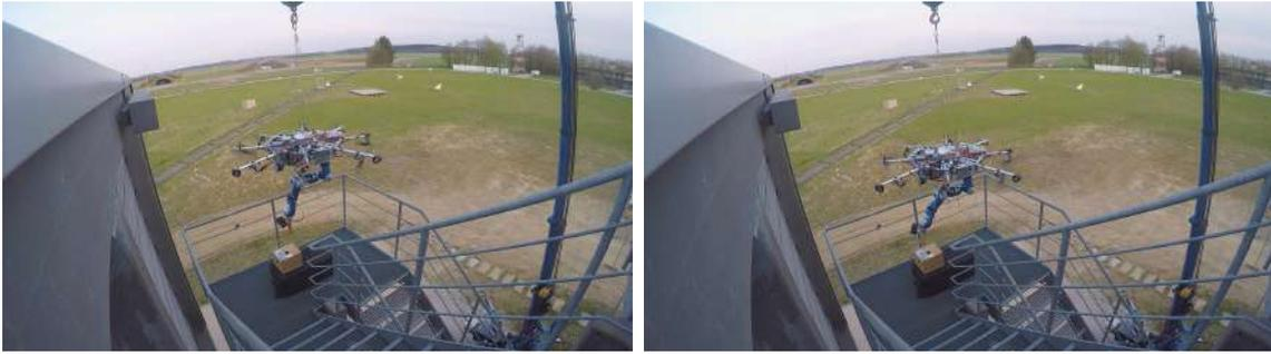
(a) Lowering the SAM toward the box      (b) Adjusting the distance between the platform and the box by null-space control of the platform along vertical axis
