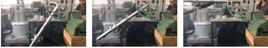
(a) The leg in the lower position (b) The leg in the transition (c) The leg in the upper position
