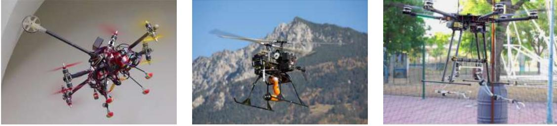
(a) ETH Zurich aerial inspection platform [Bodie et al., 2019, Kamel et al., 2018] (b) DLR Flettner with 7-DOF robotic arm [Huber et al., 2013] (c) University of Seville dual lightweight aerial manipulator [Suárez et al., 2018]
