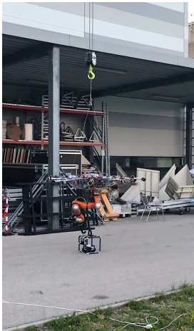
(a) Placing the cage with the crawler on the ground
