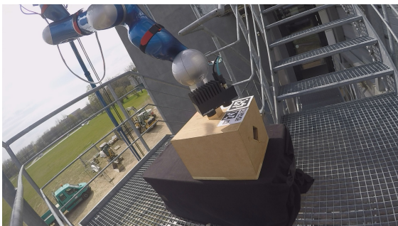
(c) Inserting the peg into the hole
