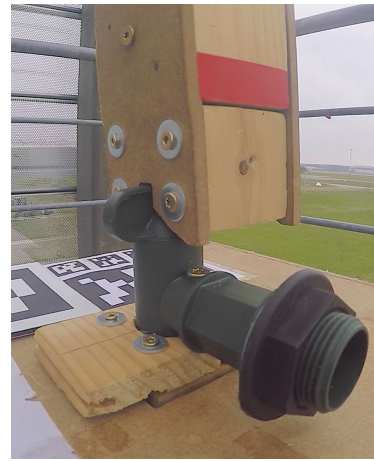
(c) Fitting the tool groove with a valve handle
