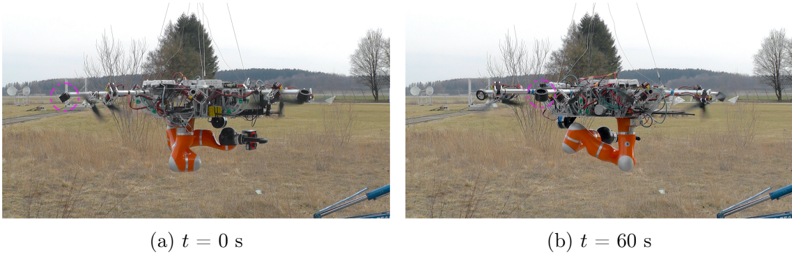
Figure 6-10: Illustration of the experiment: geometric yaw control. Configurations of the SAM platform at t = 0 s and at t = 60 s are shown. The purple dashed circle denotes the location of the landing pad.
