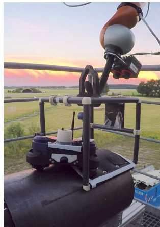
(c) The crawler is halfway into the cage pressed by the tool (the hook)
