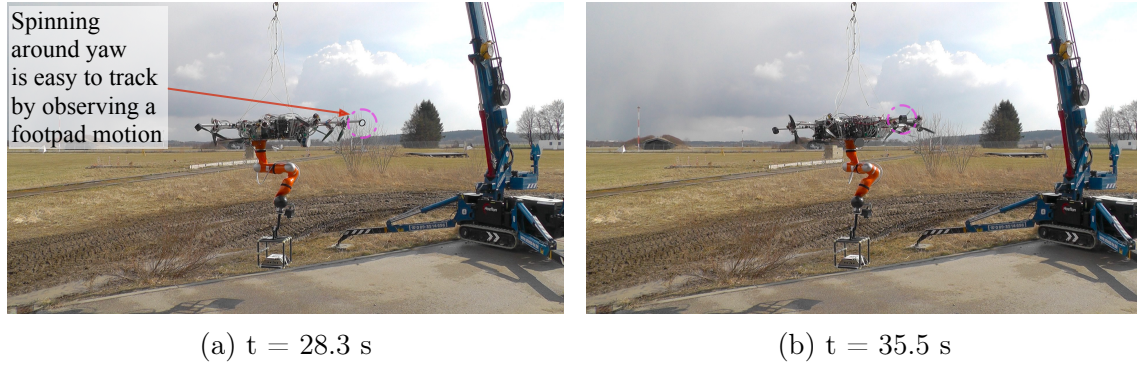
Figure 6-35: Illustration of the experiment: null-space control of the platform around the vertical axis. Snapshots demonstrate the change of the platform orientation around yaw while keeping the same pose of the robotic arm end effector. Purple dashed circle shows the particular footpad location.
