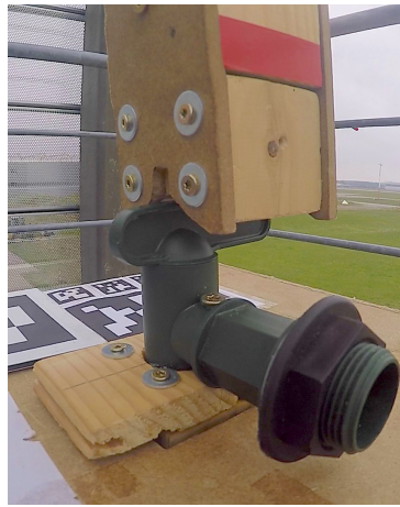
(b) Approaching the valve by the groove of the tool
