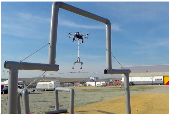
(a) Rigid link-decoupled aerial manipulator [Suárez et al., 2018]
