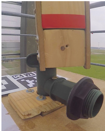
(d) Turning the valve handle by rotation of the end effector for roughly 45 degrees
