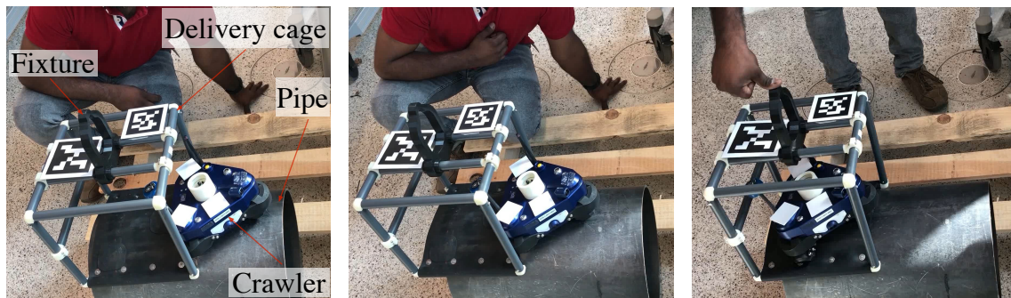
(a) The crawler is at the beginning of the movement toward the cage (b) The crawler pushes the free-placed cage instead of getting in (c) The crawler moves in the cage pressed by external vertical force (by human thumb)
