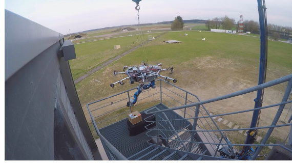
(b) Adjusting the distance between the platform and the box by null-space control of the platform along vertical axis
