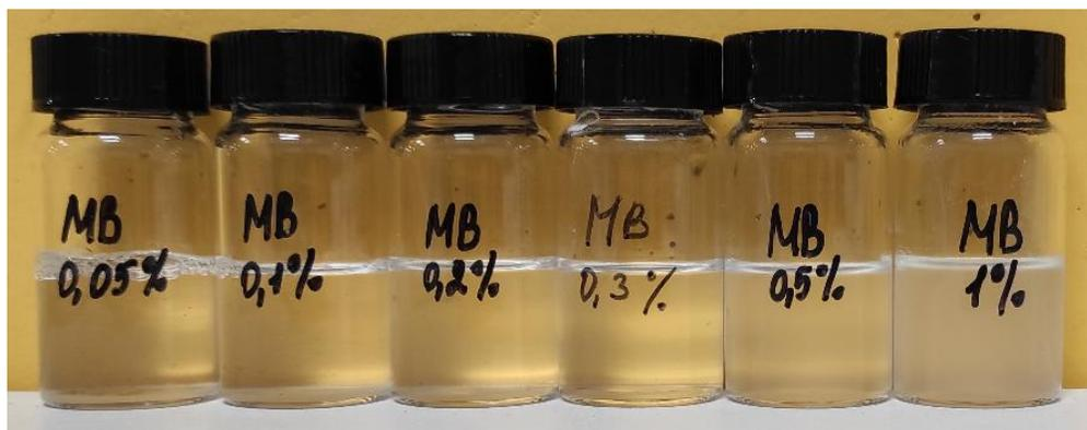
Appearance of surfactant solutions with the addition of sodium metaborate tetrahydrate after 14 days of heating at 70°C
