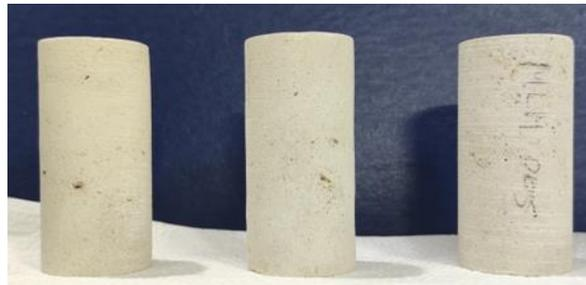
Figure 50. Limestone samples with diameter of 30 mm
