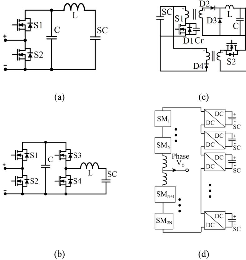
Fig. 23 (a) Half-bridge with SC connected through an inductor, (b) Half-bridge with integrated DC/DC boost converter, (c) Soft-switching SM cell and (d) Alternative MMC topology to include SCs.
