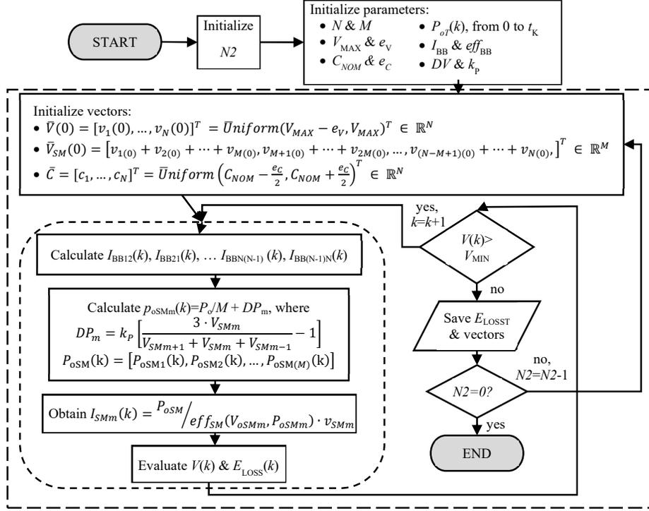
Fig. 40 MMC discharging cycle flow diagram for any Case.
