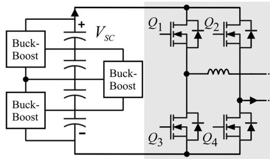
Fig. 39 Internal Buck-Boost balancing system, Case 4 example.
