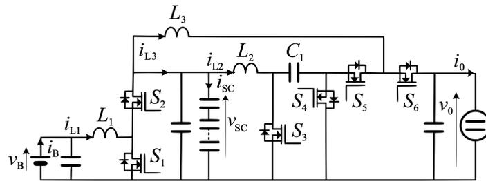
Fig. 12 High-gain dual-input DC/DC converter.
