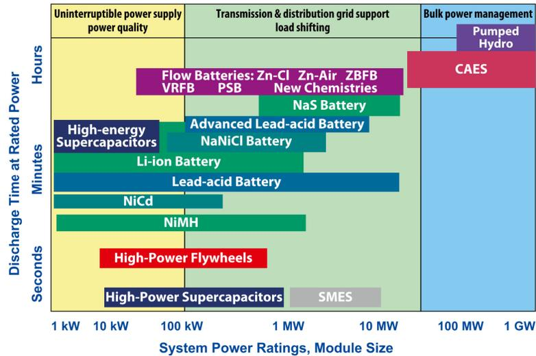
Fig. 5 Energy storage devices ordered based on their power rating and discharging times, and their possible application in the grid [3].
