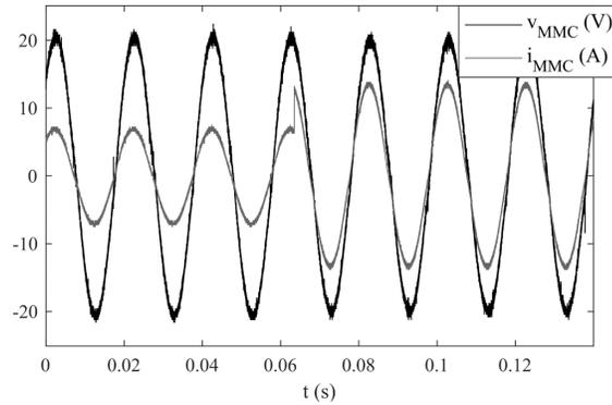
Fig. 49 MMC output voltage and current for a step change in the load.
