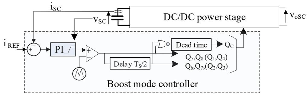
Fig. 29 Proposed SM Boost-mode controller.
