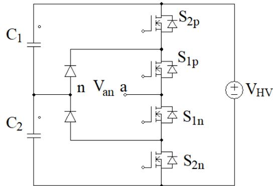
Fig. 20 Diode-clamped 3-level DC/AC multi-level inverter.
