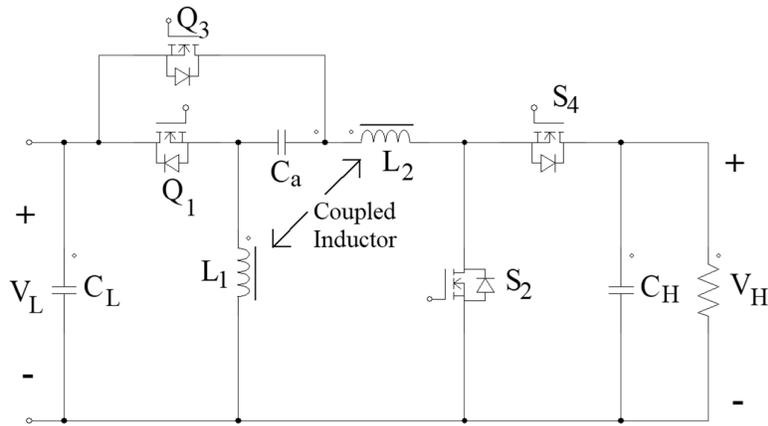
Fig. 8 High-gain bidirectional quadratic DC–DC converter based on coupled inductor.
