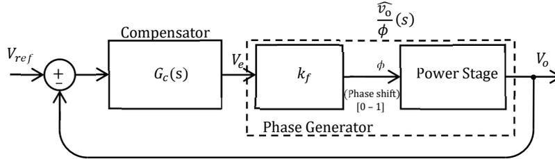
Fig. 31 SM inner control loop.
