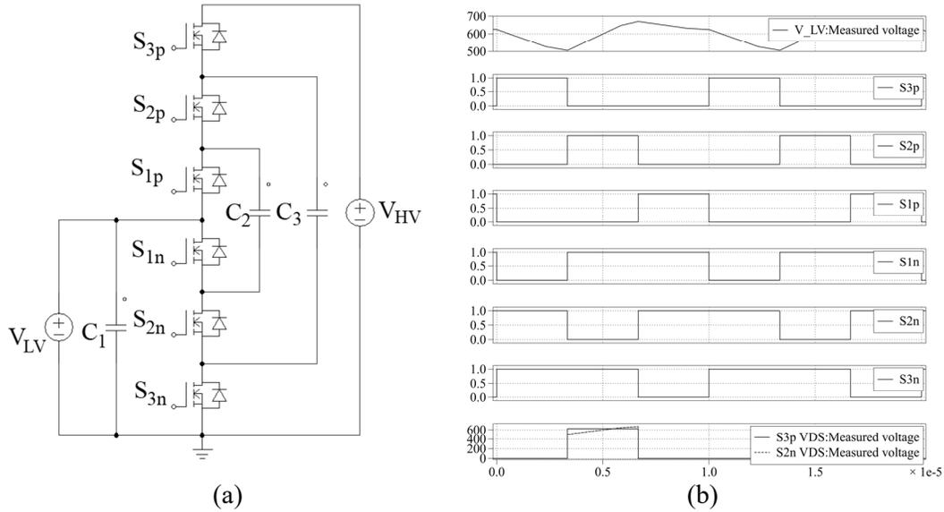
Fig. 14 Flying-capacitor multi-level DC/DC converter, 3 level example.
