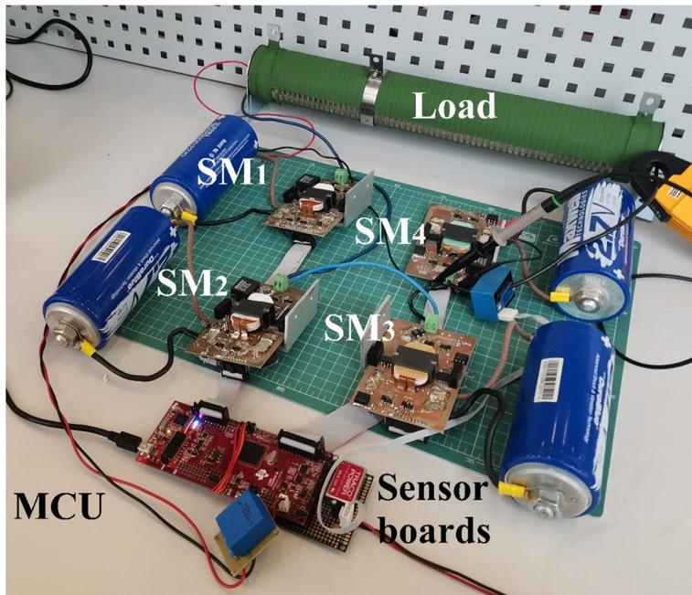
Fig. 47 Complete MMC Prototype.
