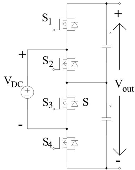
Fig. 16 Multi-level bidirectional DC/DC converter with high efficiency.
