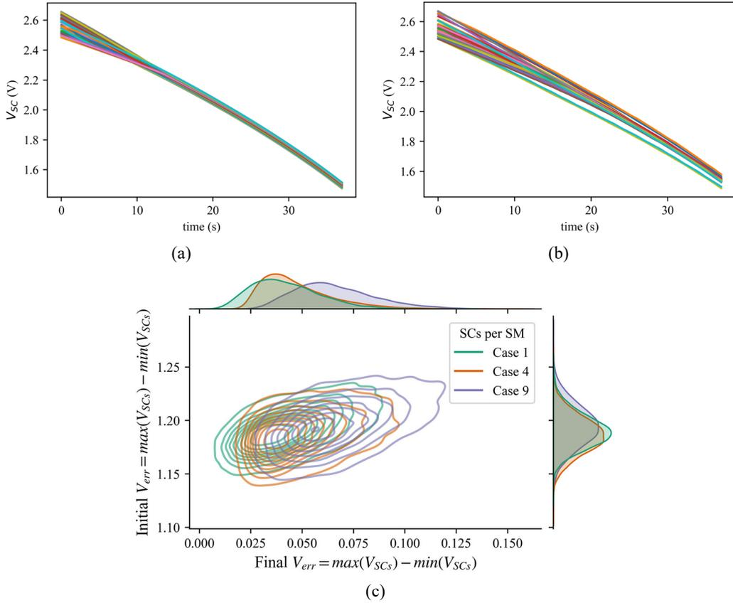
Fig. 41 Voltage plot of each SC for the discharging cycle for (a) Case 1, (b) Case 4 and (c) scattered surface plot for Case 1, 4 and 9.
