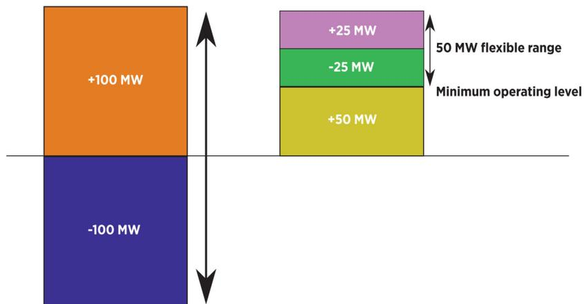
Fig. 3 100MW ESS (left) versus 100MW gas turbine (right) [6].
