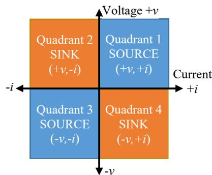
Fig. 18 Four-quadrant plot for bidirectional DC/AC inverters.
