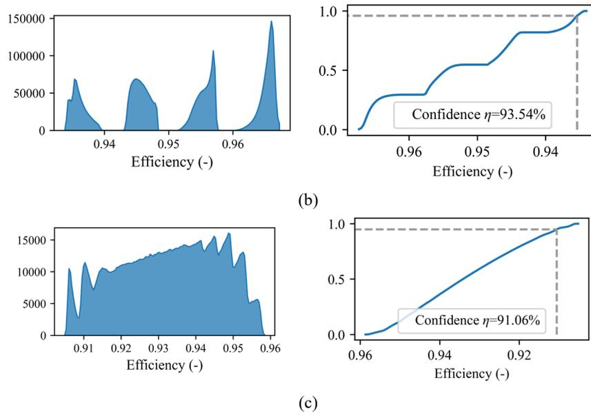
Fig. 42 SM efficiency histograms and CDF plots for Case 1, 4 and 9.
