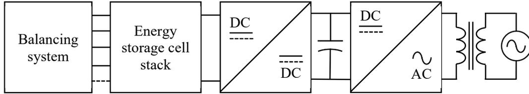
Fig. 7 ESS basic block diagram.
