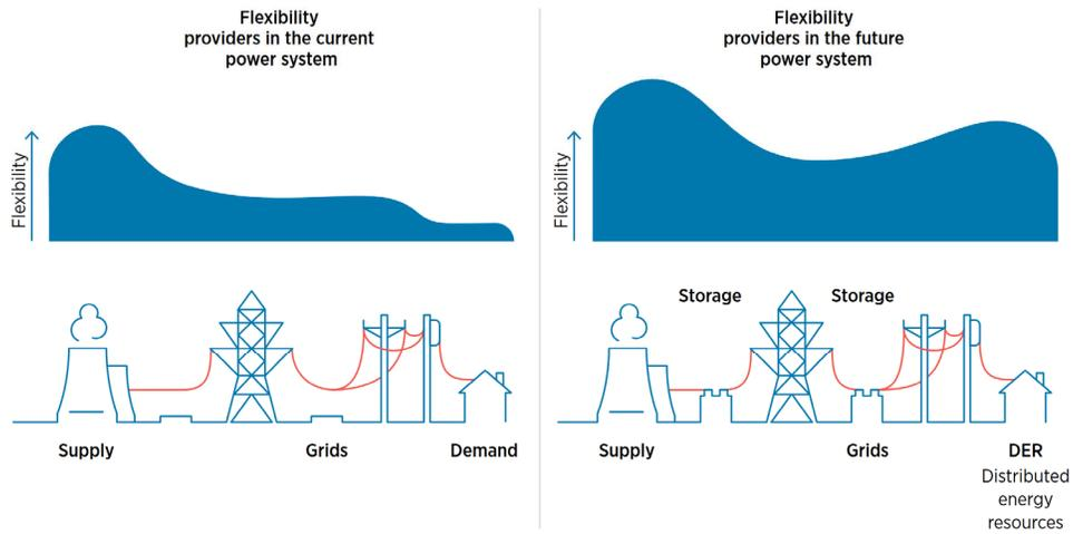
Fig. 2 Traditional grid vs emerging flexible grid [5].
