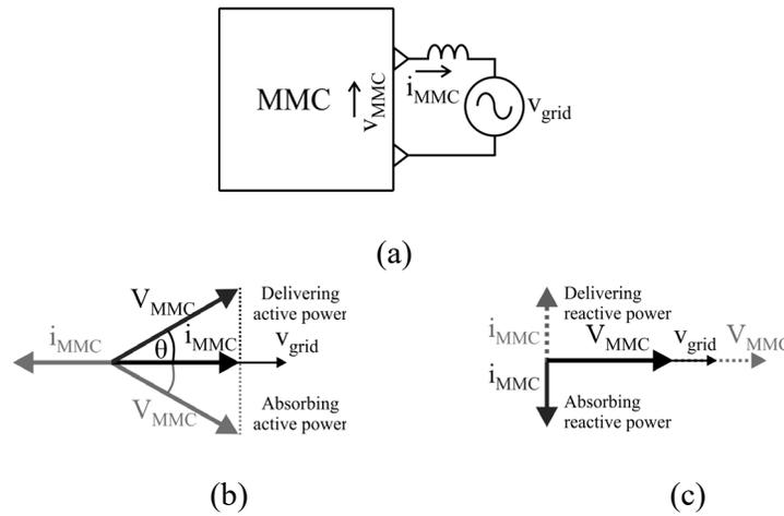
Fig. 34 MMC connected to the grid: (a) basic diagram, (b) phasors when MMC is delivering or absorbing active power, and (c) reactive power.
