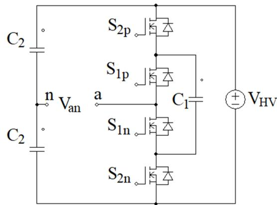
Fig. 19 Capacitor-clamped 3-level DC/AC multi-level inverter.
