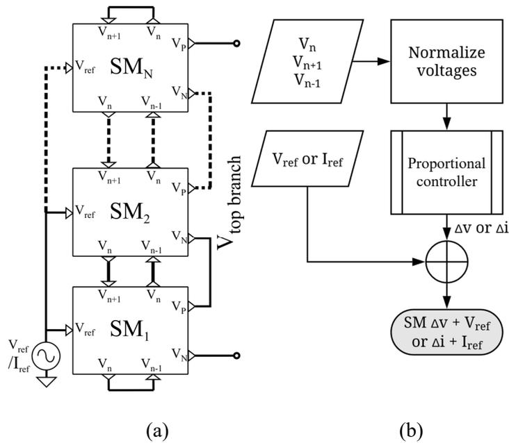
Fig. 33 MMC (a) branch detailed interconnection, and (b) proportional controller of each SM to achieve the self-balancing capability.
