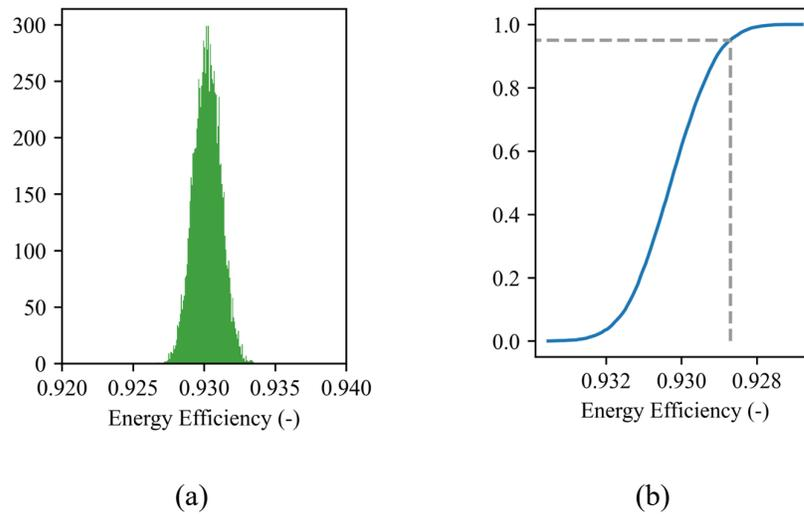
Fig. 54 Probabilistic study based on the extracted SM efficiency from the prototype, (a) histogram and (b) CDF plot.
