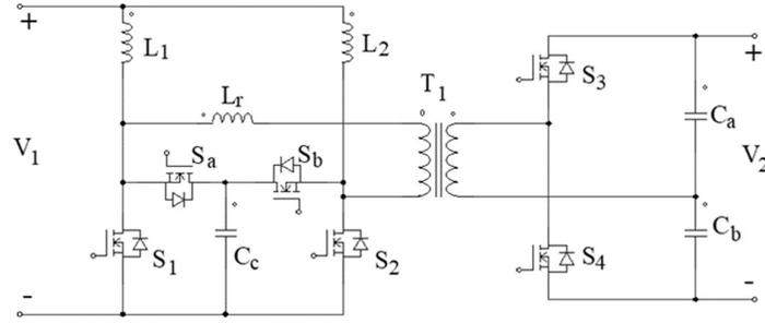
Fig. 11 ZVS bidirectional DC/DC converter with phase-shift plus PWM control scheme.
