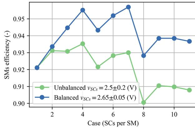
Fig. 43 Minimum SMs efficiency with a confidence level of 95% for unbalanced and balanced initial conditions for all Cases.
