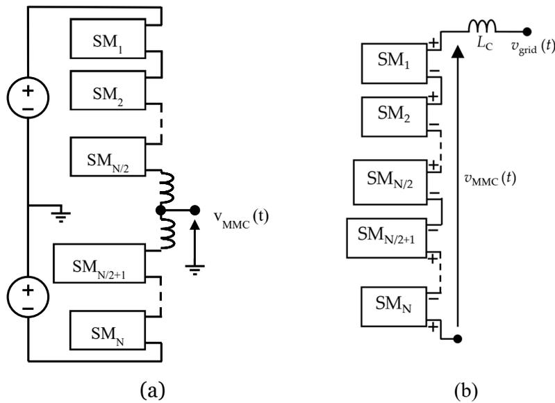
Fig. 25 Block diagram (a) of the traditional and (b) the proposed MMC topology.
