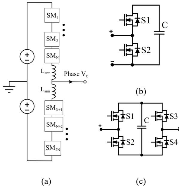
Fig. 22 Modular Multilevel Converter, (a) basic block diagram, (b) half-bridge SM and, (c) full-bridge SM.
