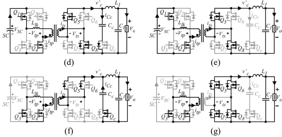
Fig. 28 Bidirectional full-bridge, (a) waveforms, (b) before 1<sup>st</sup> interval, (c) 1<sup>st</sup> interval, (d) 2<sup>nd</sup> interval, (e) 3<sup>th</sup> interval, (f) 4<sup>th</sup> interval and (g) 5<sup>th</sup> interval for the Buck-mode.
