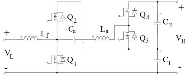
Fig. 10 High-gain soft-switching bidirectional DC/DC converter composed of two half-bridges.
