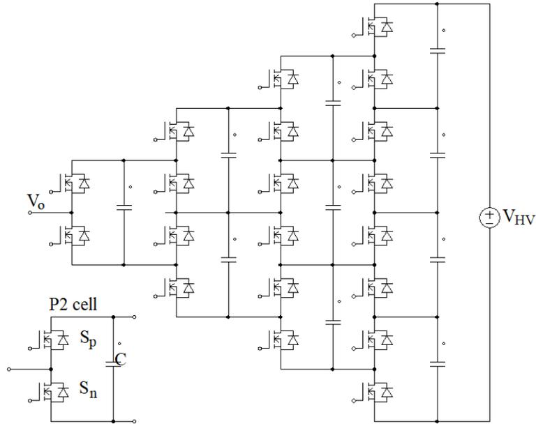
Fig. 21 Generalized multi-level DC/AC inverter with P2 cell.
