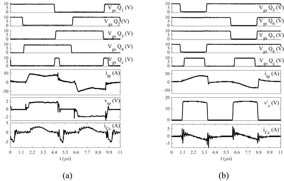
Fig. 48 Experimental waveforms for each SM in (a) buck and (b) boost-mode.
