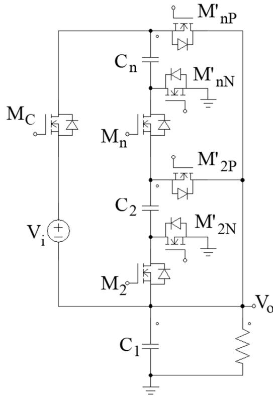
Fig. 15 An n-stage switched-capacitor DC/DC converter schematic.
