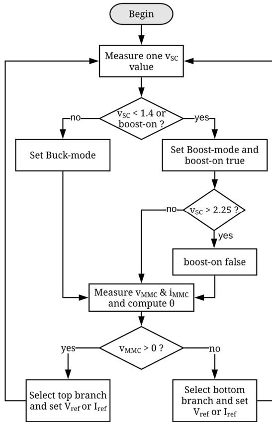
Fig. 36 MMC control diagram for the mode selection.
