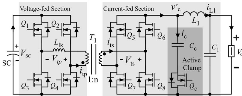
Fig. 26 Bidirectional full-bridge DC/DC converter, presented in [49].
