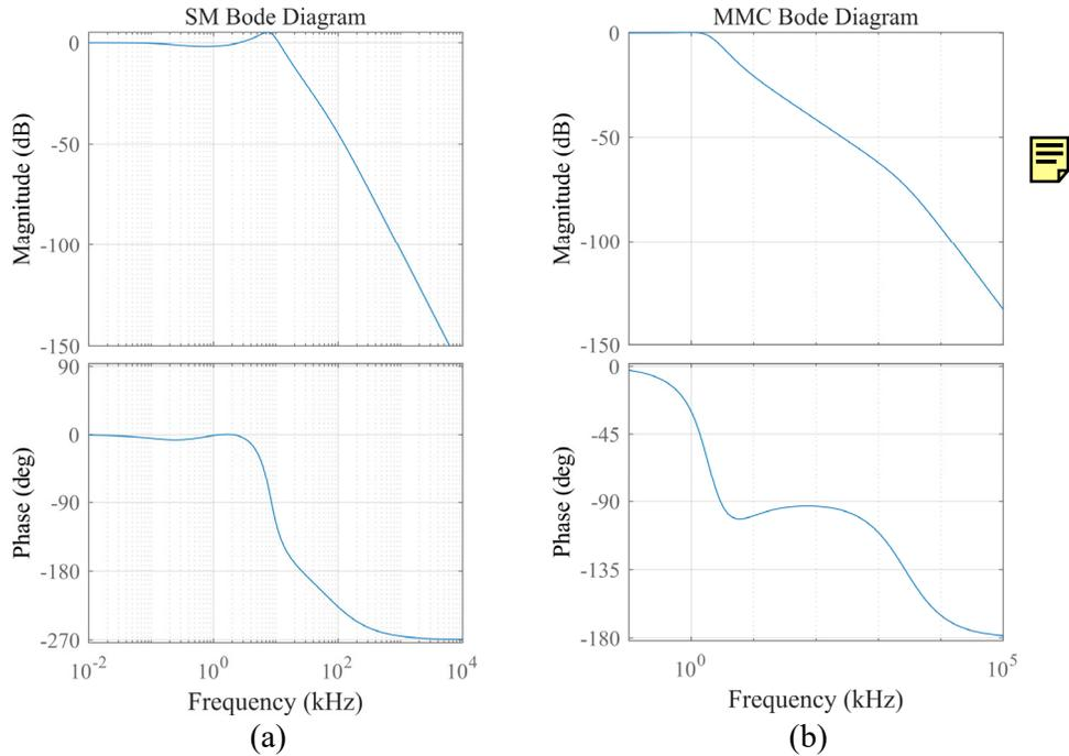
Fig. 32 Closed loop transfer function for: (a) SM using a type-III controller and (b) MMC using a PI controller.
