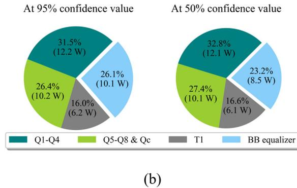
Fig. 46 SM power losses for the main components (a) box plot and (b) pie charts at 95% and 50% confidence levels.
