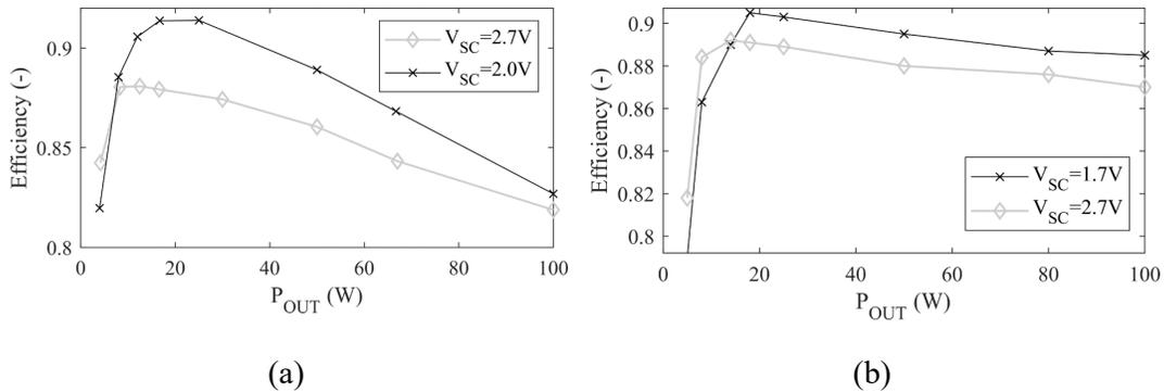
Fig. 51 Efficiency of the MMC for (a) buck and (b) boost-mode.
