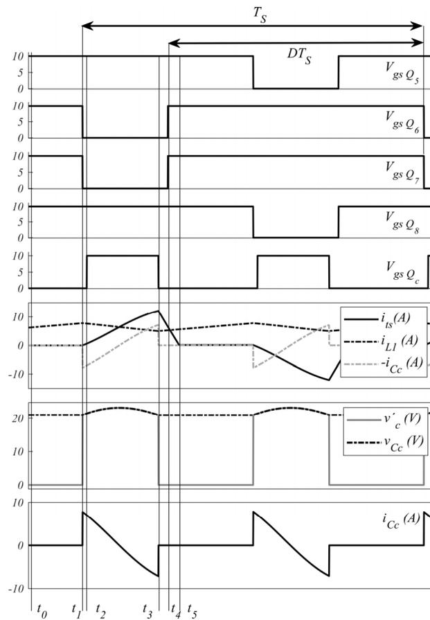
Fig. 30 Bidirectional Full-bridge Boost-mode waveforms.
