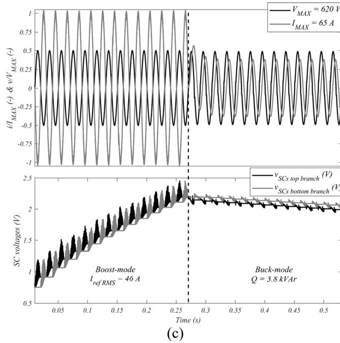
Fig. 37 Buck-mode: (a) balancing process discharging at 10 kW, (b) delivering or absorbing active or reactive power and (c) changing from boost-mode to buck-mode.
