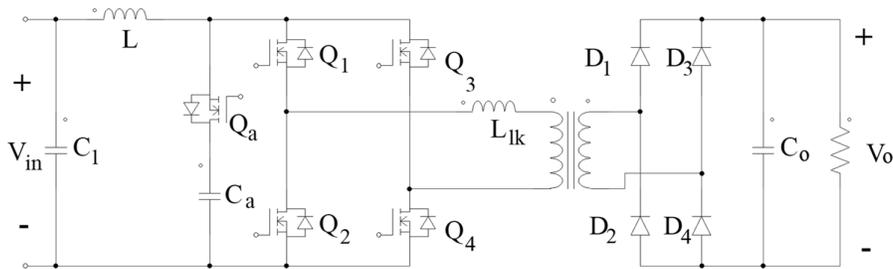
Fig. 13 Extended range ZVS active-clamped current-fed full-bridge isolated DC/DC converter.
