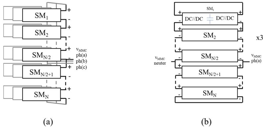
Fig. 38 Extension for a three-phase system: (a) balanced and (b) non-balanced.
