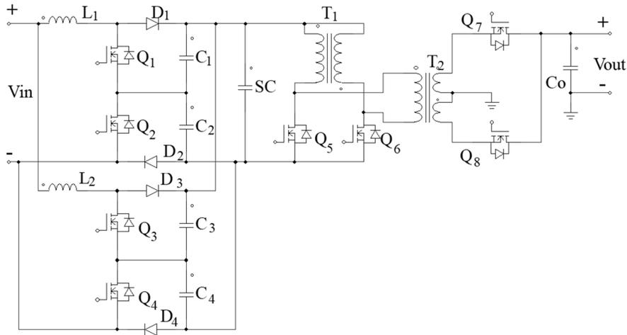
Fig. 9 Wide input range DC/DC converter composed of two cascaded stages.
