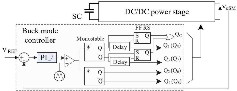
Fig. 27 Proposed SM Buck-mode controller with gating signals.
