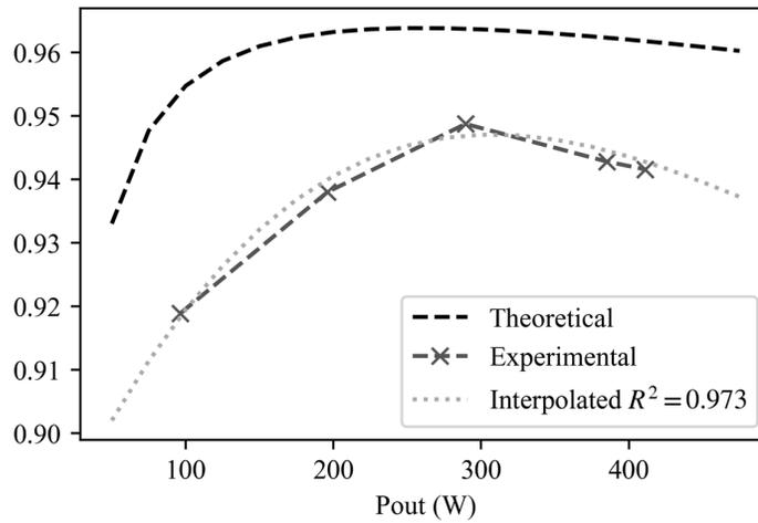
Fig. 53 SM obtained efficiency values vs theoretical curve.
