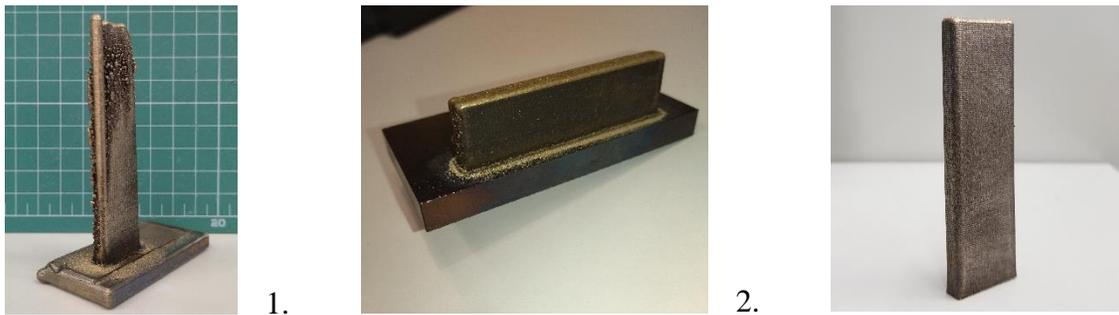
**Figure 42** – Parts fabricated: a) with ultrasonic assistance (built in a vertical direction) (left picture); b) with ultrasonic assistance (built in a horizontal direction) (middle picture); c) without ultrasonic assistance (built in a vertical direction) (right picture).
