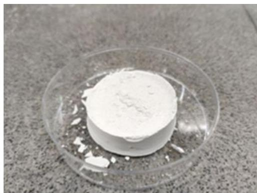
Figure 3. Typical BN/PVA aerogel prototype with the stoichiometric ratio of (2:1) (chapter 3).
