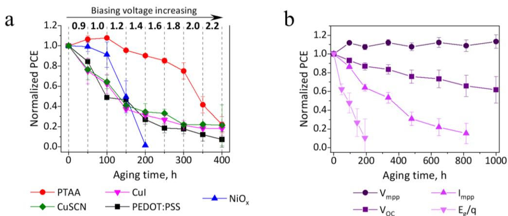
Figure 22. Evolution of normalized PCE during the “stepwise” biasing of solar cells with various HTLs (a). Evolution of the efficiency of PSCs with PTAA as HTL under applied electric bias ( $V_{mpp} = 0.7$  V,  $V_{OC} = 1$  V,  $I_{mpp} = 18.3$  mA/cm<sup>2</sup>,  $E_g/q = 1.55$  V) (b).
