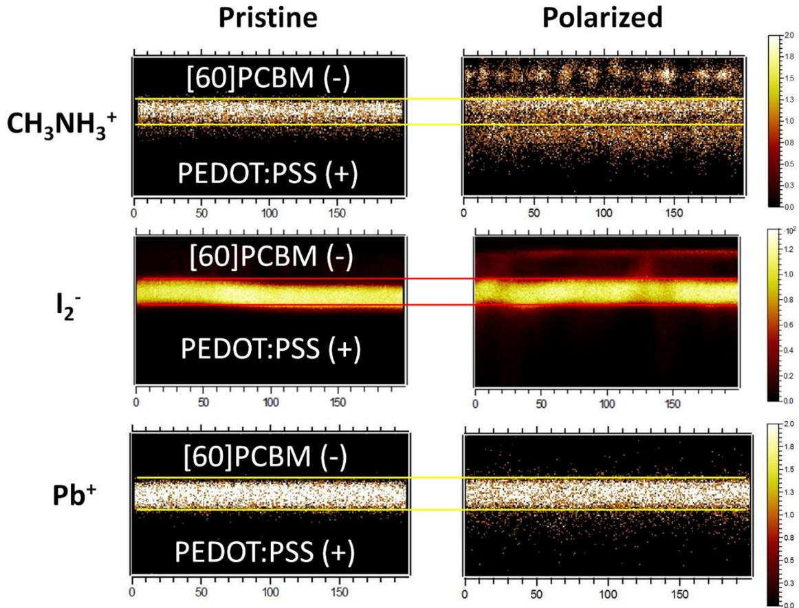
Figure 13. ToF-SIMS chemical maps showing the distribution of the characteristic marker ions  $\text{Pb}^+$ ,  $\text{I}_2^-$  and  $\text{CH}_3\text{NH}_3^+$  in the reference cells and devices exposed to 2 V under forward bias for 160 h.
