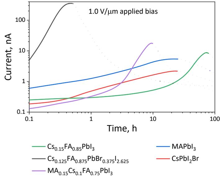
Figure 16. Evolution of the current flowing through the channel of the lateral two-terminal device under potentiostatic polarization with  $1 \text{ V}/\mu\text{m}$  applied bias for various perovskite materials.
