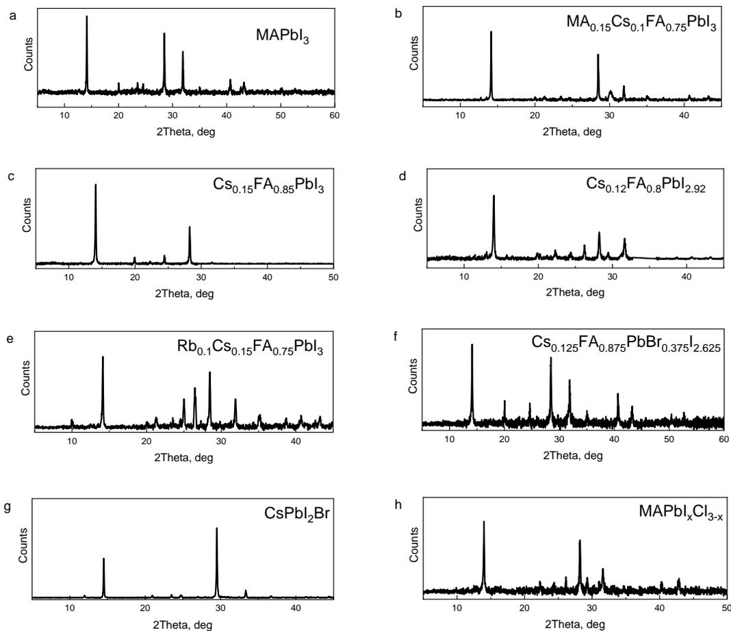
Figure A1. XRD data for freshly prepared optimized thin films of perovskite materials:
