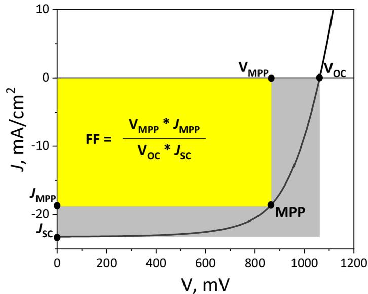
Figure 4. Example of  $J$ - $V$  curve with measured solar cell characteristics
