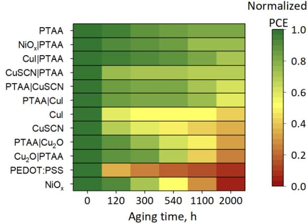
Figure 23. Evolution of normalized average efficiency for solar cells with various HTLs under constant 1V electric bias. HTLs are ranged from the best (top) to worst (bottom).
