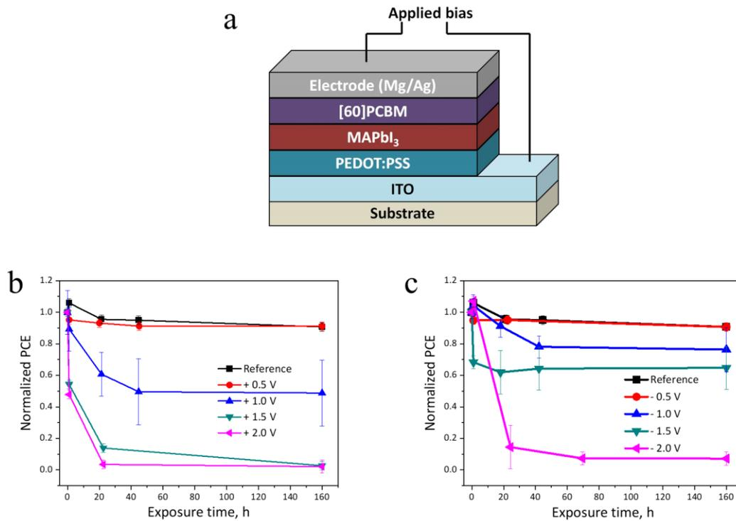
Figure 11. Schematic layout of the p-i-n perovskite solar cell architecture (a) The evolution of the device performance under different external biases applied in forward direction (b) and the comparison of the device degradation kinetics under forward and reverse bias of 1.5 V (c).
