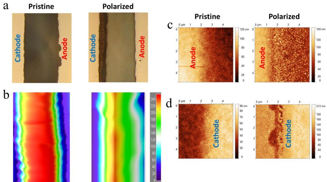
Figure 9. Optical microphotograph of the device channel before (left) and after (right) applying  $1 \text{ V}/\mu\text{m}$  bias for 340 h (a). PL mapping of the channel before (left) and after (right) applying  $1 \text{ V}/\mu\text{m}$  bias for 24 h (b). AFM for anode (c) and cathode (d) areas before (left) and after (right) applying  $1 \text{ V}/\mu\text{m}$  bias for 100 h.
