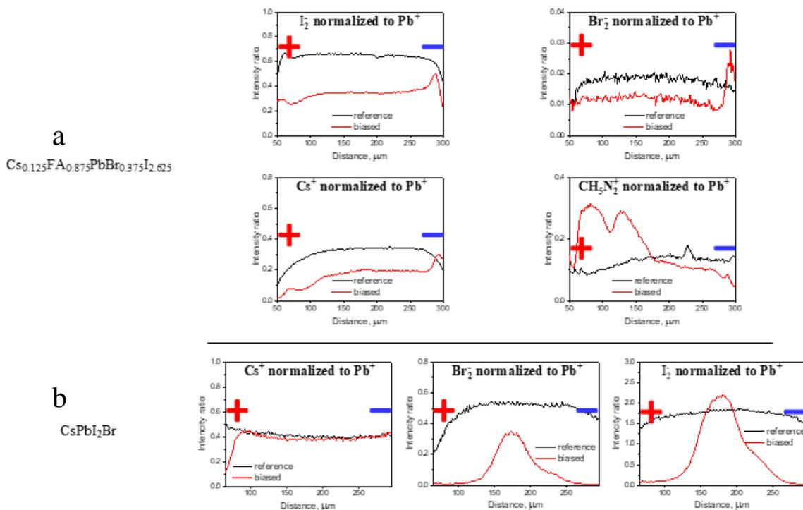
Figure 18-2. ToF-SIMS profiles of lateral two-terminal devices for across the channel formed by corresponding (noted on the left) perovskite semiconductor film  $\text{Cs}_{0.125}\text{FA}_{0.875}\text{PbBr}_{0.375}\text{I}_{2.625}$  (a)  $\text{CsPbI}_2\text{Br}$  (b) before (reference) and after (biased) exposure to electric bias of 1 V/ $\mu\text{m}$  for 300 h. A ratio of ion yields is given to account for possible geometry effects.
