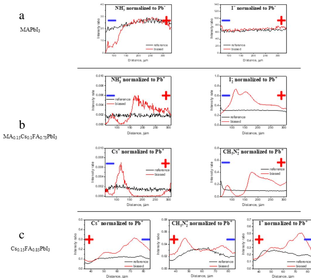
Figure 18-1. ToF-SIMS profiles of lateral two-terminal devices for across the channel formed by corresponding (noted on the left) perovskite semiconductor film MAPbI<sub>3</sub> (a) MA<sub>0.15</sub>Cs<sub>0.1</sub>FA<sub>0.75</sub>PbI<sub>3</sub> (b) Cs<sub>0.15</sub>FA<sub>0.85</sub>PbI<sub>3</sub> (c) before (reference) and after (biased) exposure to electric bias of 1 V/μm for 300 h. A ratio of ion yields is given to account for possible geometry effects.
