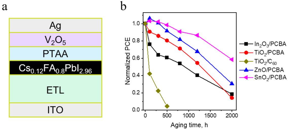
Figure 27. Schematic structure of solar cells used in the experiment of ETL variation (a).
