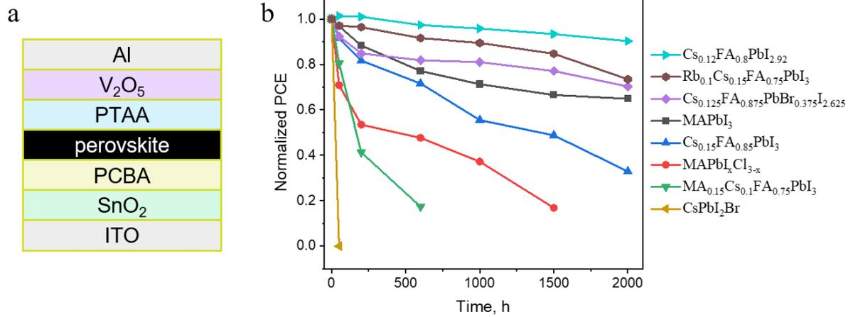
Figure 20. N-i-p solar cells device configuration (a). Normalized average PCE evolution for the batches of solar cells with different perovskite photoactive layers (b).
