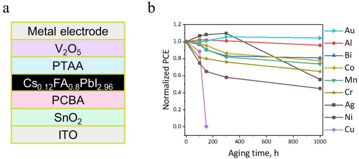
Figure 28. Schematic structure of solar cells used in the experiment of top electrode variation (a). Evolution of normalized average PCE of solar cells with various electrode materials (b).
