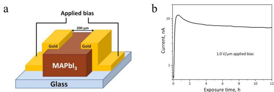
Figure 8. General layout of the lateral two-electrode device (a). Evolution of the current flowing through the channel of the lateral two-terminal device under potentiostatic polarization with  $1\ \text{V}/\mu\text{m}$  applied bias (b).
