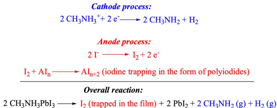
Figure 15. Schematic representation of the revealed mechanism of the field-induced electrochemical decomposition of MAPbI<sub>3</sub>.
