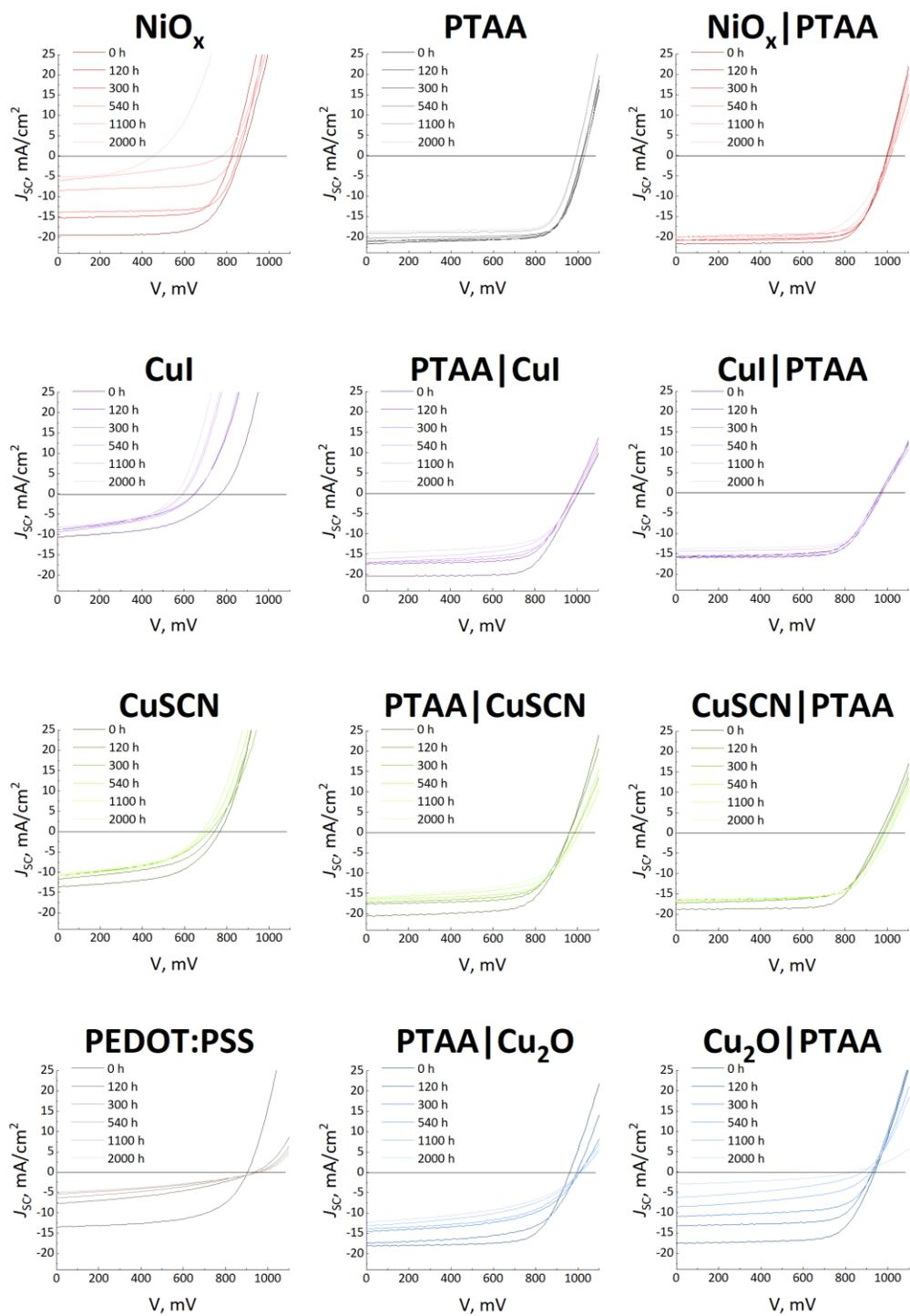
Figure A5. The typical examples of the device J-V curves evolution under 1 V external bias voltage applied in forward direction.
