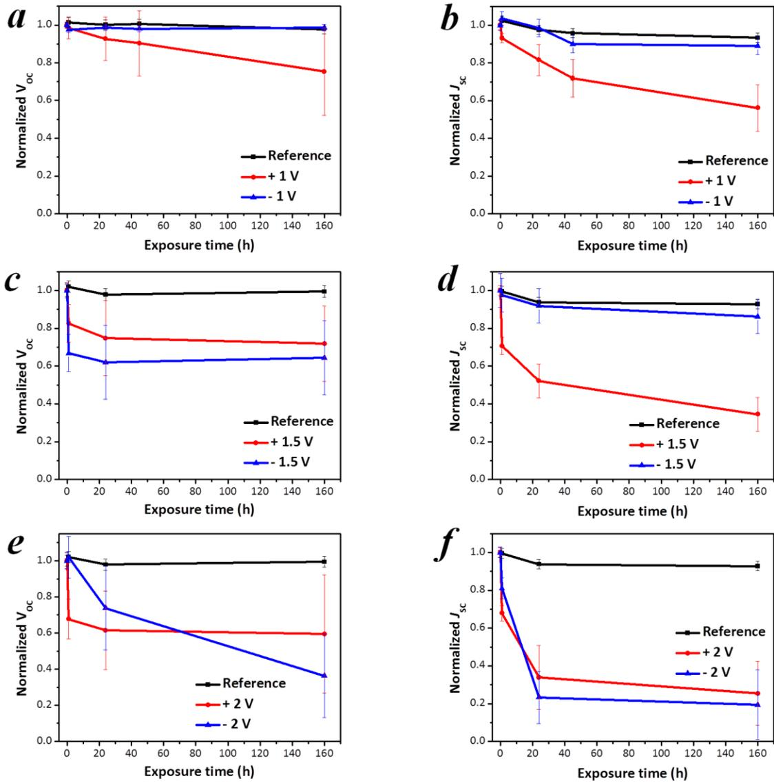
Figure A2. Evolution of the solar cell open circuit voltage ( $V_{oc}$ ; a, c, e) and short circuit current density ( $J_{sc}$ ; b, d, f) as functions of the electric bias exposure time at the applied potentials of 1 V (a-b), 1.5 V (c-d) and 2 V (e-f) in forward and reverse directions.
