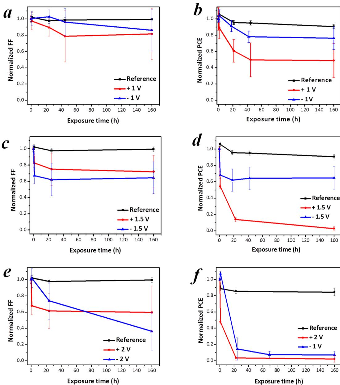
Figure A3. Evolution of the solar cell fill factor ( $V_{OC}$ ; a, c, e) and power conversion efficiency ( $PCE$ ; b, d, f) as functions of the electric bias exposure time at the applied potentials of 1 V (a-b), 1.5 V (c-d) and 2 V (e-f) in forward and reverse directions.
