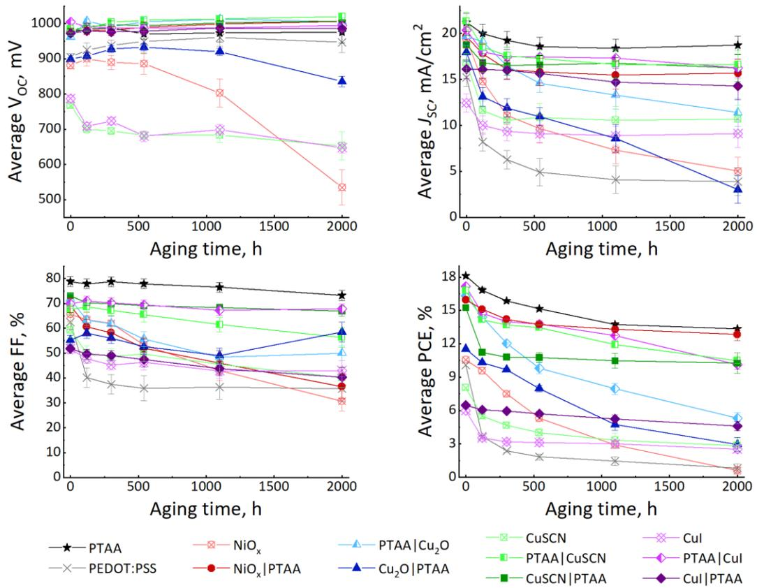
Figure A4. Evolution of the solar cell average open circuit voltage ( $V_{oc}$ ), short circuit current density ( $J_{sc}$ ) fill factor (FF) and power conversion efficiency (PCE) as functions of the electric bias exposure time at the applied potential of 1 V in forward direction.
