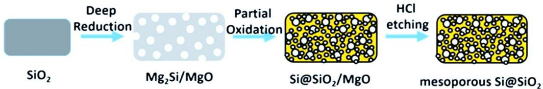
Figure 4 Schematic representation of the unconventional MRR (Deep reduction and Partial oxidation) [81]
