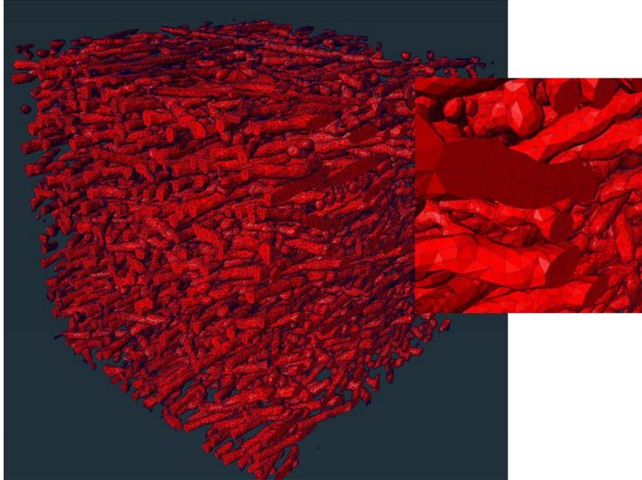
Figure 44 – FE model of fibres created using Avizo software
