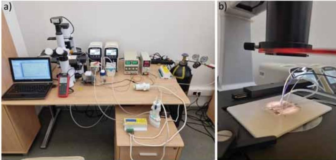
Figure 45. a) Photograph of the whole experiment setup, b) Photograph of microfluidic cell.
