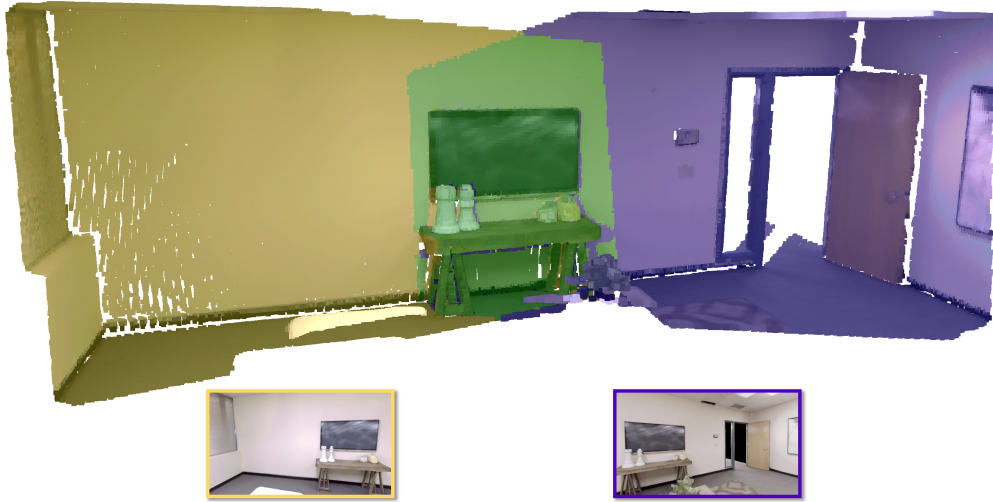
Figure 4-3: Visual explanation of 3D Intersection over Union (IoU) metric used for camera frames proximity estimation. Computed with voxels of the scene, this metric naturally describes both proximity of the camera poses and the visual similarity of their image frames. Here for the visualized frames the 3D IoU is equal to 0.15.
